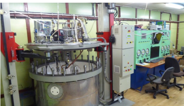
Figure 2. Stand of combined simulators: respiratory, metabolic and hyperbaric.
