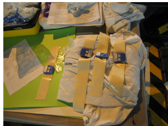
Figure no. 1: Personal Alarm Dosimeter (Blog: Histoires d'un scaphandrier or the Stories of a Commercial Diver, 2015)
