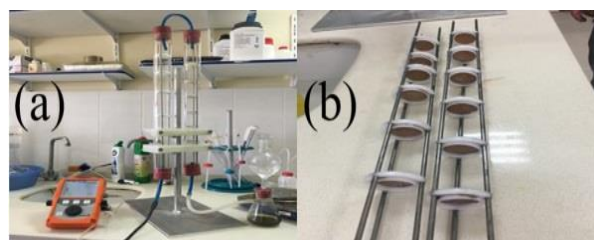
Figure 10(a). Experiment start; (b) Image of the membranes at the end of the experiment
