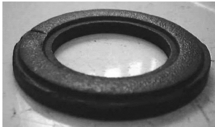
Figure 5 Valve ring subject to heavy wear due to the deposition of coke particles at the valve seats [42]
