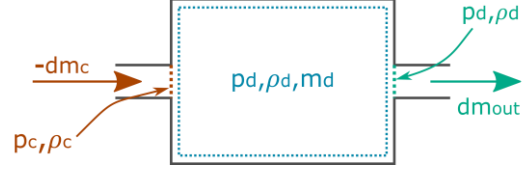
Figure 26 Discharge plenum chamber
