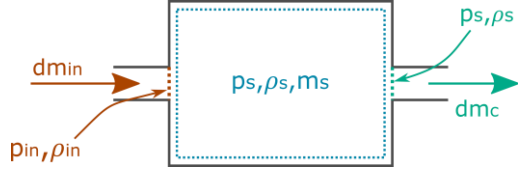
Figure 25 Suction plenum chamber
