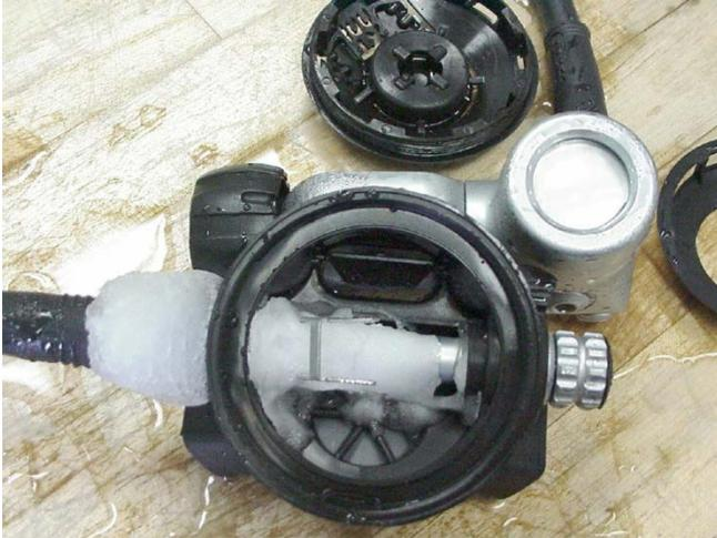
**Figure 11-1 Ice accumulation in a 2<sup>nd</sup> stage regulator after free flow.**
