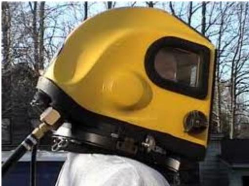
UBAs in this category also supply gas to the diver via an umbilical hose; however, the gas constantly flows past the diver's face (no demand required) into the helmet or mask. Excess gas is constantly dumped from the helmet or mask into the water. No oral-nasal mask or mouthpiece is used.
