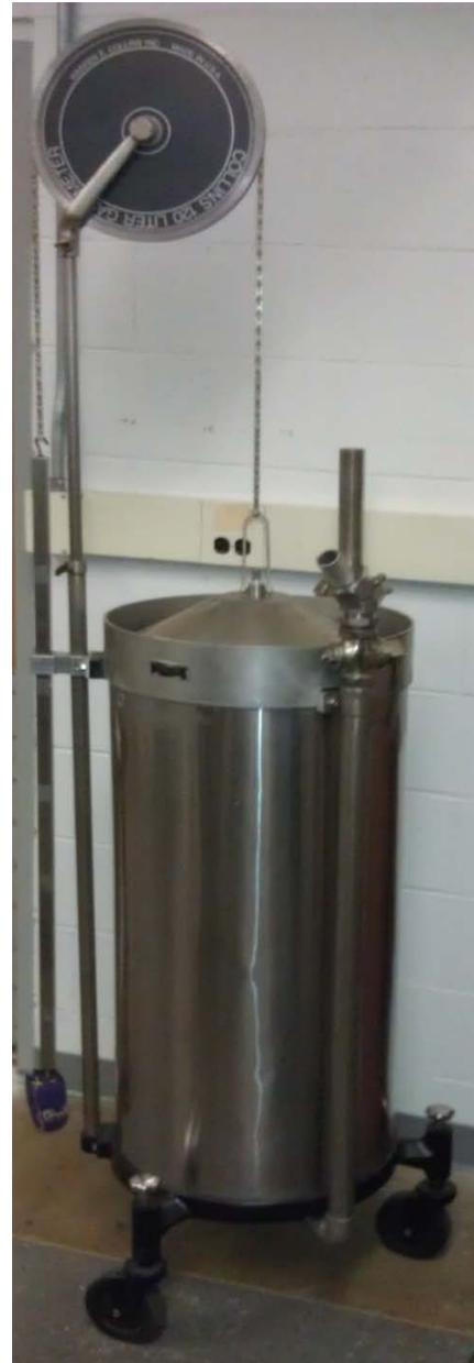
**Figure 5-5 Tissot Gasometer,
