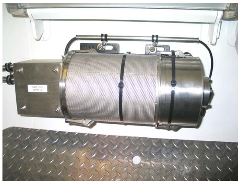
Figure 3-21. Carbon Dioxide (CO 2 ) Scrubber Assembly
