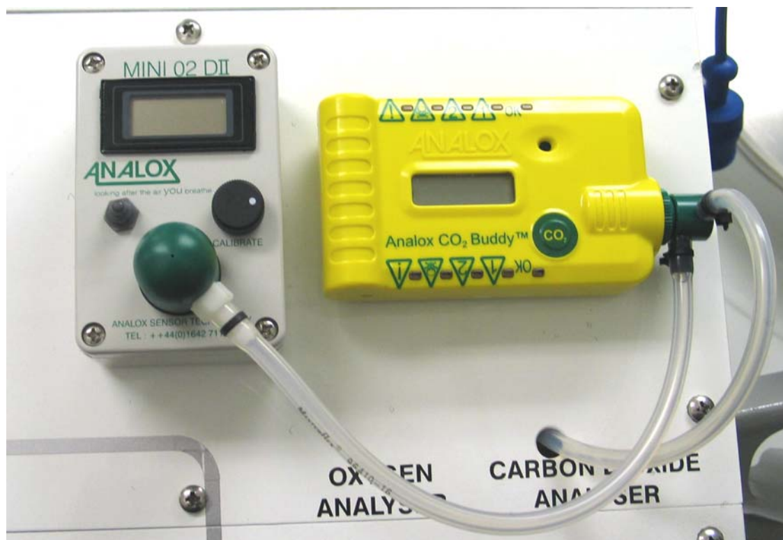
Figure 3-18. Oxygen (O 2 ) Analyzer (left) and Carbon Dioxide (CO 2 ) Analyzer
