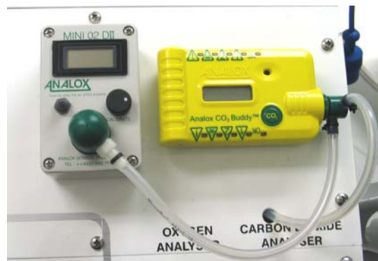
Figure 2-12. Air Sample Monitors
