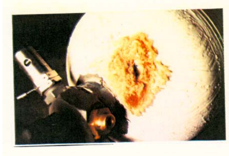
LEVEL 3 STRUCTURAL DAMAGE (CONDEMNED)
