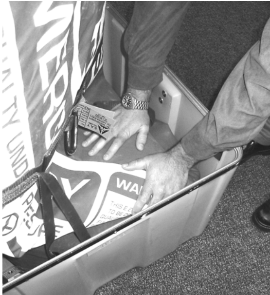
Figure 4-2. Folding The Flexible Tube – Second Fold
