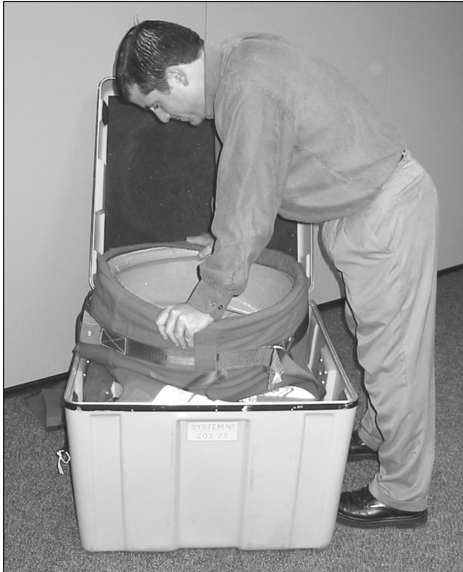
Figure 4-4. Folding The Flexible Tube – Fourth Fold
