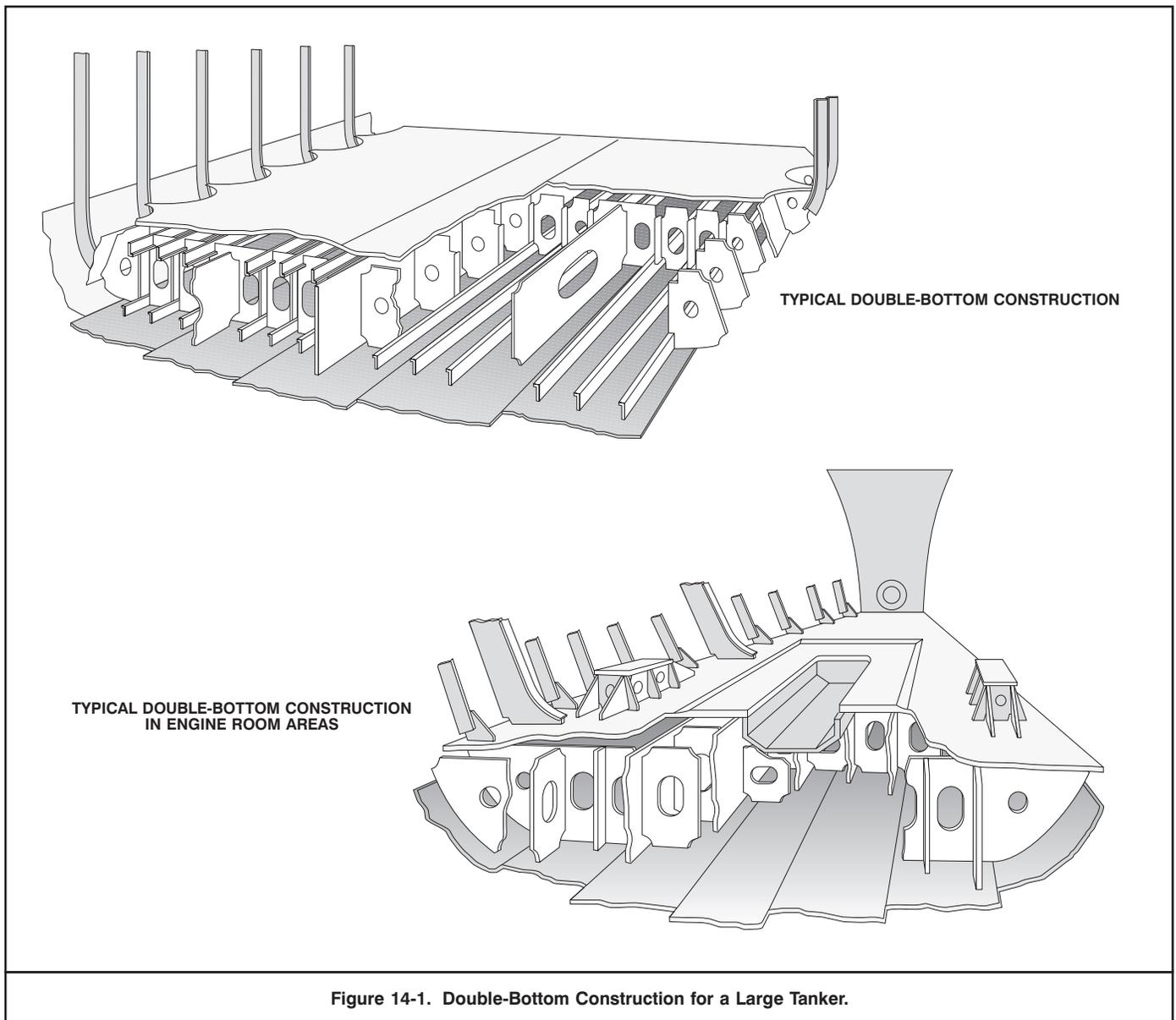
Figure 14-1. Double-Bottom Construction for a Large Tanker.
