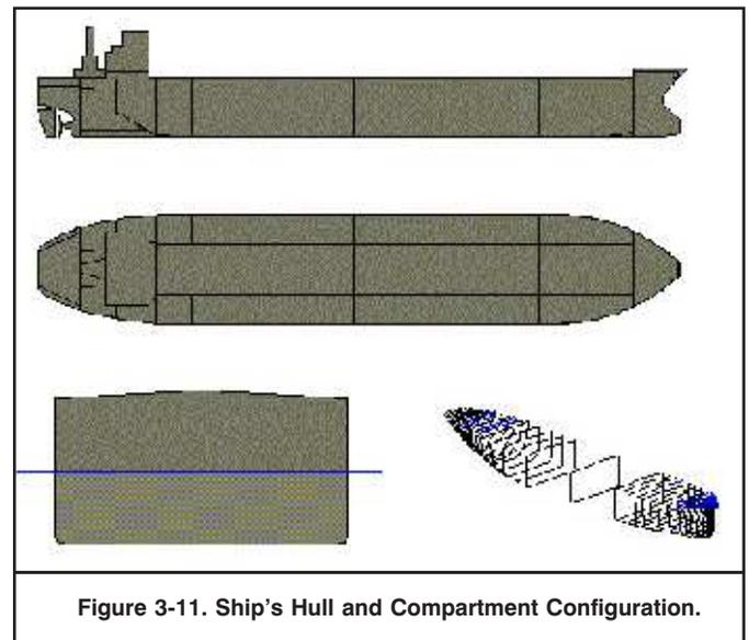
**Figure 3-11. Ship's Hull and Compartment Configuration.**
