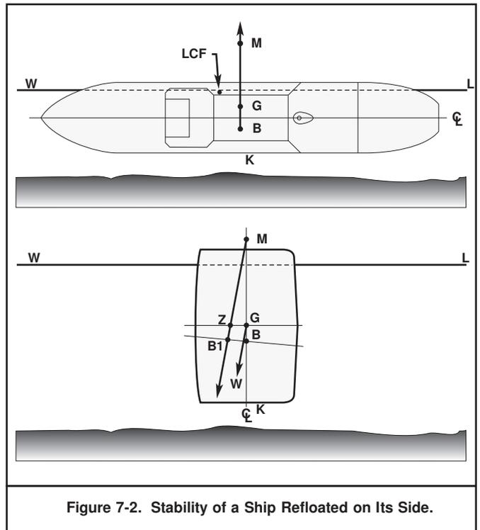
Figure 7-2. Stability of a Ship Refloated on Its Side.
