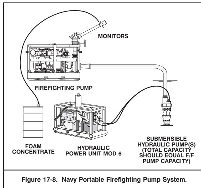
Figure 17-8. Navy Portable Firefighting Pump System.
