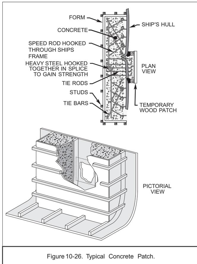
Figure 10-26. Typical Concrete Patch.
