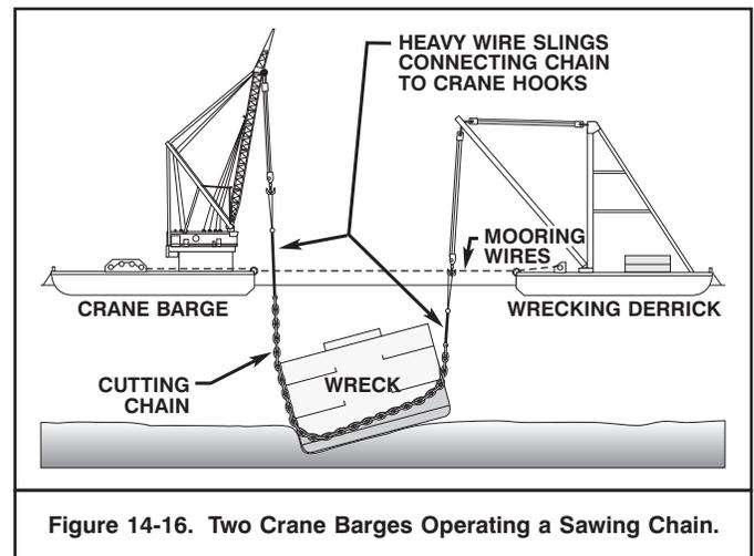
Figure 14-16. Two Crane Barges Operating a Sawing Chain.
