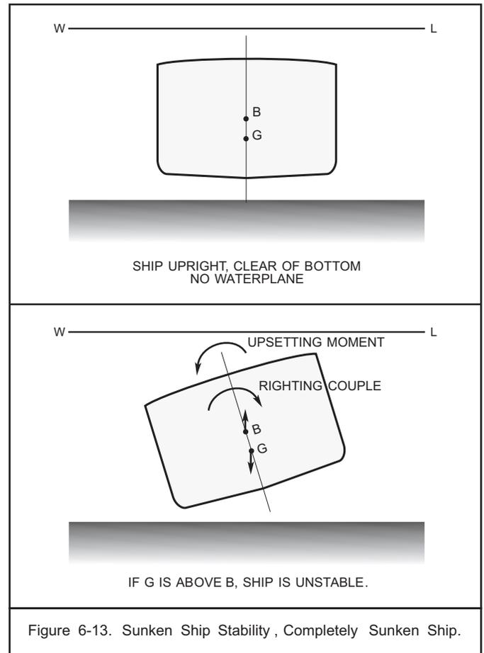
Figure 6-13. Sunken Ship Stability, Completely Sunken Ship.
