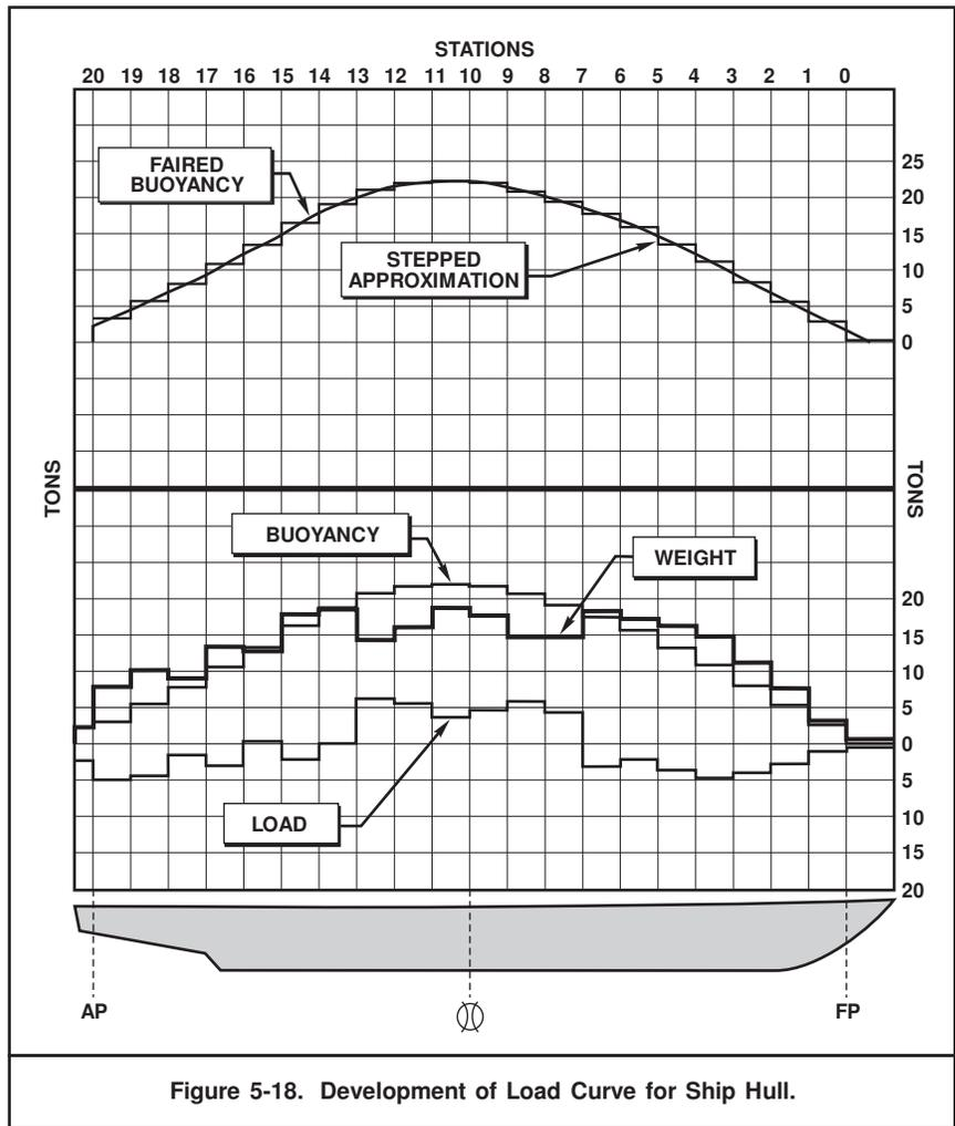
Figure 5-18. Development of Load Curve for Ship Hull.
