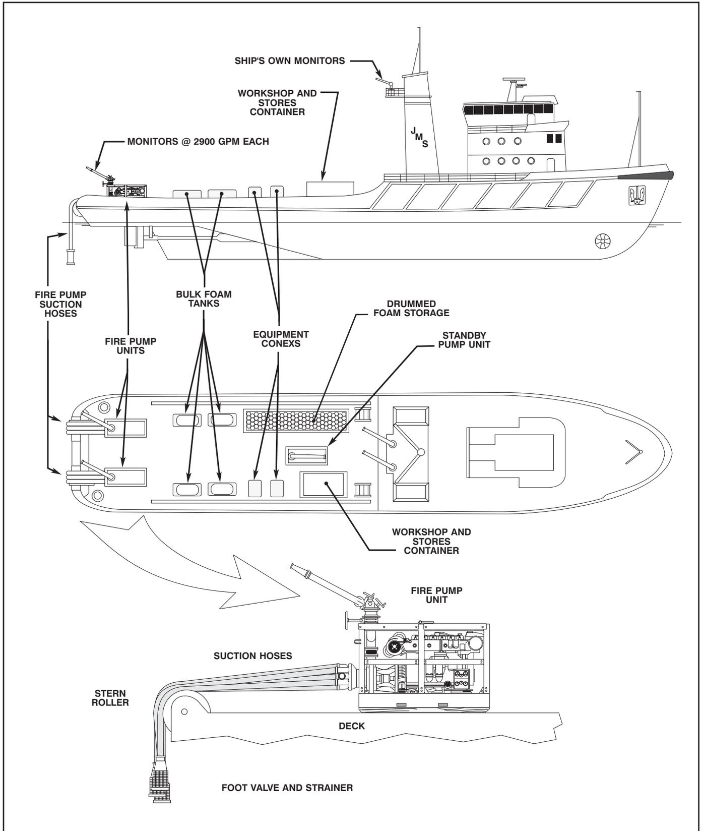
Figure 19-11. Common Arrangement of Portable Fire Pump Units on Chartered Oilfield Tug/Supply Ship.
