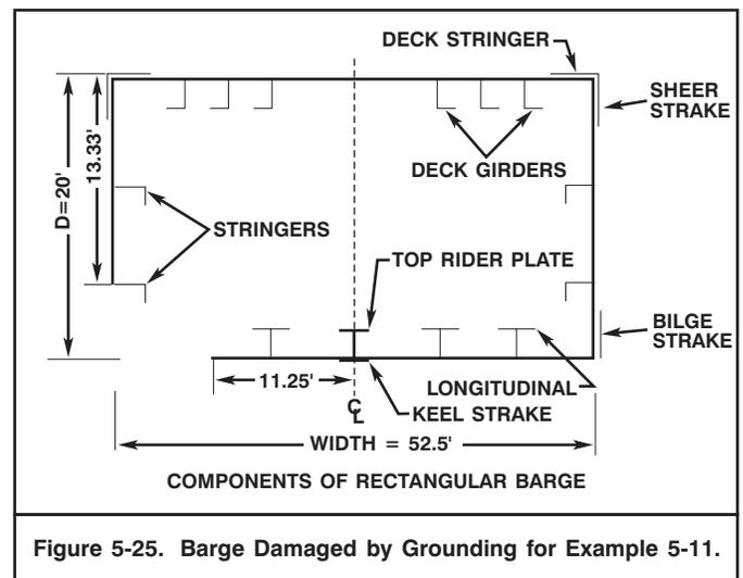
Figure 5-25. Barge Damaged by Grounding for Example 5-11.
