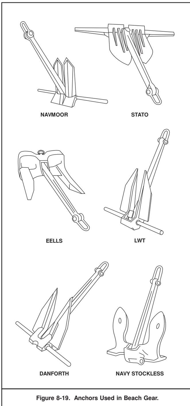
Figure 8-19. Anchors Used in Beach Gear.
