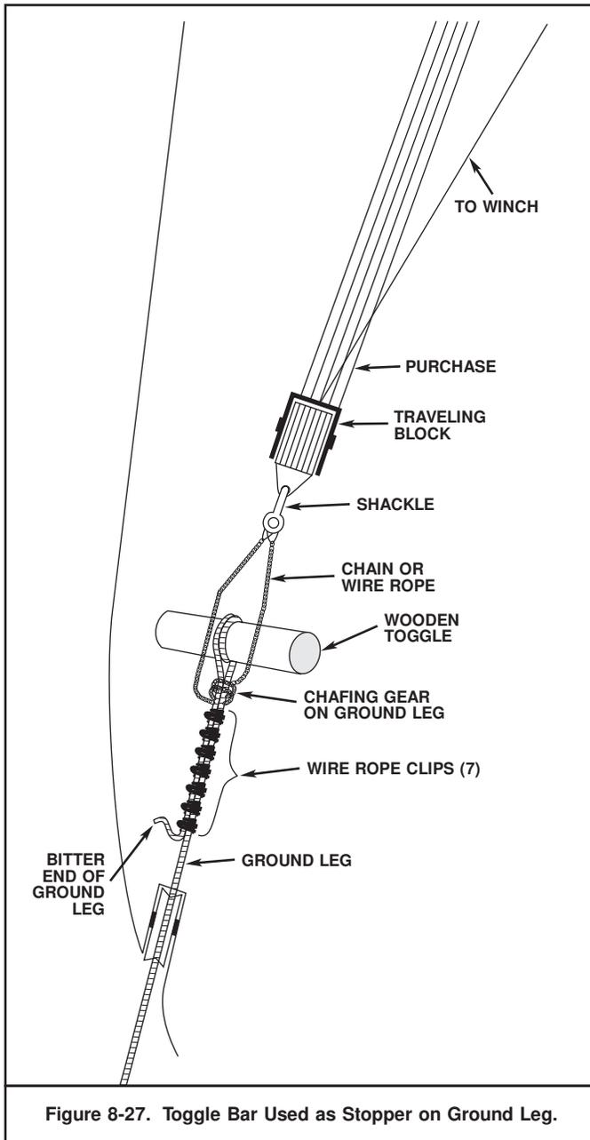
Figure 8-27. Toggle Bar Used as Stopper on Ground Leg.
