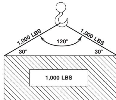
Figure E-1. Tension on Legs of Slings with Angular Loading.
