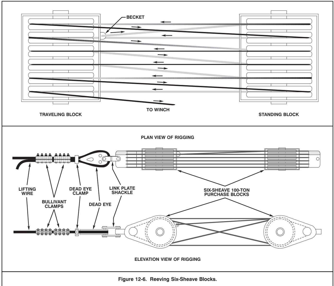
Figure 12-6. Reeving Six-Sheave Blocks.
