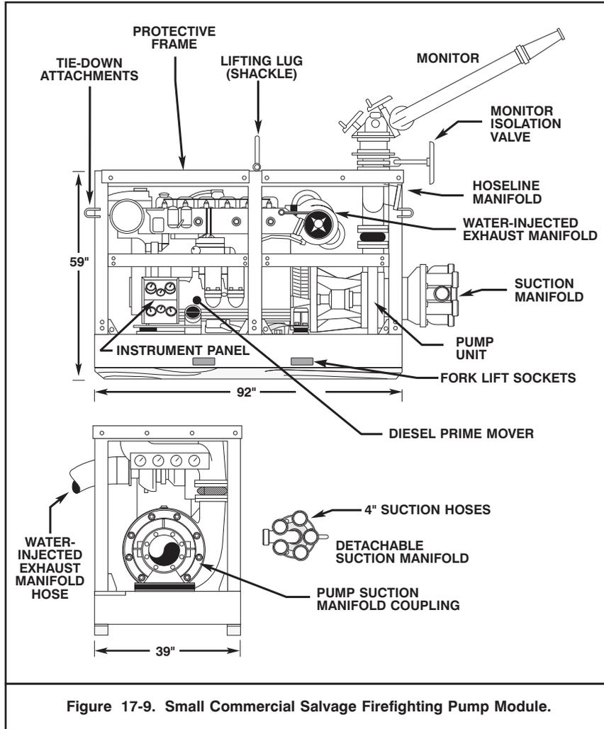
**Figure 17-9. Small Commercial Salvage Firefighting Pump Module.**
