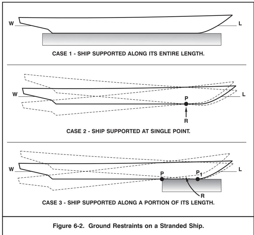
Figure 6-2. Ground Restraints on a Stranded Ship.
