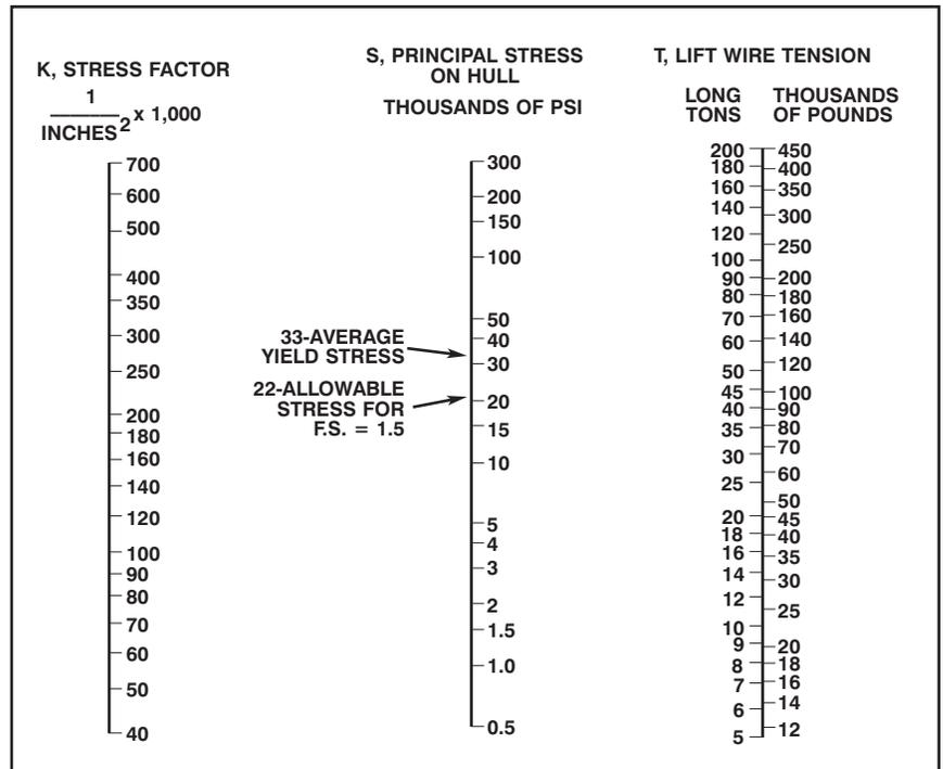
**Figure 12-17. Hull Stress Nomogram.**
