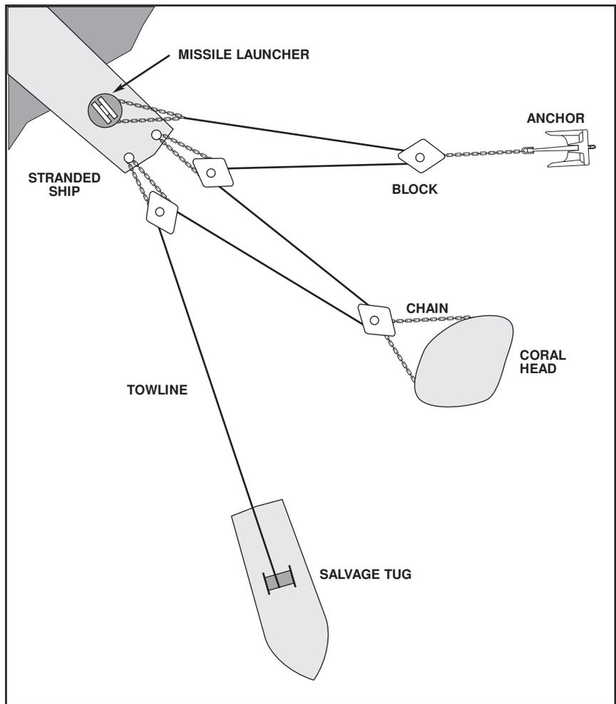
Figure 8-6. Dynamic Purchase Rigged Between Stranded Ship and Tug.
