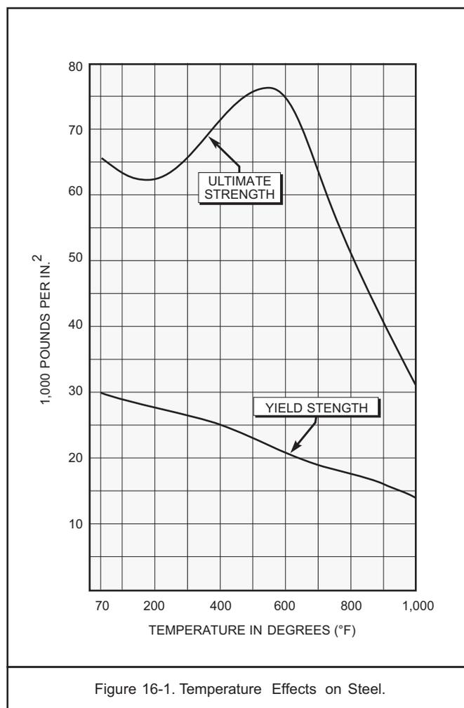
Figure 16-1. Temperature Effects on Steel.
