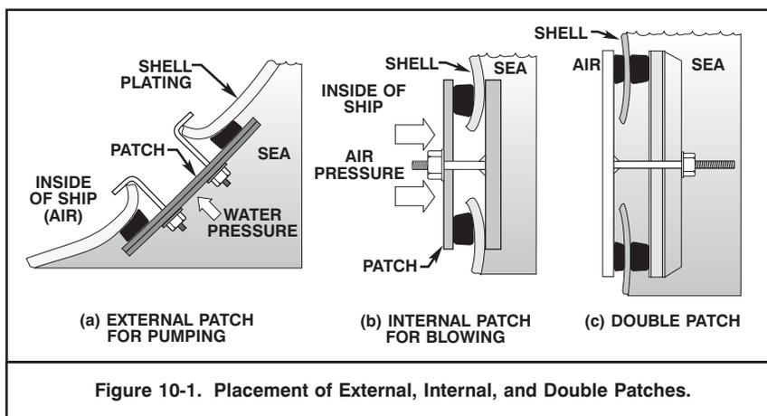
Figure 10-1. Placement of External, Internal, and Double Patches.
