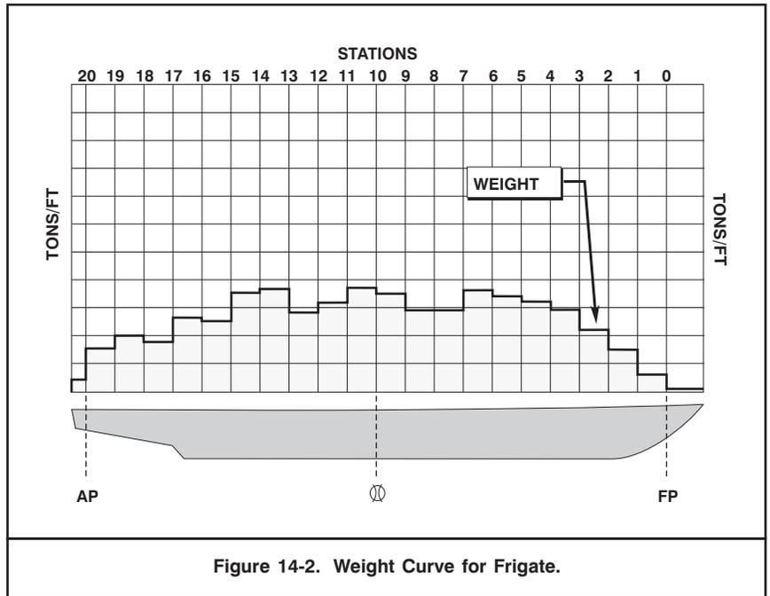
Figure 14-2. Weight Curve for Frigate.
