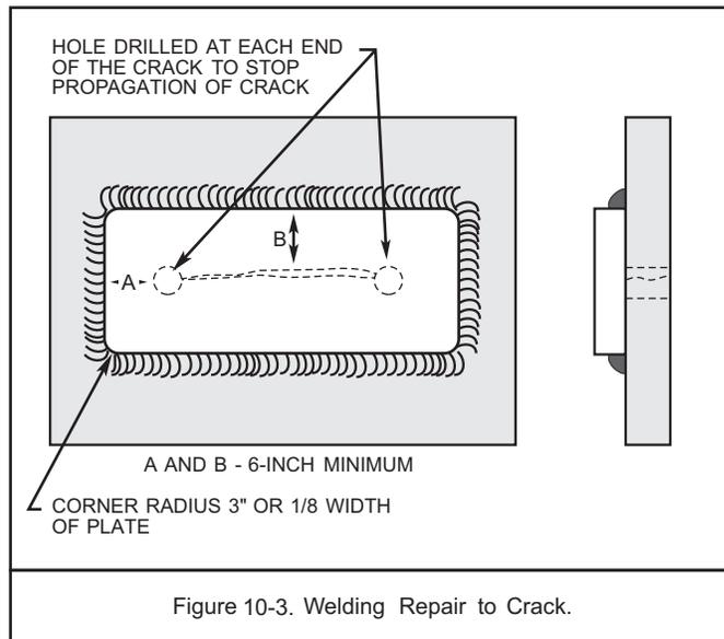
Figure 10-3. Welding Repair to Crack.
