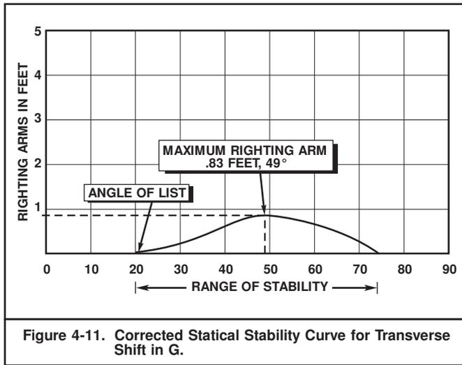
Figure 4-11. Corrected Statical Stability Curve for Transverse Shift in G.
