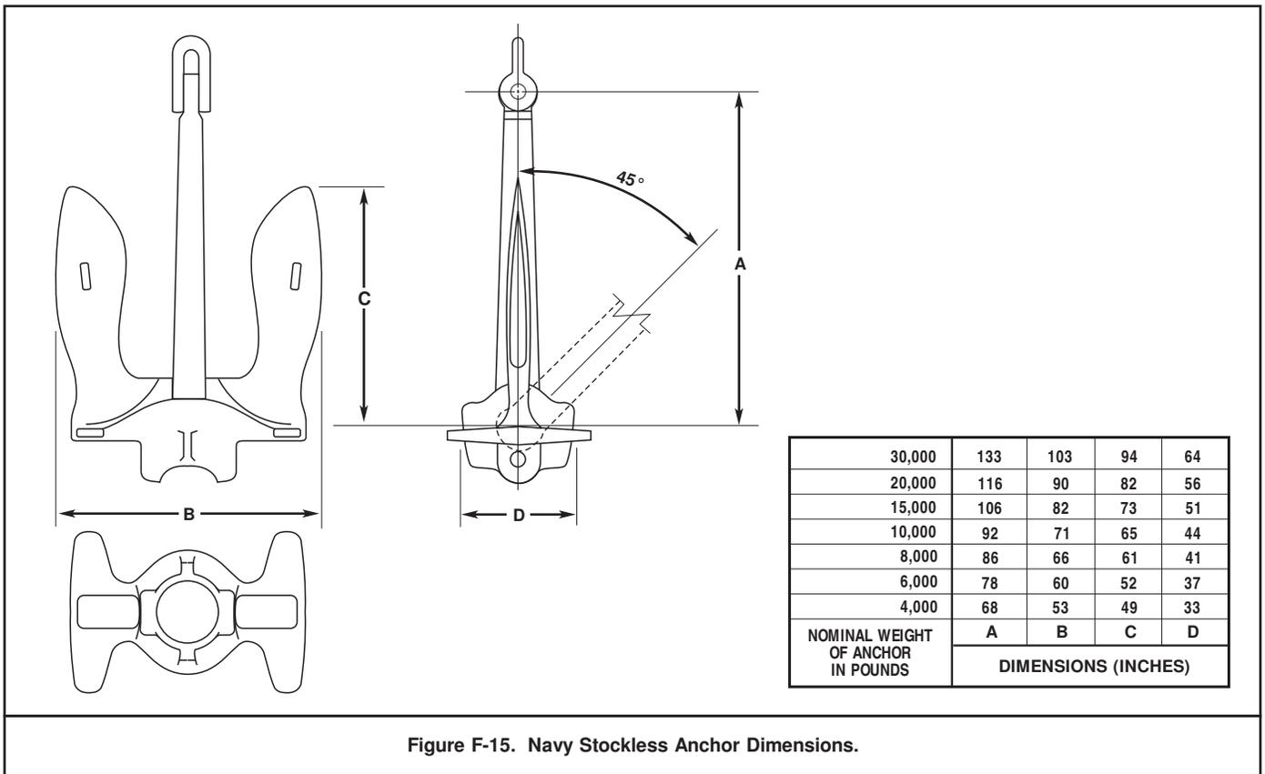
Figure F-15. Navy Stockless Anchor Dimensions.
