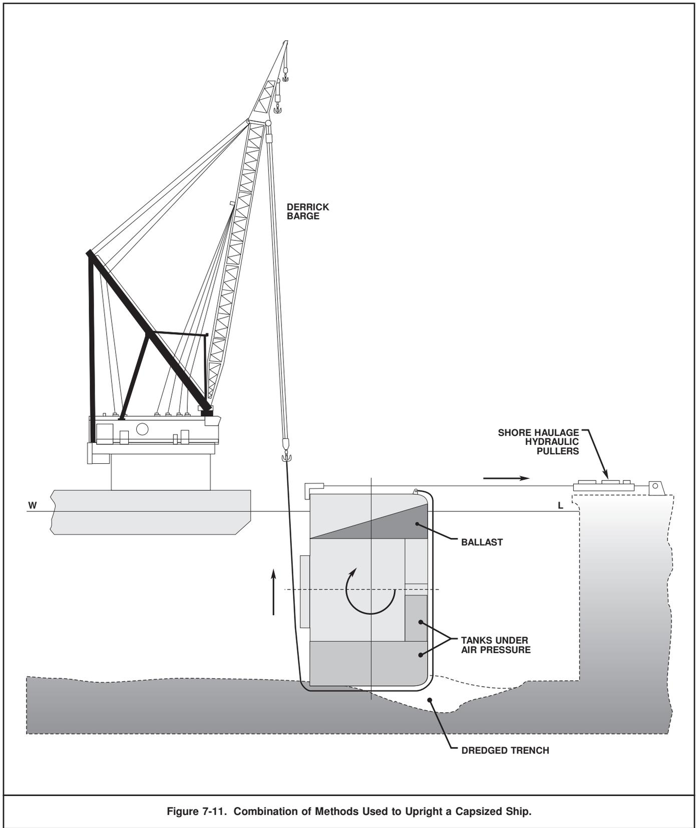
Figure 7-11. Combination of Methods Used to Upright a Capsized Ship.
