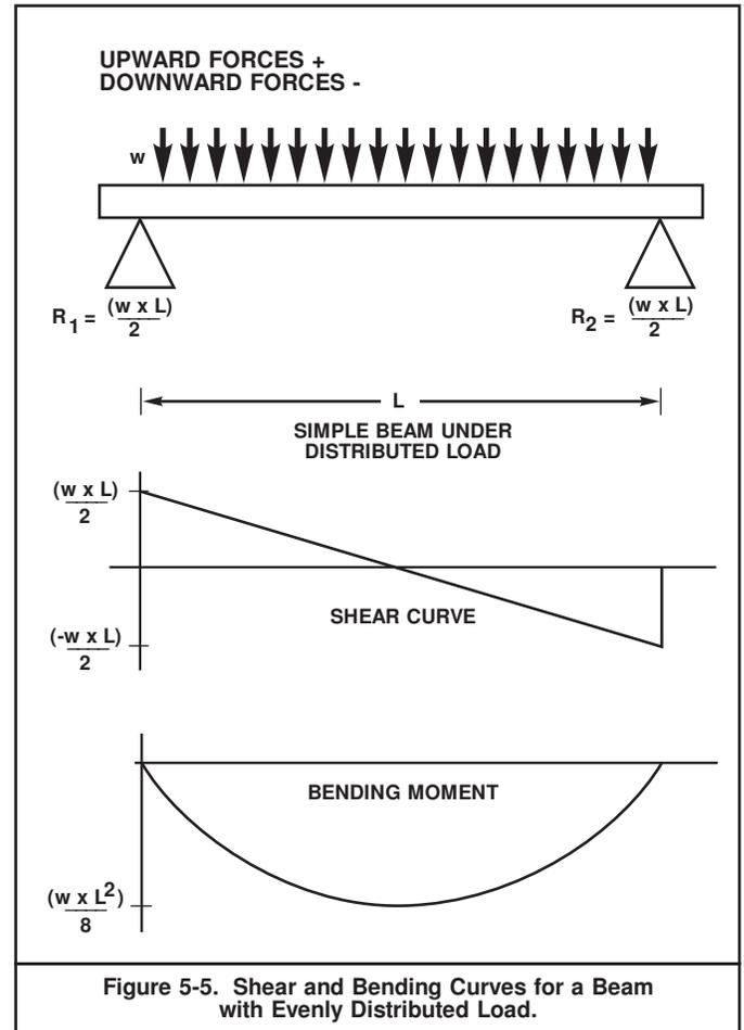
If the weight is evenly distributed along the length of the beam, the shear curve will pass through zero at the center of the beam and the bending moment curve will be a parabola with its maximum at center of the beam.
