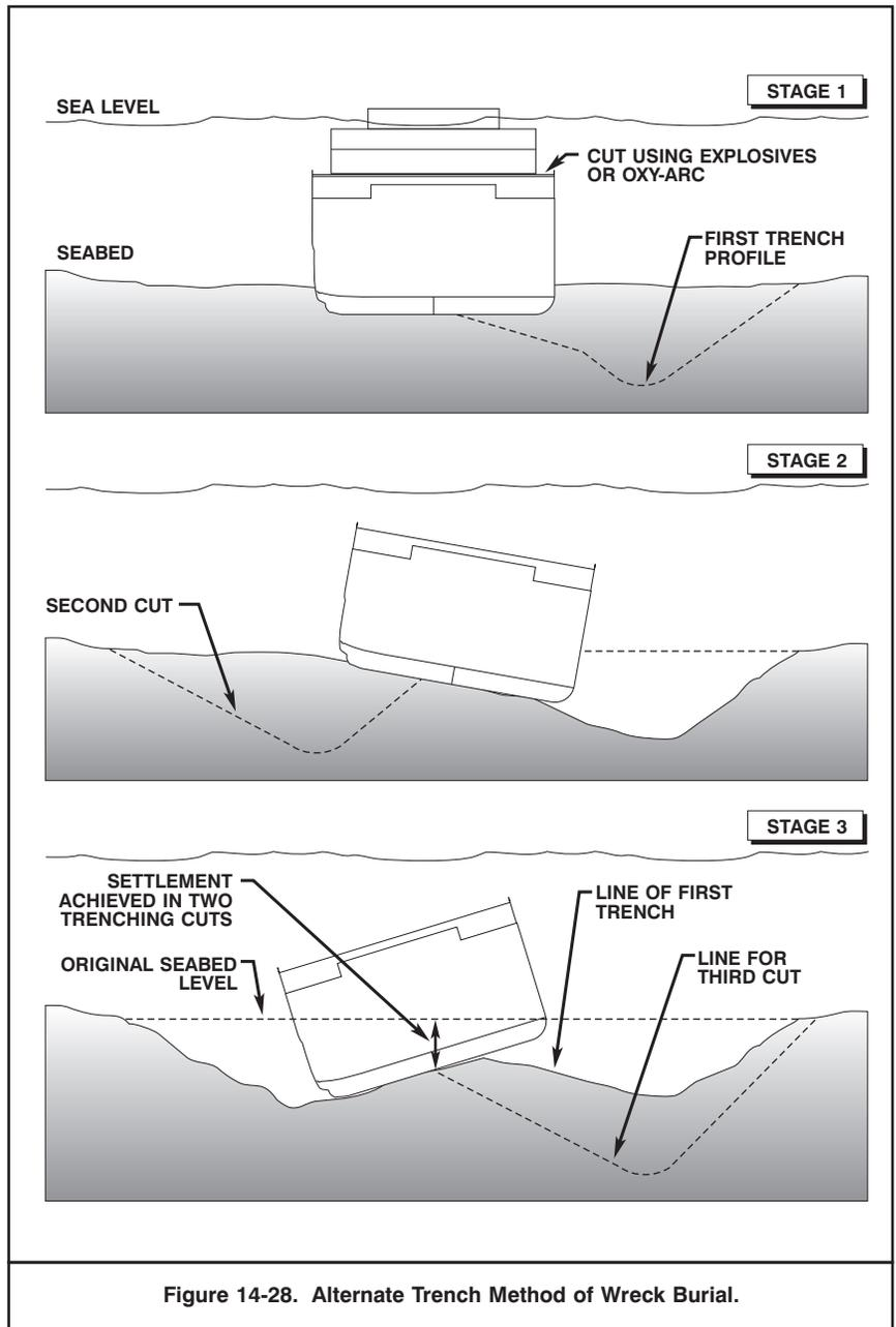
Figure 14-28. Alternate Trench Method of Wreck Burial.
