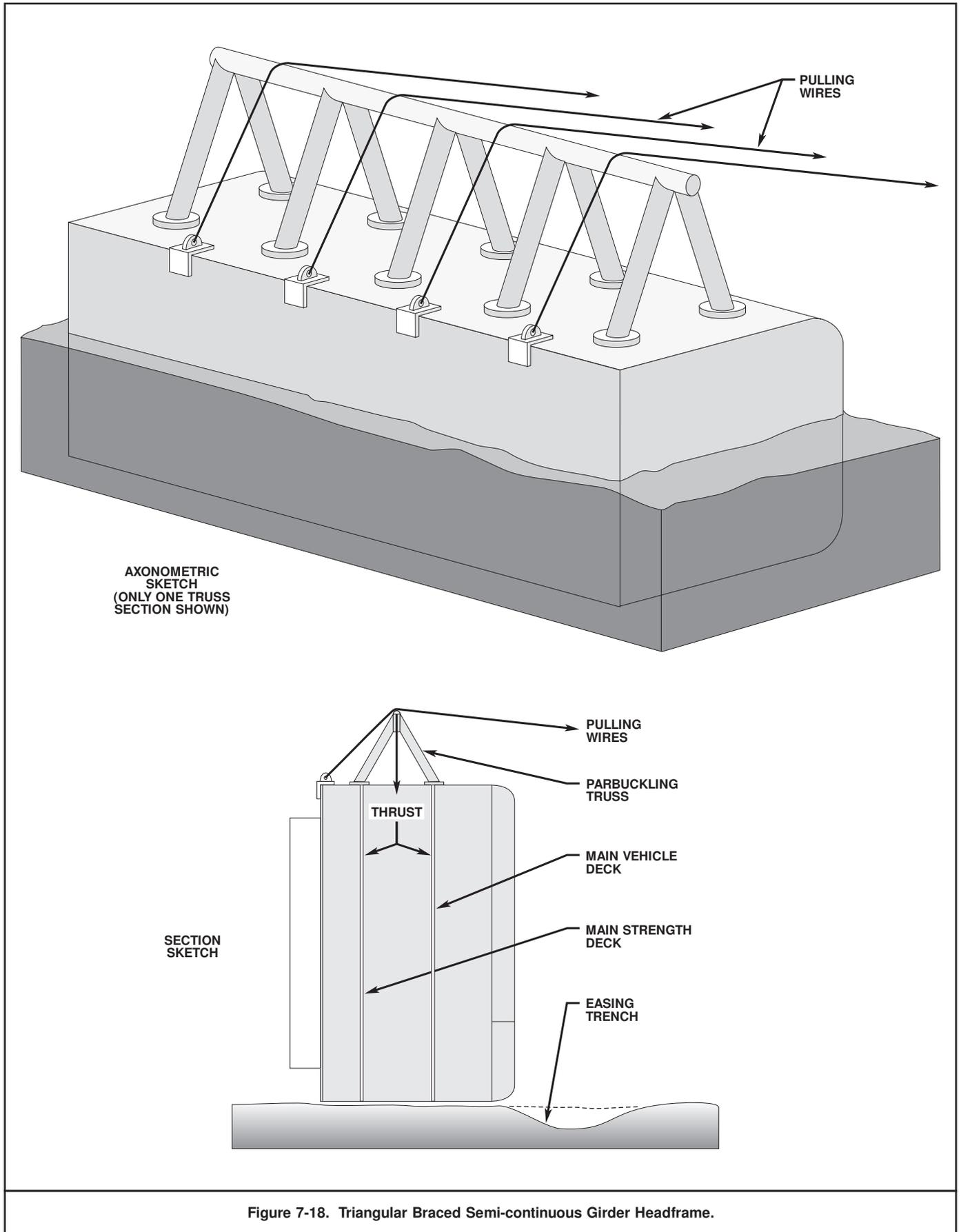
Figure 7-18. Triangular Braced Semi-continuous Girder Headframe.
