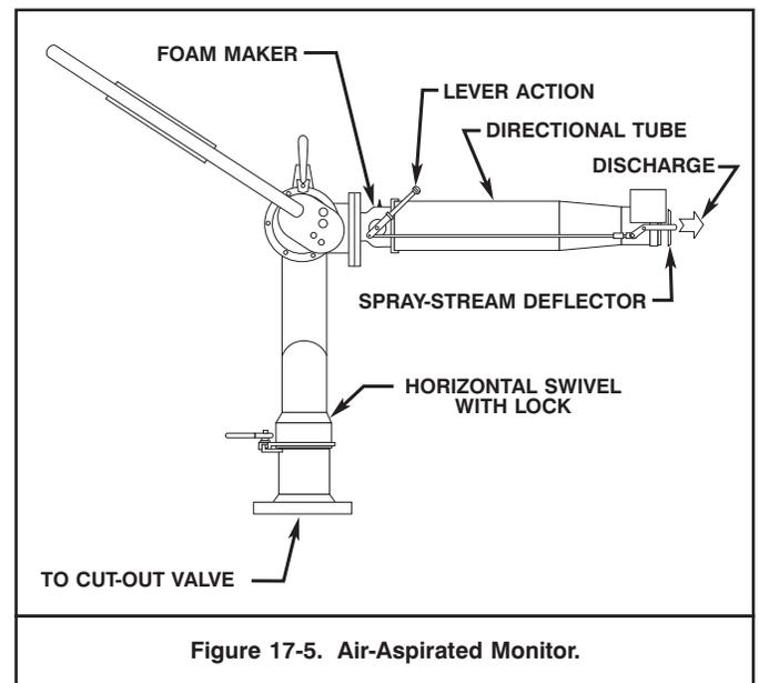
Figure 17-5. Air-Aspirated Monitor.
