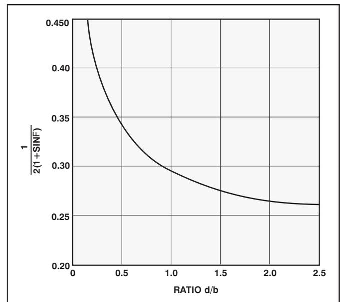
Figure 12-16. Wire Tension Factor.
