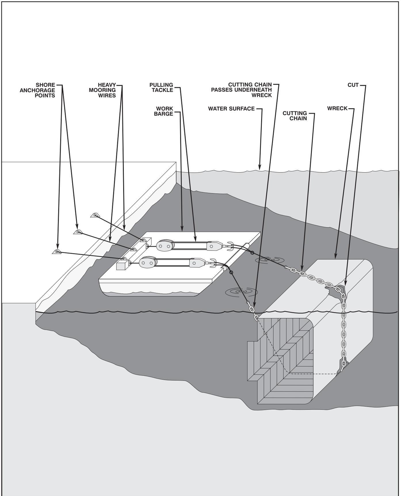
Figure 14-18. Horizontal Chain Cutting System.
