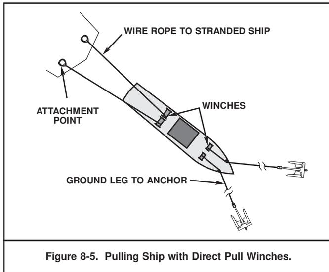
Figure 8-5. Pulling Ship with Direct Pull Winches.
