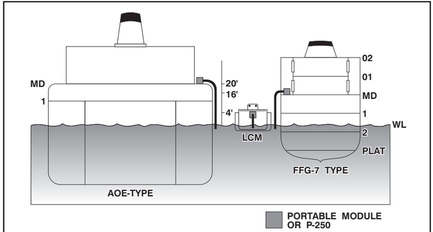
Figure 20-1. Relationship of Work Boat to Casualty Vessels and Staging of Portable Pumps.
