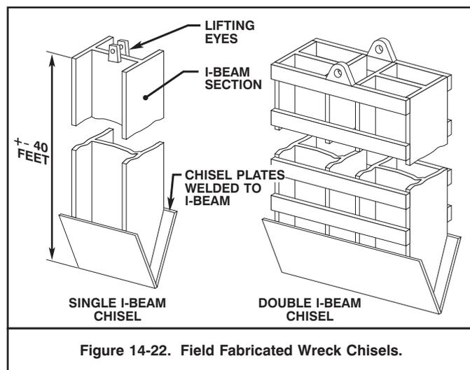
Figure 14-22. Field Fabricated Wreck Chisels.
