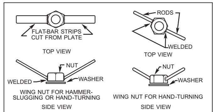
Figure 10-34. Wing Nuts for Salvage Patches.
