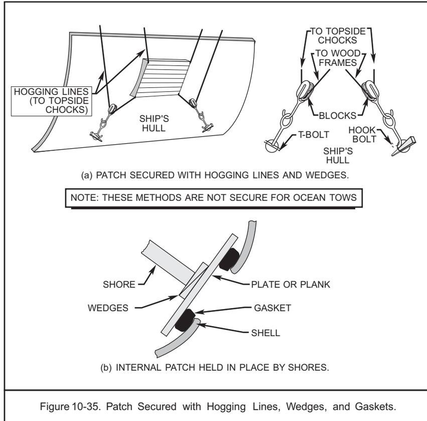
Figure 10-35. Patch Secured with Hogging Lines, Wedges, and Gaskets.
