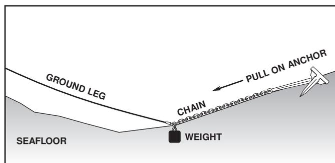
Figure 8-9. Ground Leg Configuration, Anchor on Up-Slope.
