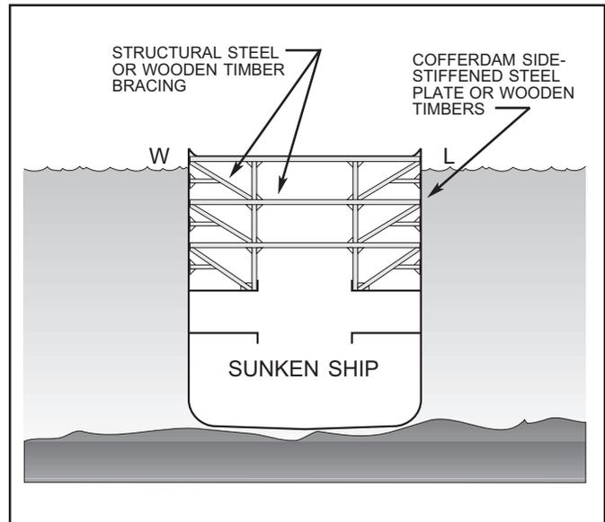
Figure 10-37. Complete Cofferdam Bracing.
