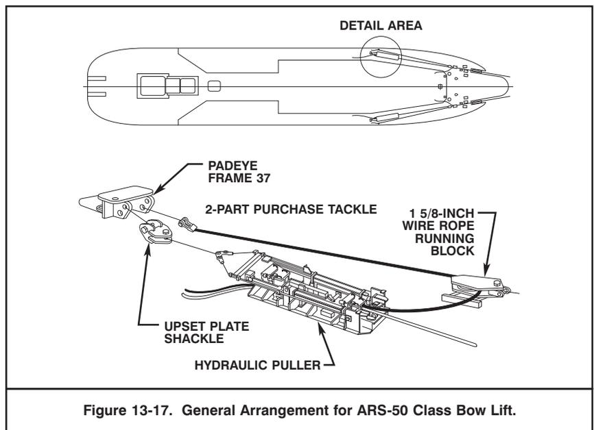
Figure 13-17. General Arrangement for ARS-50 Class Bow Lift.
