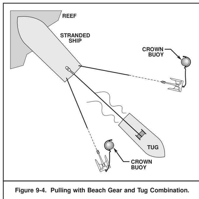
Figure 9-4. Pulling with Beach Gear and Tug Combination.
