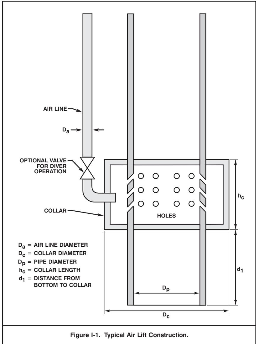
To ensure a steady flow, the compressor capacity should be twice the calculated air requirement. Pressure can be any over-bottom pressure.
