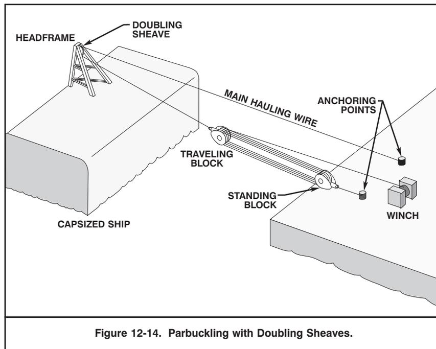
Figure 12-14. Parbuckling with Doubling Sheaves.
