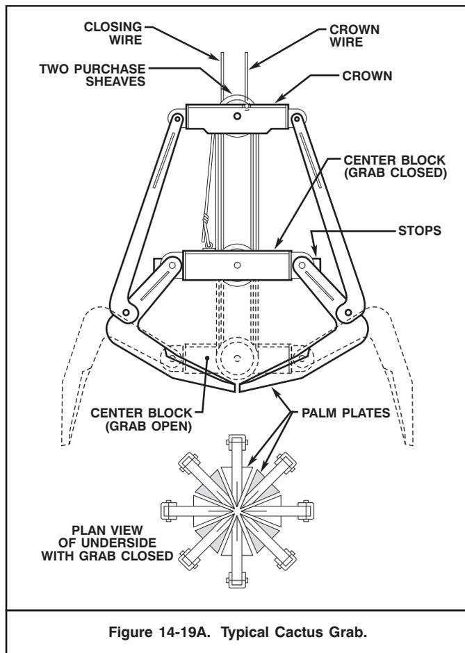
A typical cactus grab is shown in Figure 14-19A. This type of grab is useful on small wrecking-in-place projects and as an all-purpose rehandling grab on large wrecking projects. Orange peel grabs may have a different arrangement of grab leaves and tine points depending upon their design and origin.
