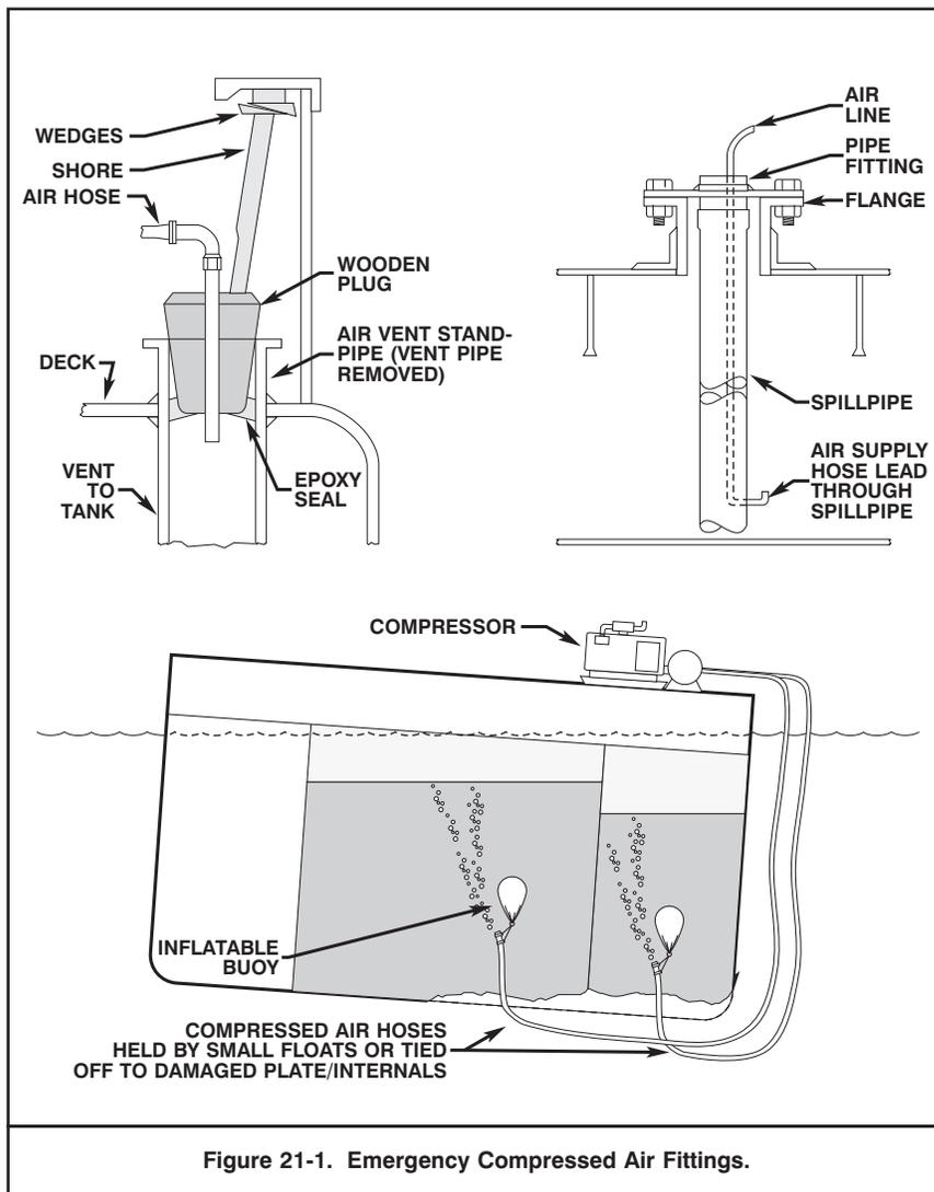
Figure 21-1. Emergency Compressed Air Fittings.
