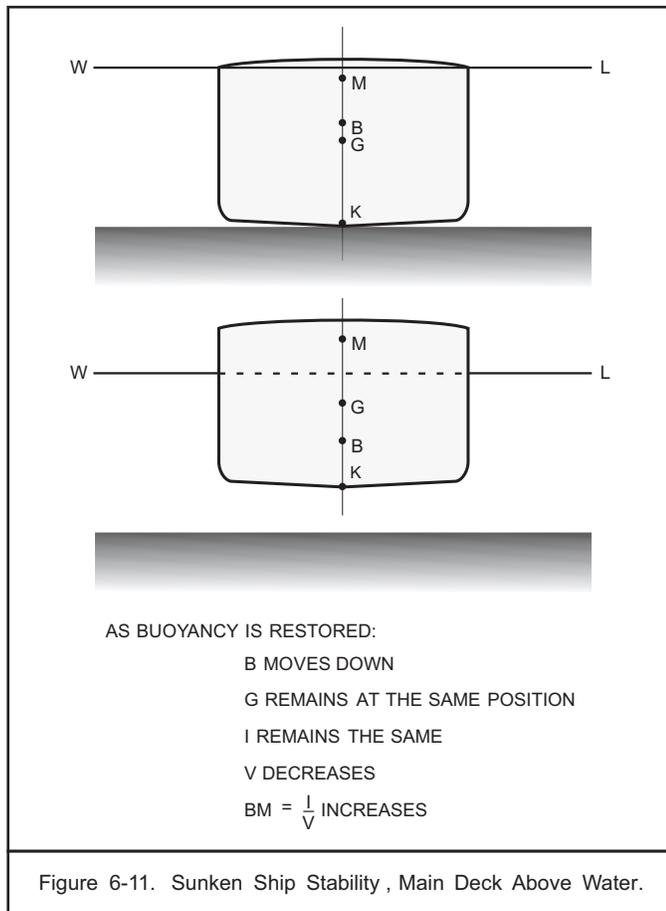
Figure 6-11. Sunken Ship Stability , Main Deck Above Water.
