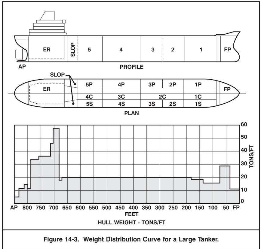
Figure 14-3. Weight Distribution Curve for a Large Tanker.
