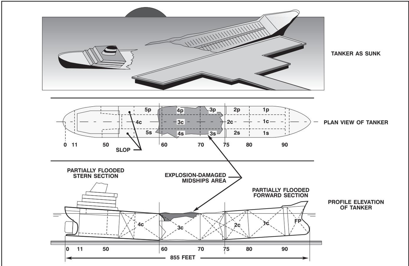
Figure 14-4. Tanker Wreck as Surveyed.
