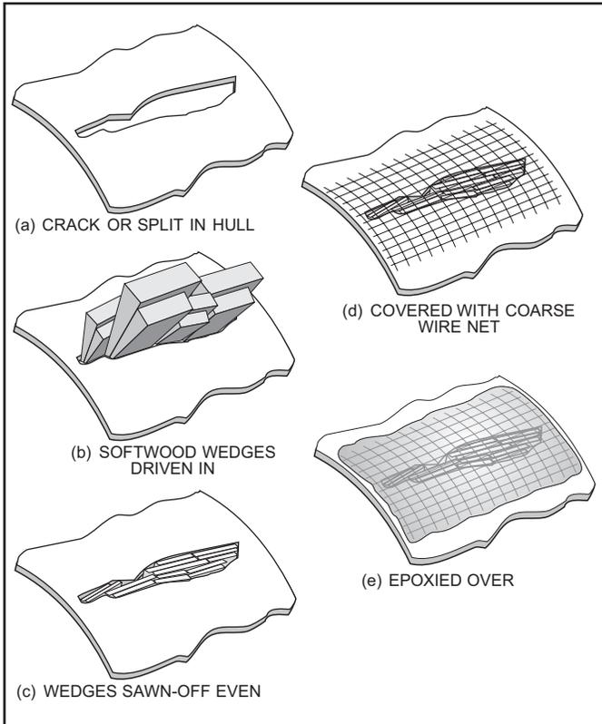
Figure 10-16. Sealing a Crack with Plugs and Wedges.
