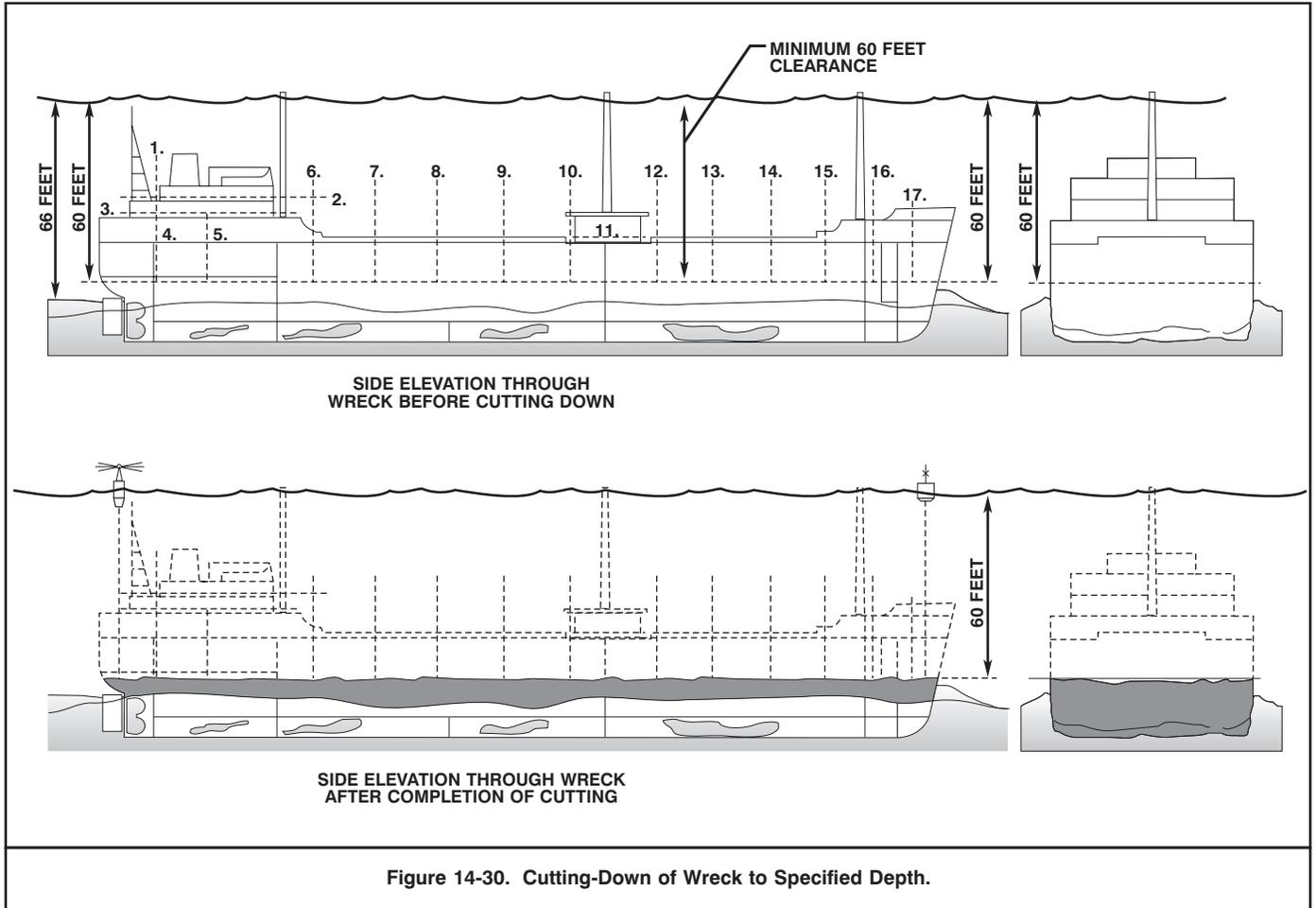
Figure 14-30. Cutting-Down of Wreck to Specified Depth.
