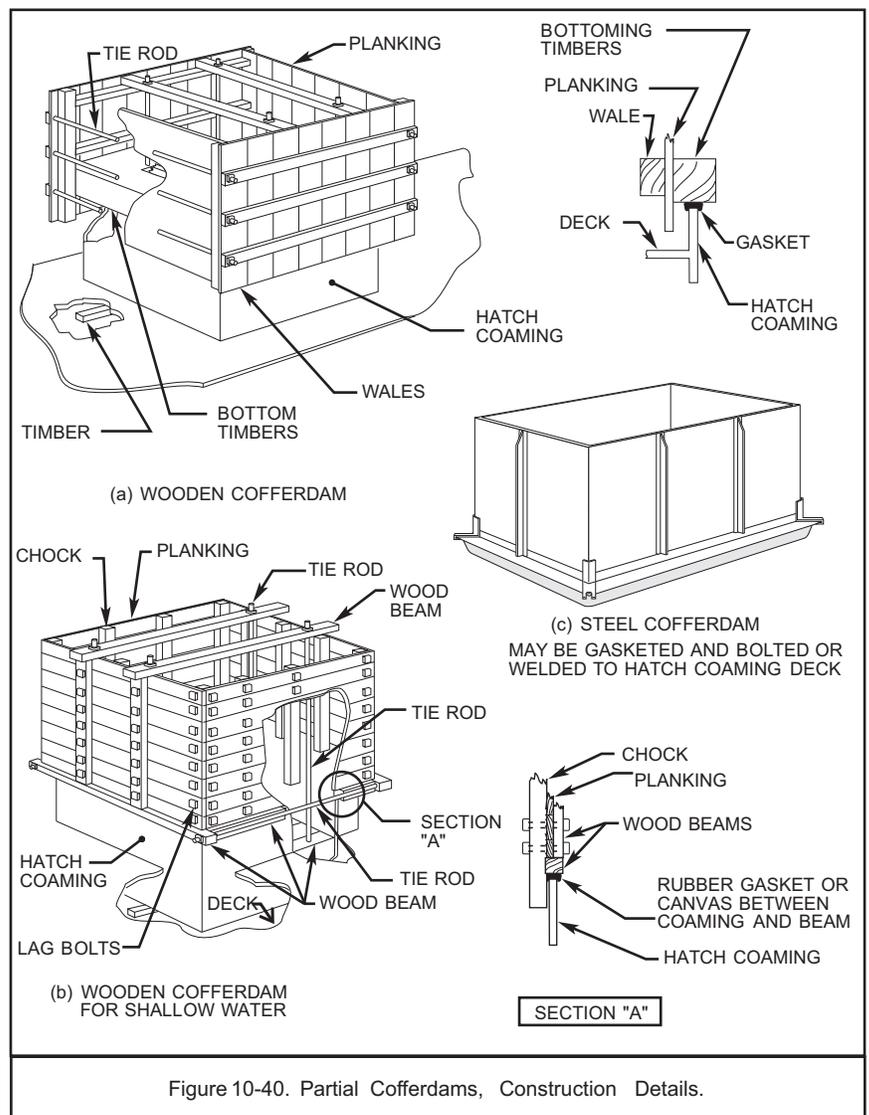
Figure 10-40. Partial Cofferdams, Construction Details.
