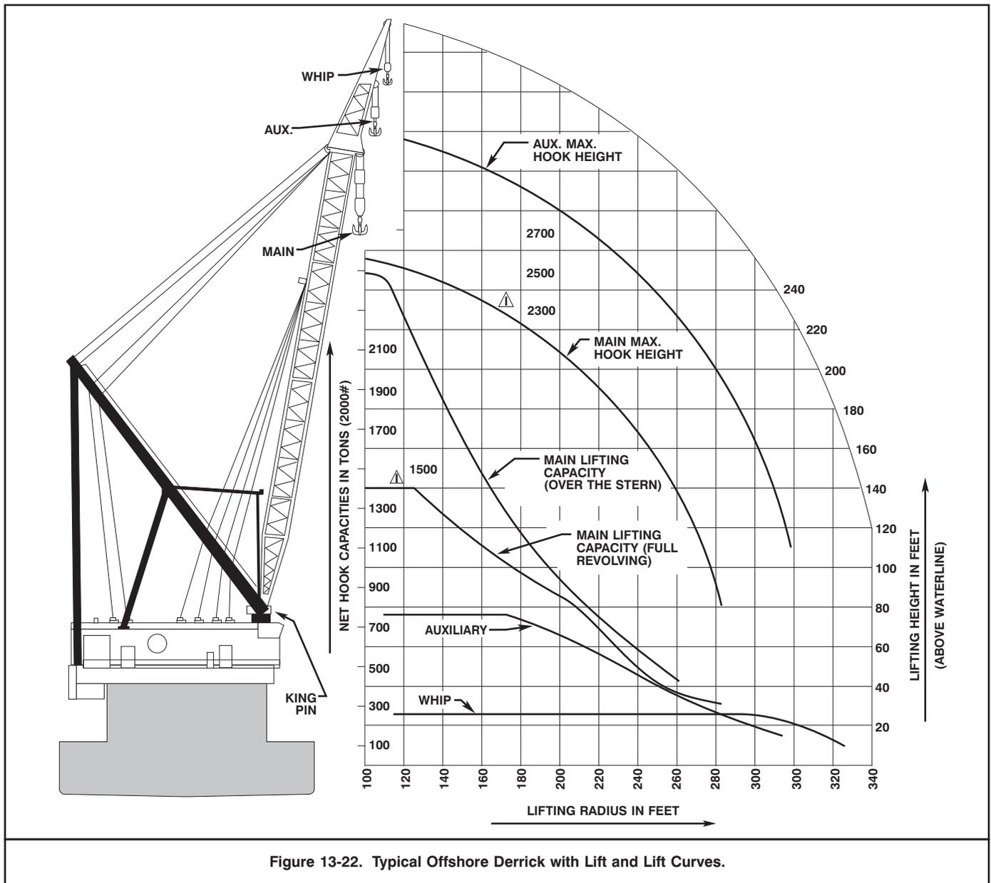
Figure 13-22. Typical Offshore Derrick with Lift and Lift Curves.
