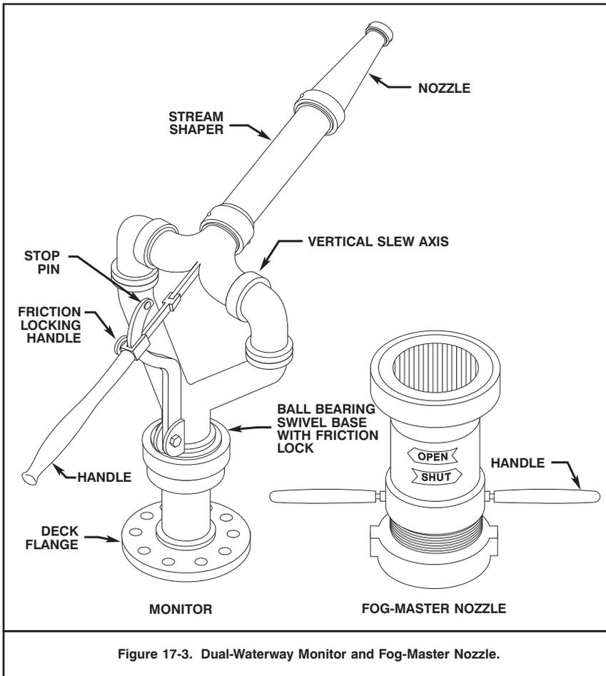
Figure 17-3. Dual-Waterway Monitor and Fog-Master Nozzle.
