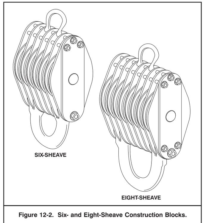
Figure 12-2. Six- and Eight-Sheave Construction Blocks.
