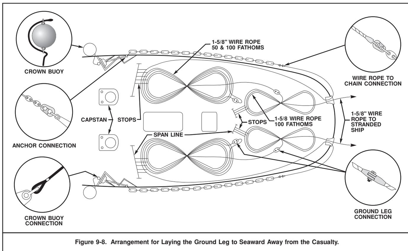
Figure 9-8. Arrangement for Laying the Ground Leg to Seaward Away from the Casualty.
