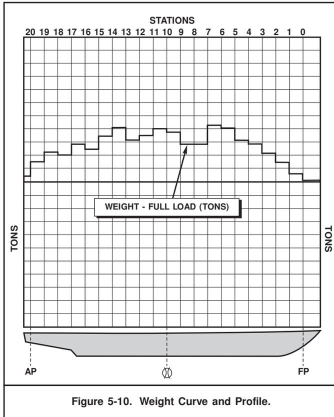
Figure 5-10. Weight Curve and Profile.
