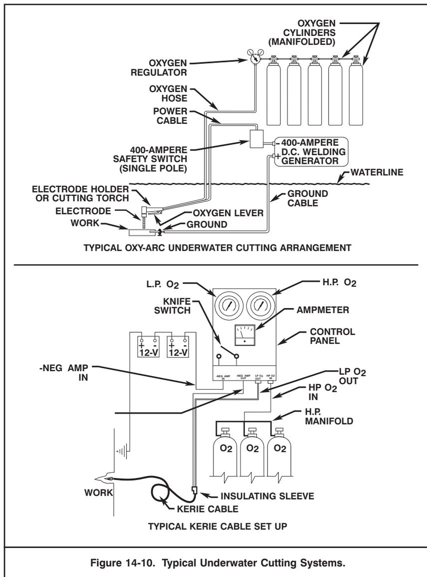
Figure 14-10. Typical Underwater Cutting Systems.
