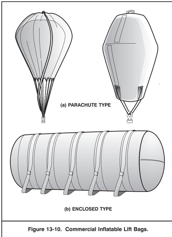
Figure 13-10. Commercial Inflatable Lift Bags.
