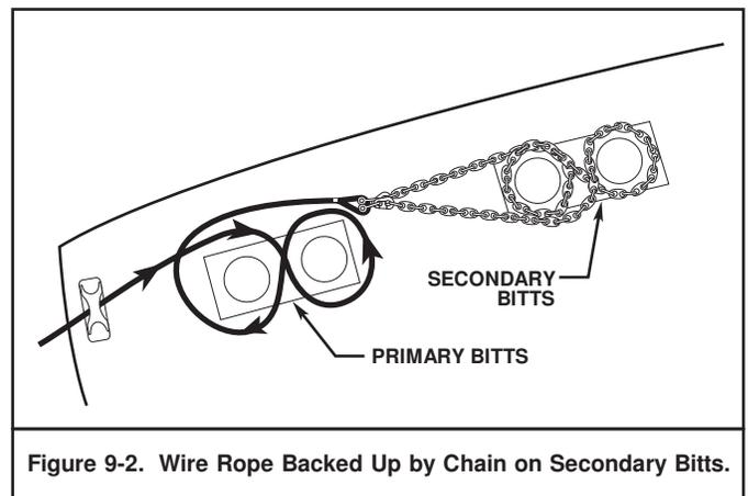
Figure 9-2. Wire Rope Backed Up by Chain on Secondary Bitts.
