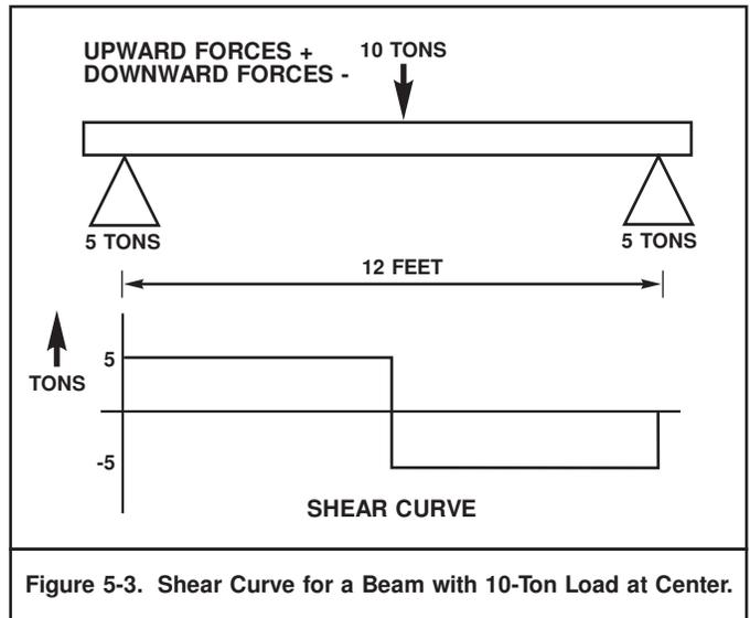
Figure 5-3. Shear Curve for a Beam with 10-Ton Load at Center.
