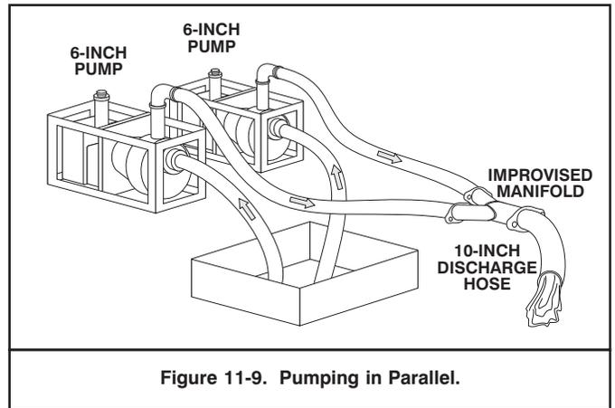
Figure 11-9. Pumping in Parallel.
