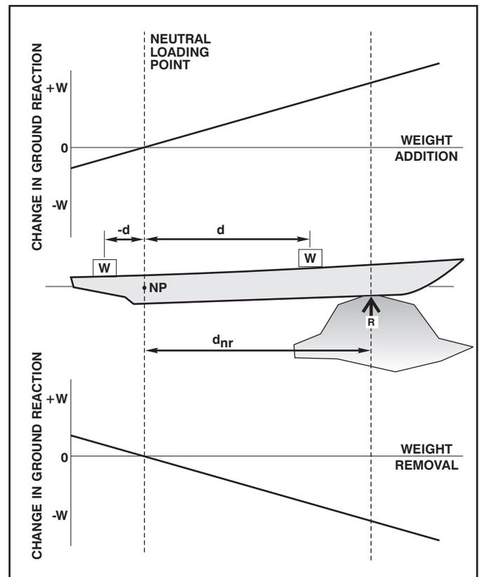
Figure 6-4. Effects of Weight Changes on Ground Reaction.
