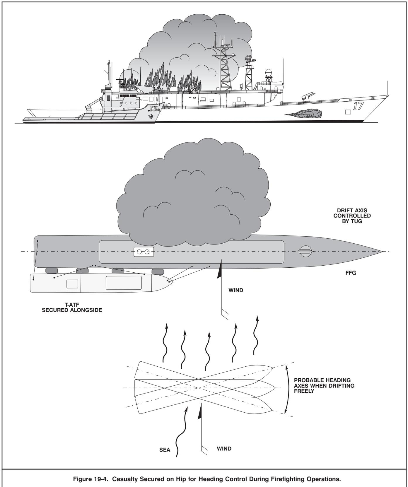
Figure 19-4. Casualty Secured on Hip for Heading Control During Firefighting Operations.
