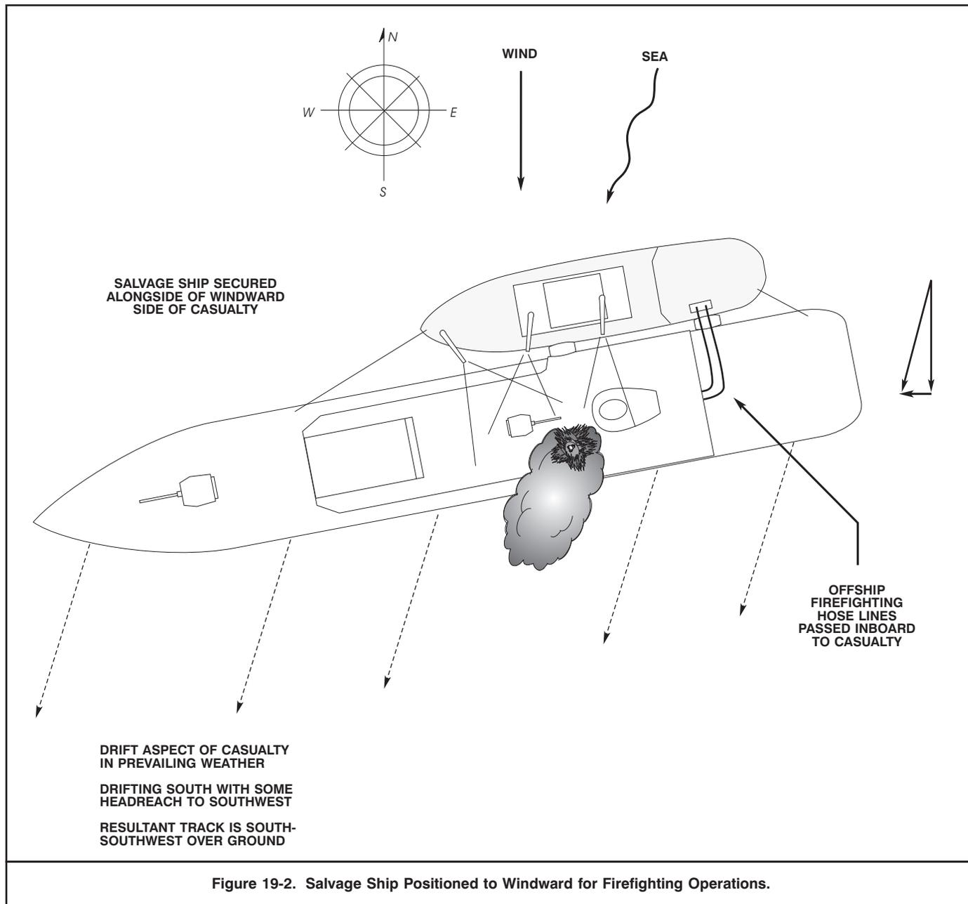
Figure 19-2 shows an assisting vessel moored alongside the windward side of a drifting small combatant, using both monitors and offship fire hoses for fire control and extinguishing. The decision as to whether the assisting vessel should make up to the casualty, as shown, or stand off depends on several factors:
