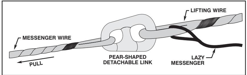
Figure 12-26. Wire Messengers Connected with Detachable Link.
