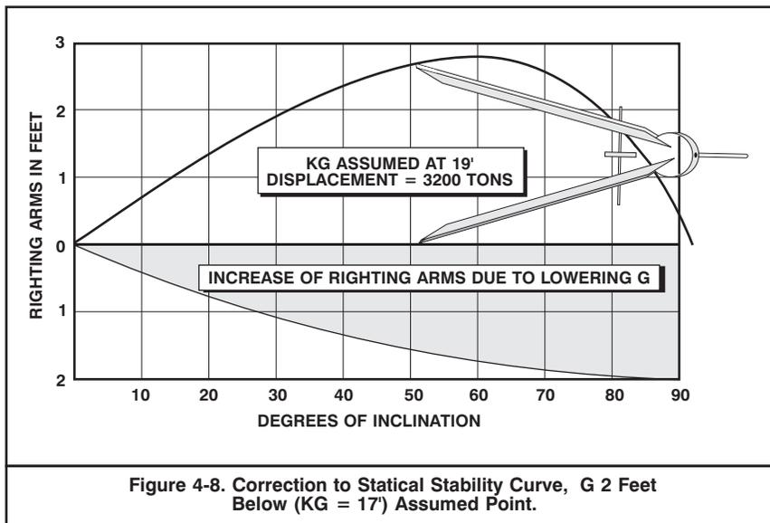
Figure 4-8. Correction to Statical Stability Curve, G 2 Feet Below (KG = 17') Assumed Point.
