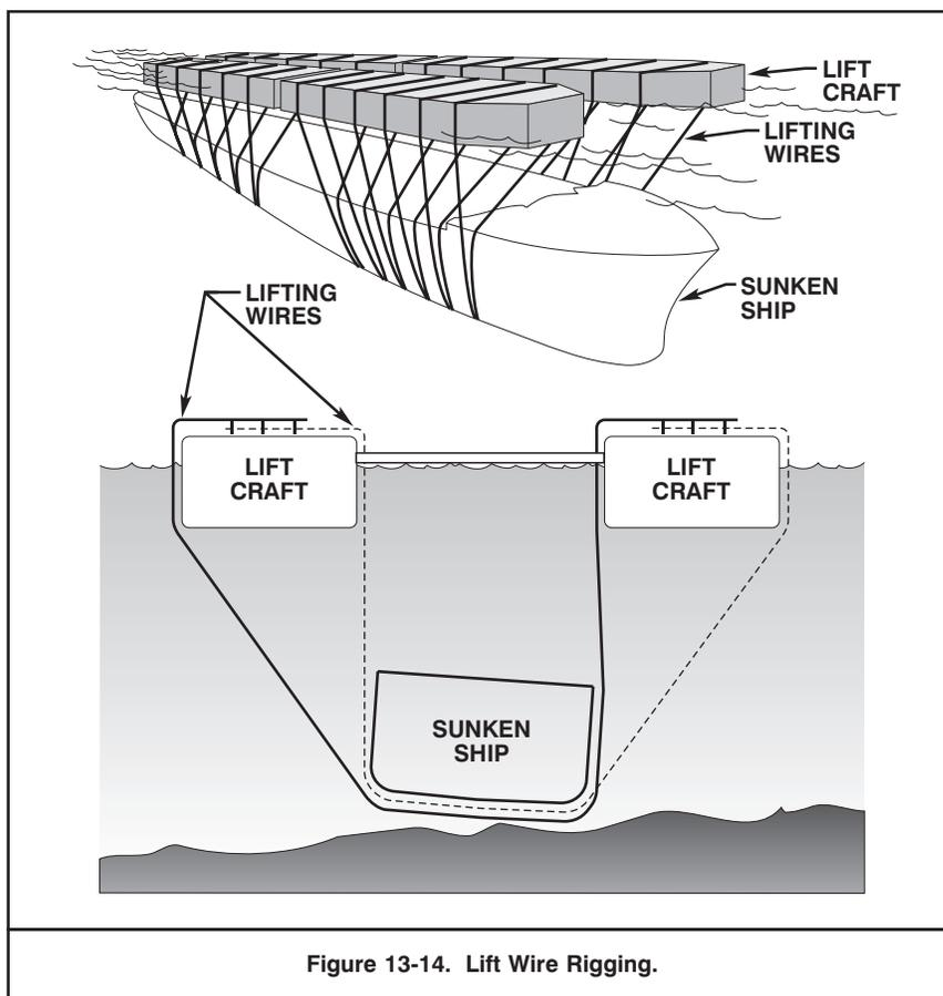
Figure 13-14. Lift Wire Rigging.
