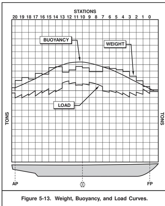
Figure 5-13. Weight, Buoyancy, and Load Curves.
