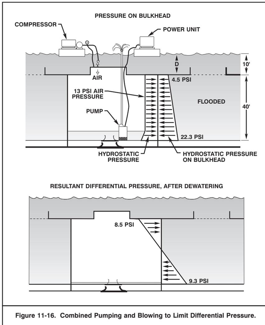
Figure 11-16 illustrates how the introduction of compressed air can lower differential pressure across the bulkhead of a compartment being dewatered between a compartment being dewatered and one open to the sea.
