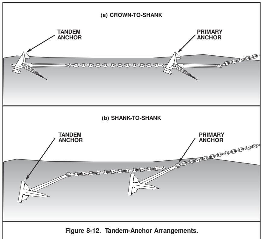
Figure 8-12. Tandem-Anchor Arrangements.
