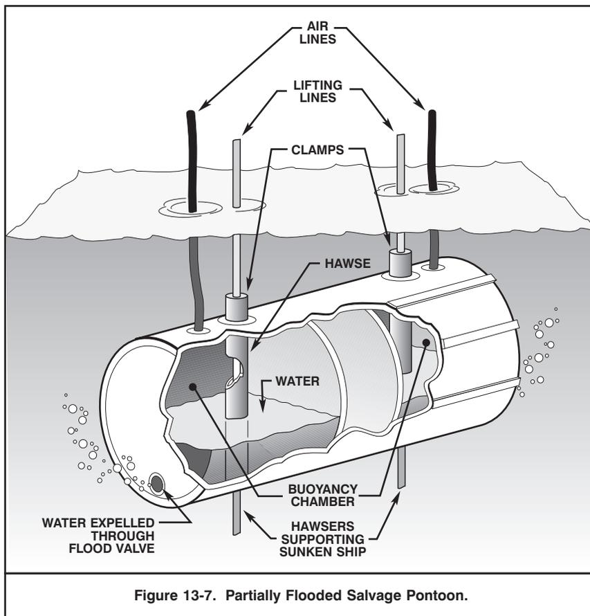
Figure 13-7. Partially Flooded Salvage Pontoon.
