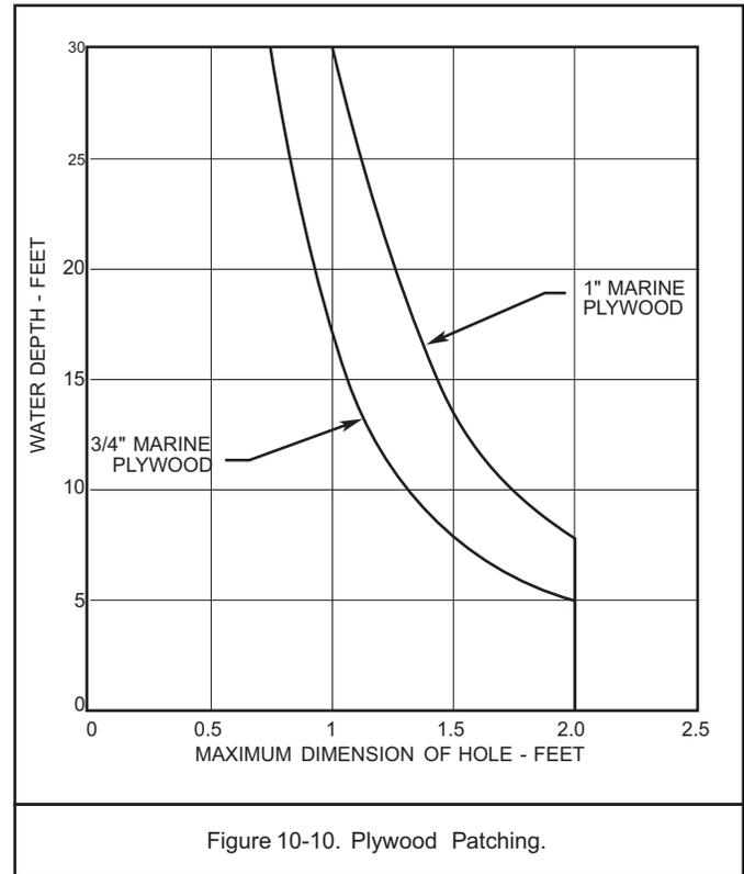
Figure 10-10. Plywood Patching.
