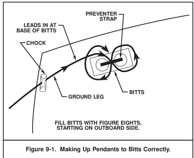
Figure 9-1. Making Up Pendants to Bitts Correctly.
