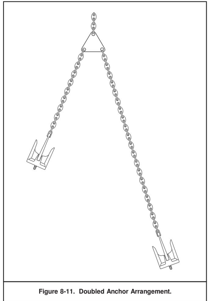
Figure 8-11. Doubled Anchor Arrangement.
