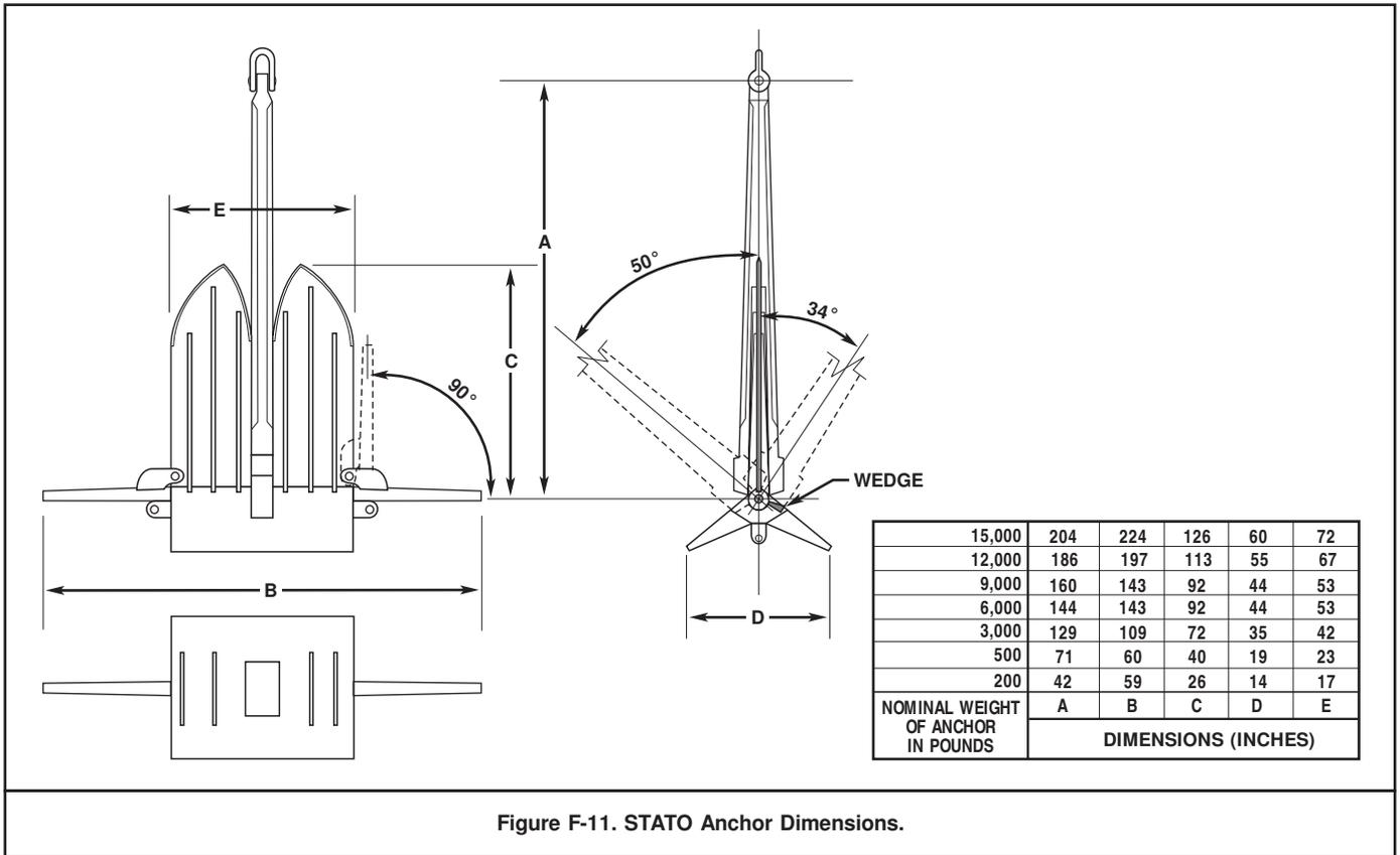
Figure F-11. STATO Anchor Dimensions.
