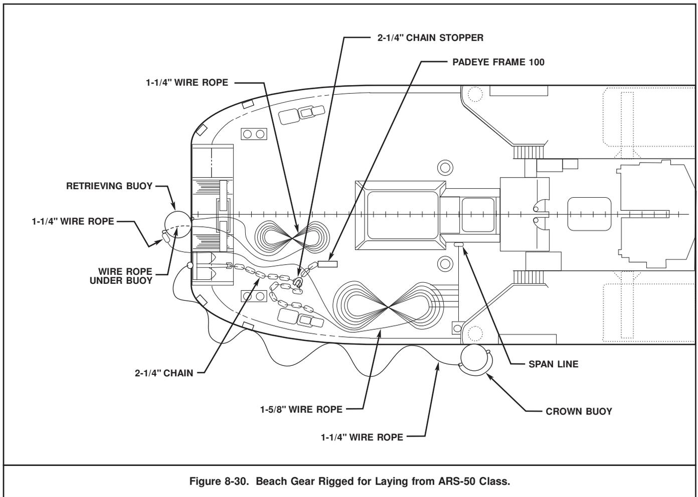
Figure 8-30. Beach Gear Rigged for Laying from ARS-50 Class.
