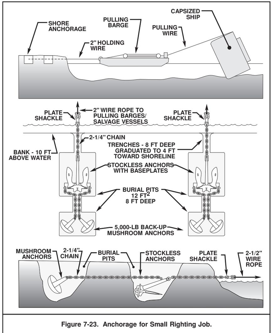
Figure 7-23. Anchorage for Small Righting Job.
