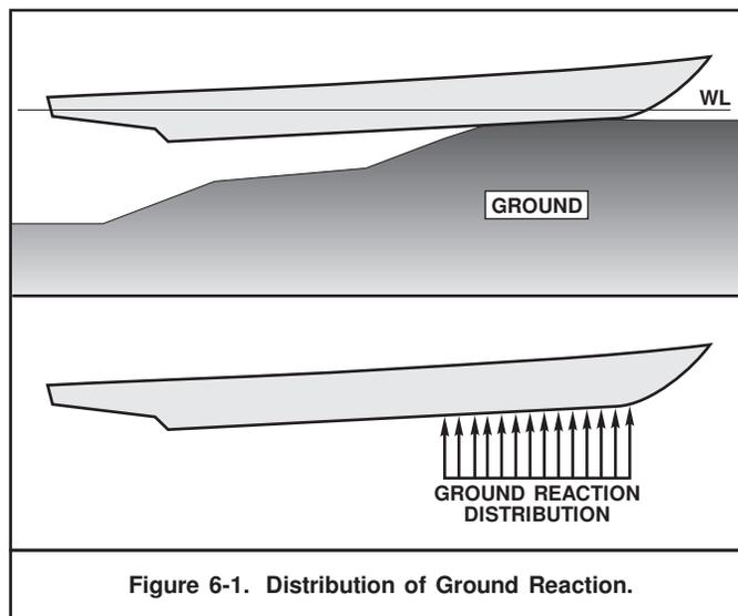
Figure 6-1. Distribution of Ground Reaction.
