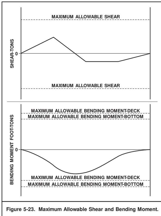
Figure 5-23. Maximum Allowable Shear and Bending Moment.
