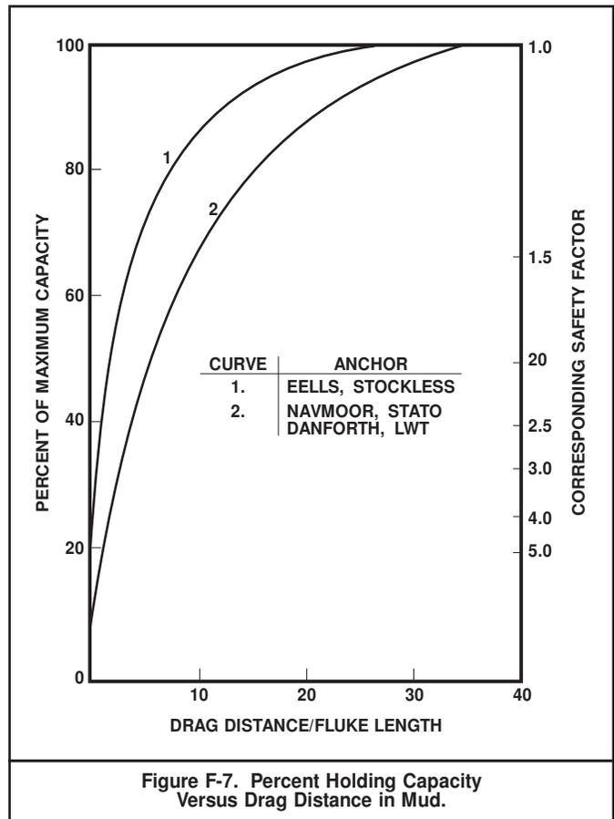
Figure F-7. Percent Holding Capacity Versus Drag Distance in Mud.
