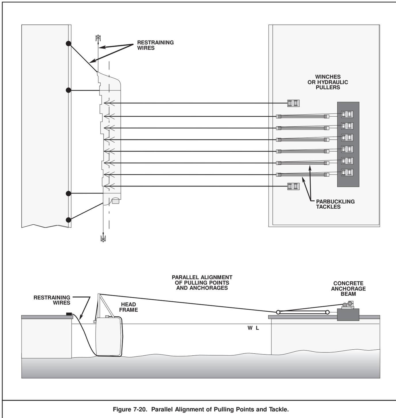
**7-8.4.1 Headframe Attachment Position.** To ensure that each purchase or pulling system develops almost identical righting moments, headframe top and hauling system anchorage point baselines must be in the same plane. To achieve this, it is customary to locate all headframe attachment positions on the capsized ship's parallel midbody.
