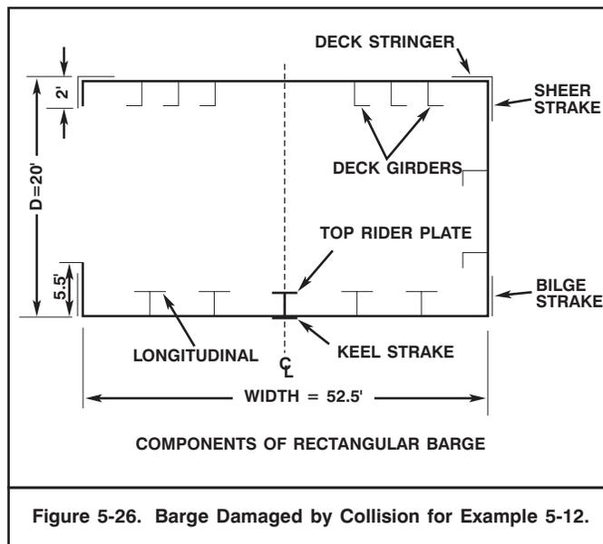
Figure 5-26. Barge Damaged by Collision for Example 5-12.
