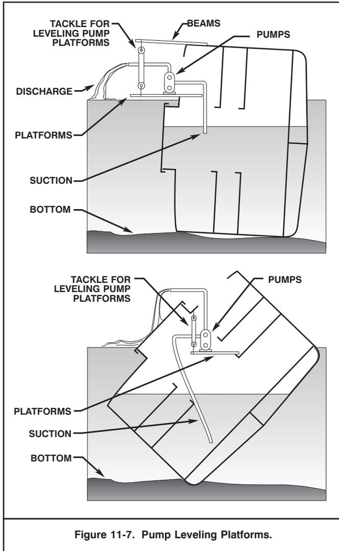
Figure 11-7. Pump Leveling Platforms.
