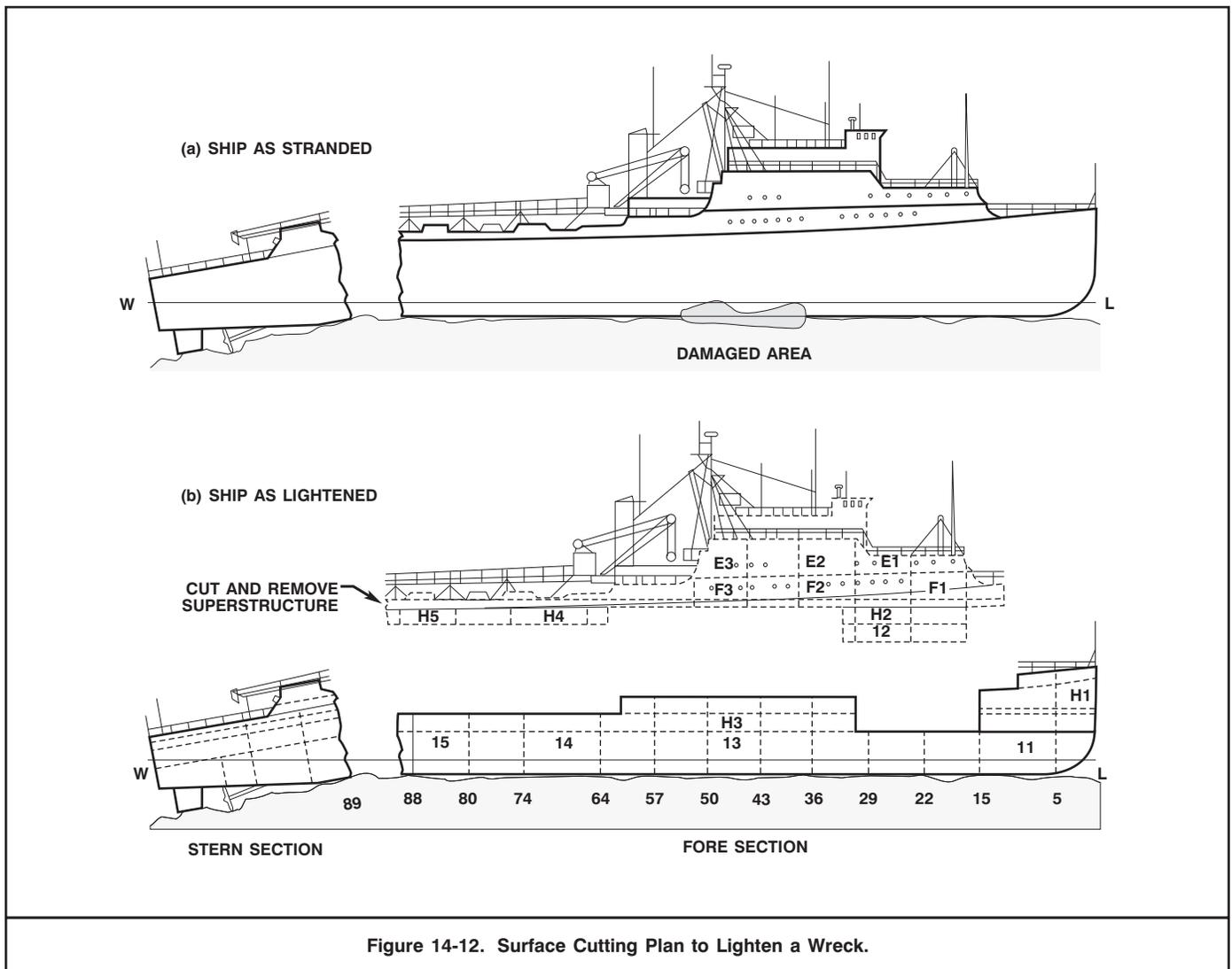
As each area is stripped and prepared for cutting, preparation teams move down in the wreck until they reach the water line. Final dry cut lines are set at either the high or low water mark, depending upon the tide range and the wreck location.
