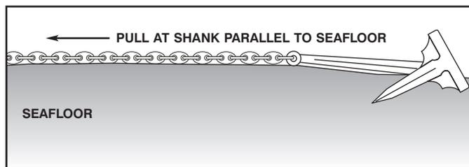
Figure 8-8. Chain Holding Anchor Shank Parallel to Seafloor.
