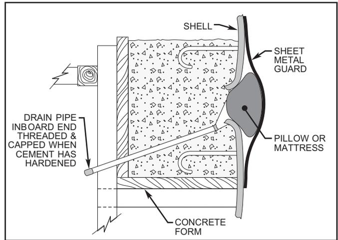
Figure 10-30. Typical Drain Pipe Installation.
