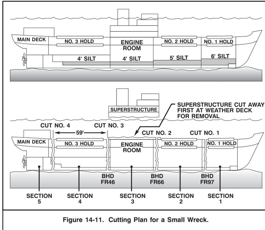
Figure 14-11. Cutting Plan for a Small Wreck.
