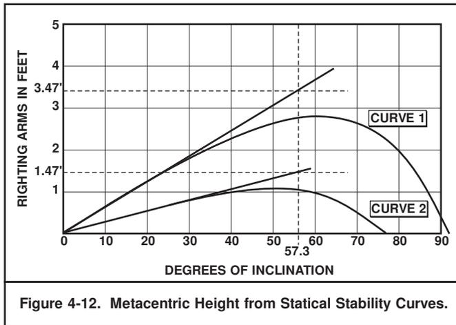
Figure 4-12. Metacentric Height from Statical Stability Curves.
