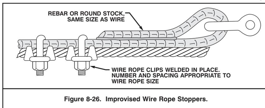
Figure 8-26. Improved Wire Rope Stoppers.
