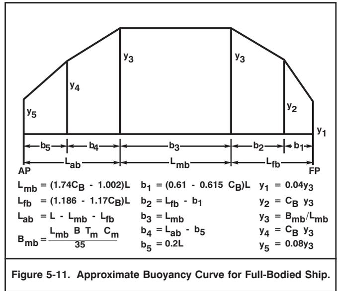
Figure 5-11. Approximate Buoyancy Curve for Full-Bodied Ship.
