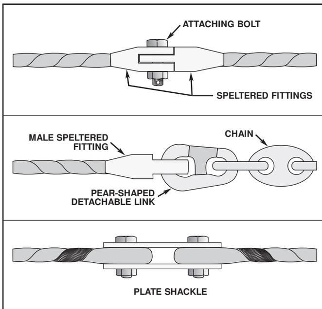
Figure 8-21. Connections for Ground Leg.
