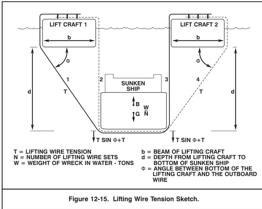
Figure 12-15. Lifting Wire Tension Sketch.
