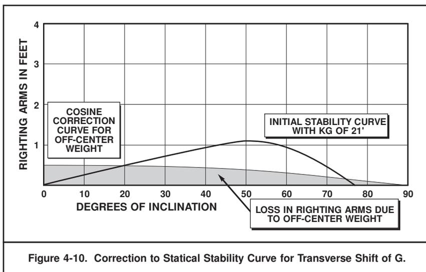
Figure 4-10. Correction to Statical Stability Curve for Transverse Shift of G.
