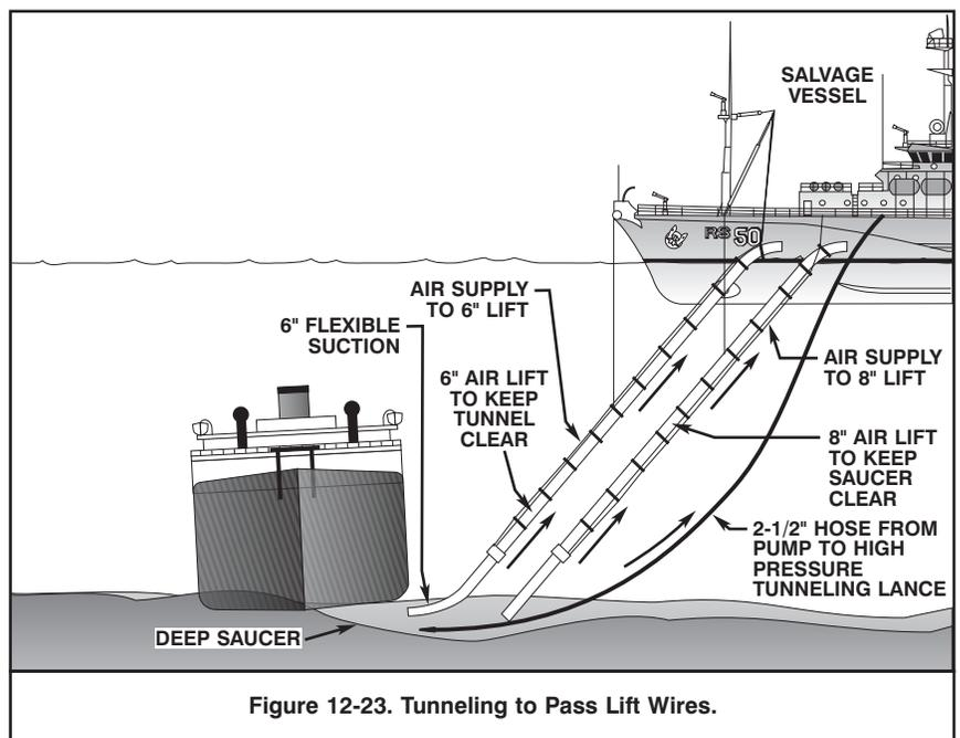
Figure 12-23. Tunneling to Pass Lift Wires.
