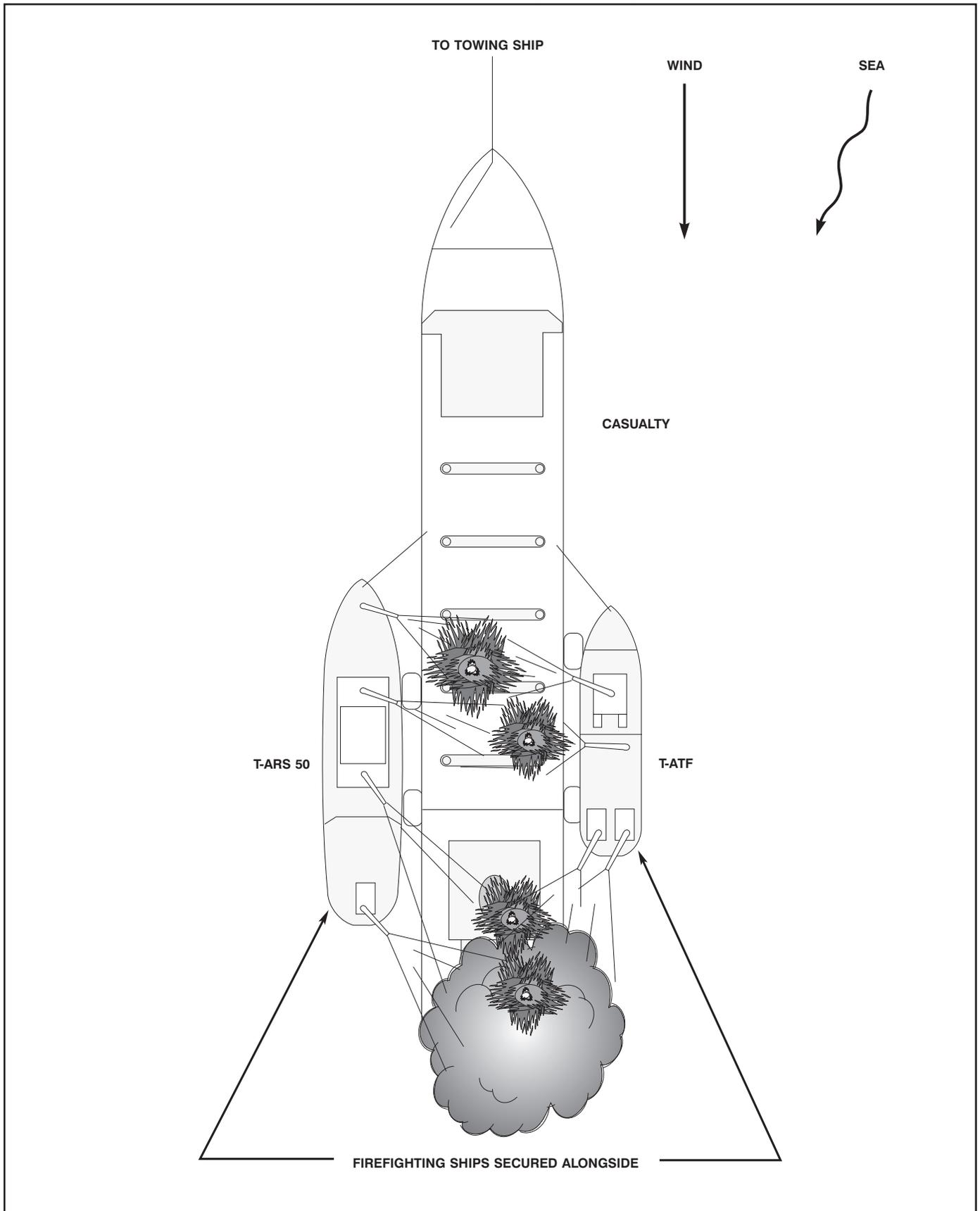
Figure 19-3. Optimum Configuration for Fighting Fires on Large Oil Carrier.
