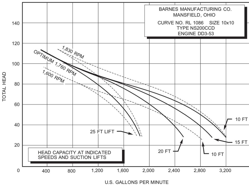
Figure H-3. Performance Curve, 10-Inch Diesel Pump.
