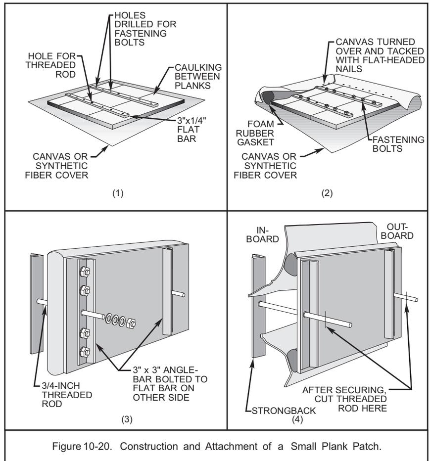
Figure 10-20. Construction and Attachment of a Small Plank Patch.
