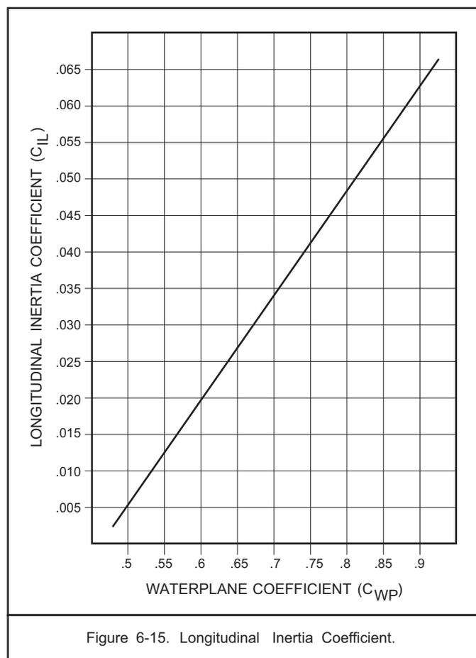
Figure 6-15. Longitudinal Inertia Coefficient.
