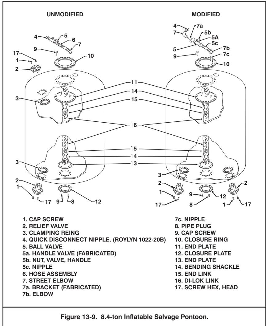
Figure 13-9. 8.4-ton Inflatable Salvage Pontoon.
