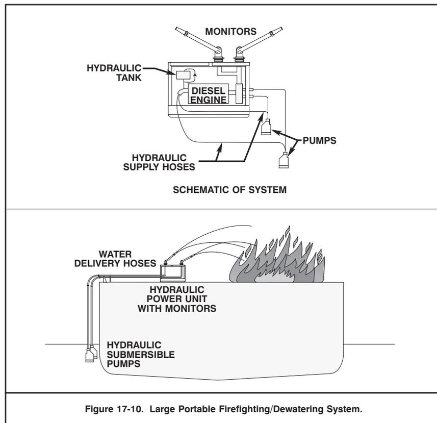
Figure 17-10. Large Portable Firefighting/Dewatering System.
