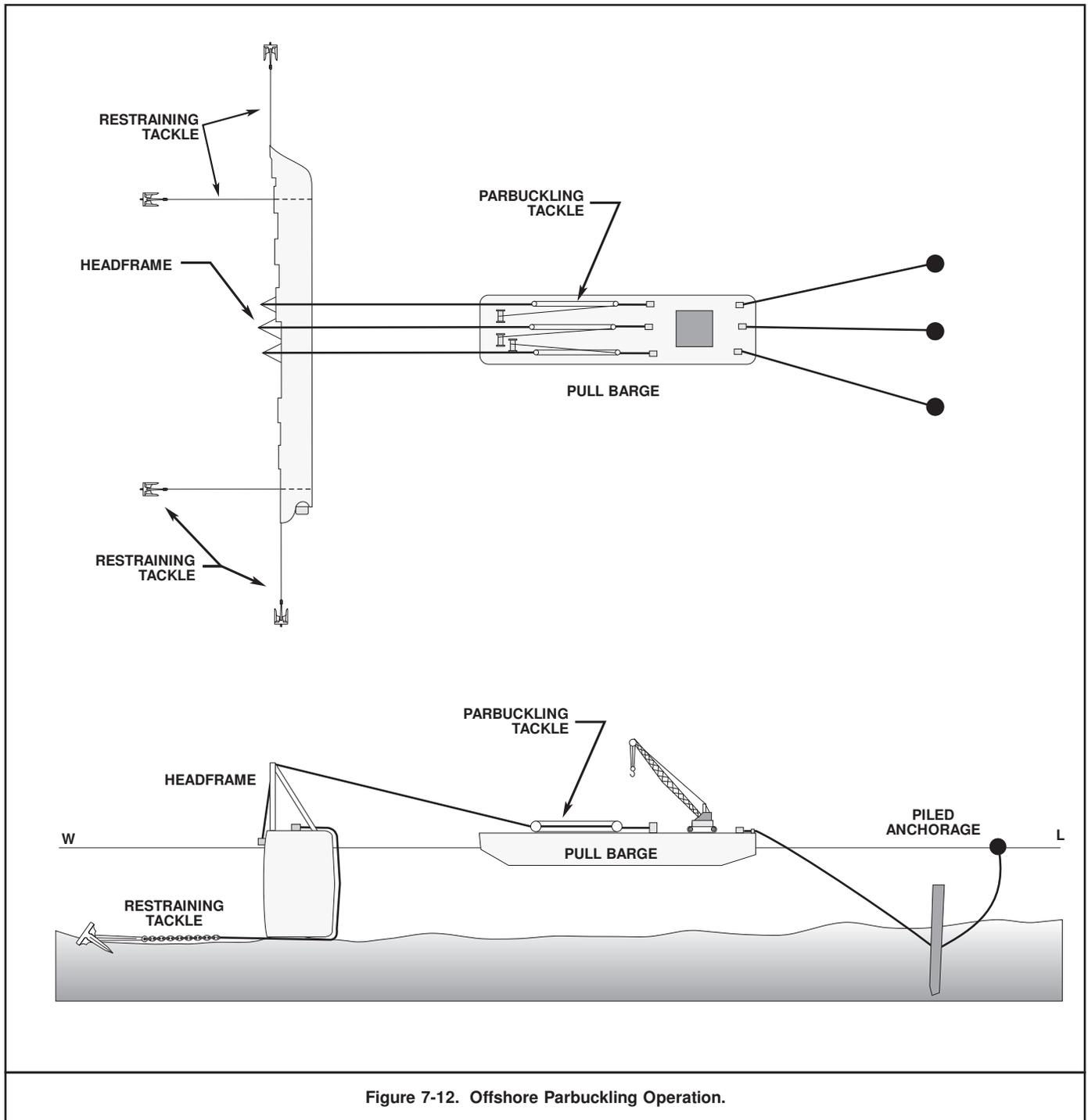
Figure 7-12. Offshore Parbuckling Operation.
