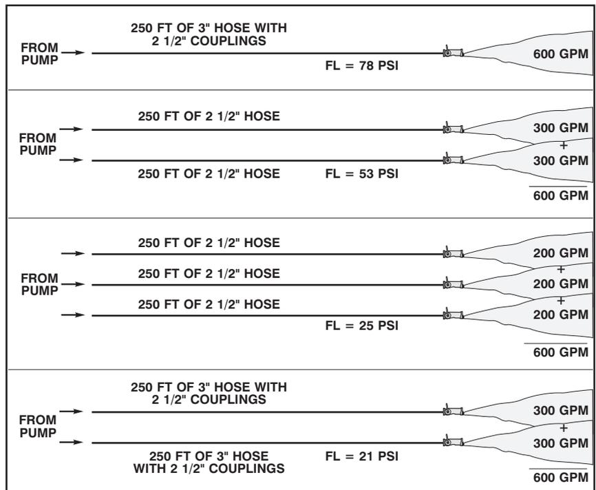
Figure 16-6B. Minimizing Friction Loss.
