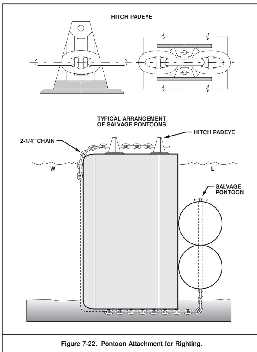
Figure 7-22. Pontoon Attachment for Righting.
