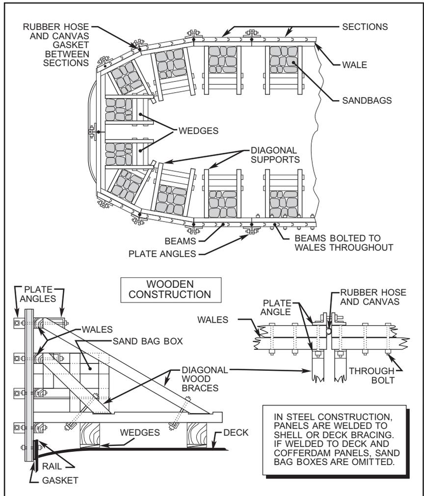
Figure 10-38. Complete Cofferdam Construction Details.
