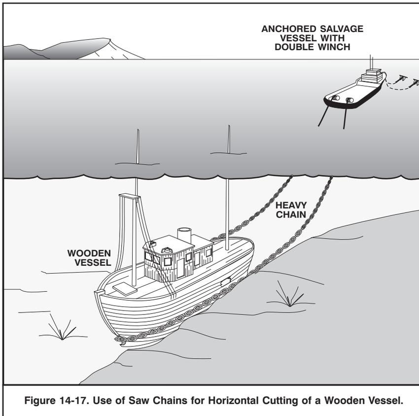
Figure 14-17. Use of Saw Chains for Horizontal Cutting of a Wooden Vessel.
