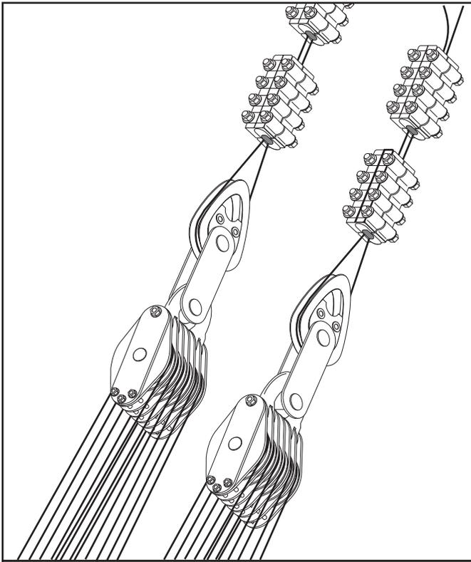
Figure 12-10. Lift Wires Made Up with Bullivant Clamps.
