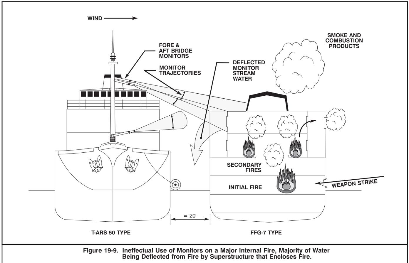
Figure 19-9 shows how a large percentage of water stream projected by monitors is wasted against steel superstructures and impenetrable barriers on a smaller combatant.
