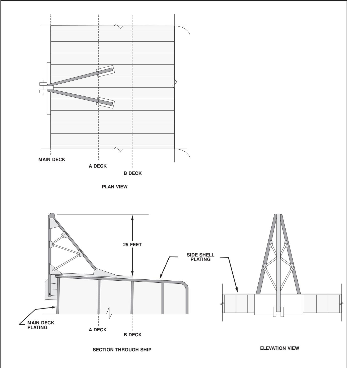
Figure 7-14. Braced-Girder Headframe.
