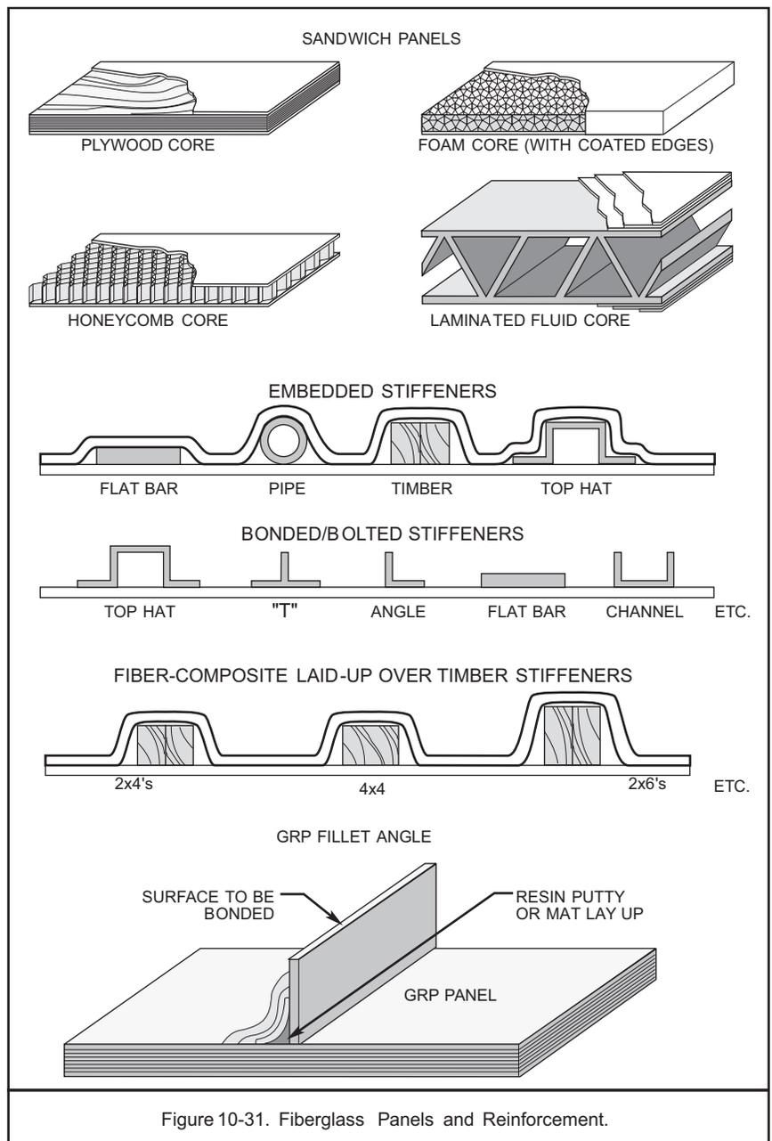
Figure 10-31. Fiberglass Panels and Reinforcement.
