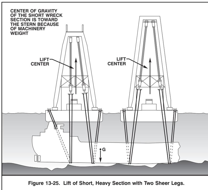
Figure 13-25. Lift of Short, Heavy Section with Two Sheer Legs.
