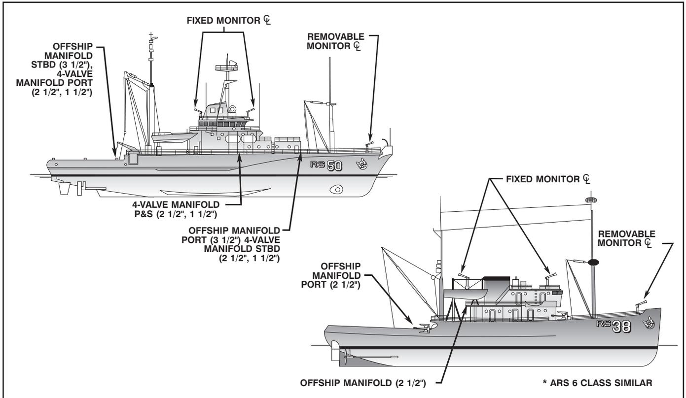
Figure 17-2A. Salvage Ship Offship Firefighting Systems.
