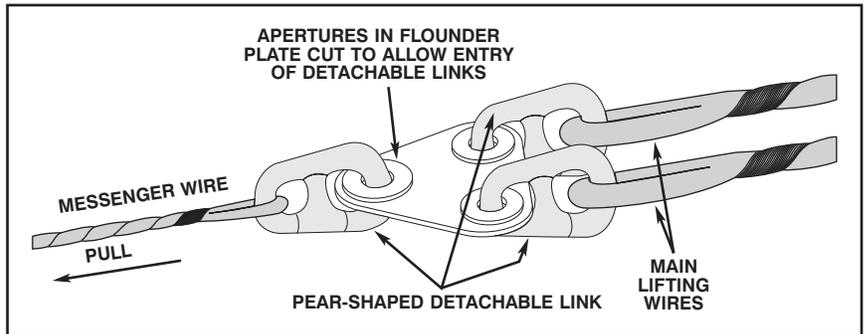
Figure 12-27A. Wire Rigged to Flounder Plate for Passing.
