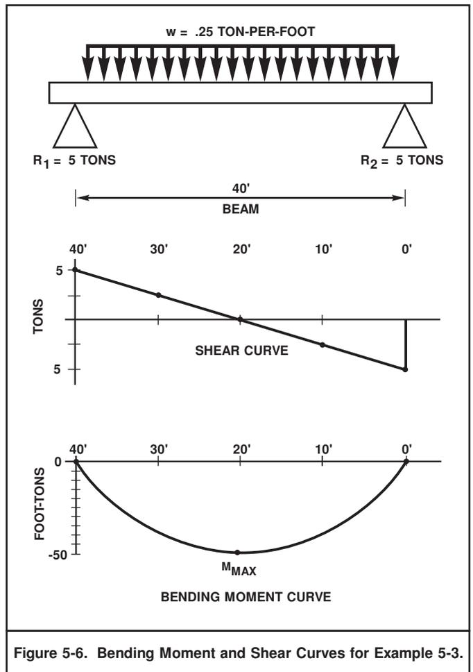
Figure 5-6. Bending Moment and Shear Curves for Example 5-3.
