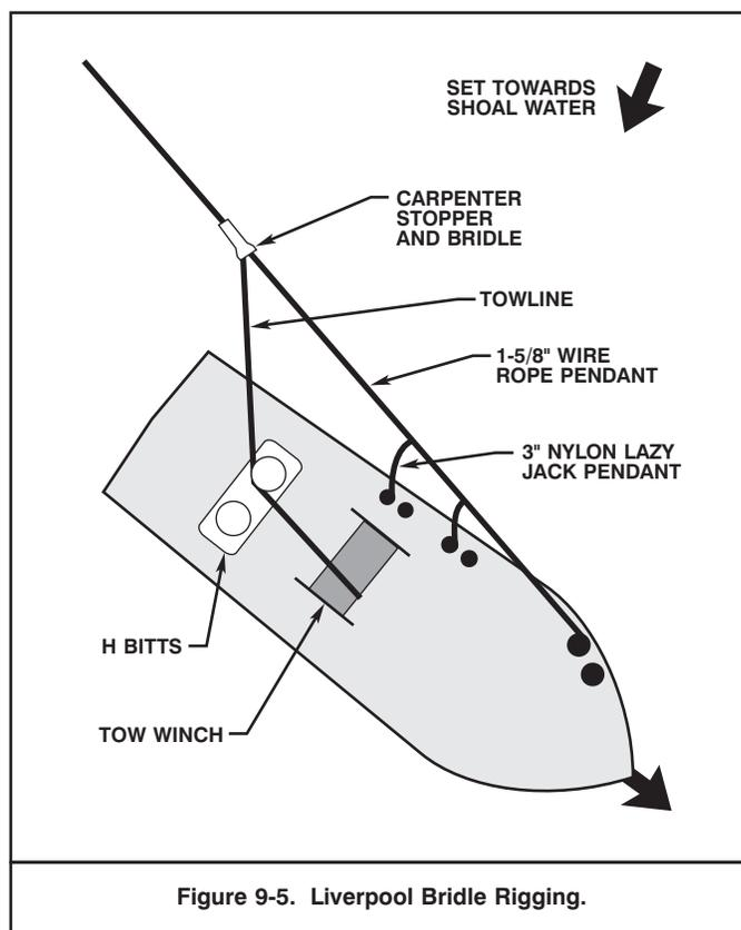
Figure 9-5. Liverpool Bridle Rigging.
