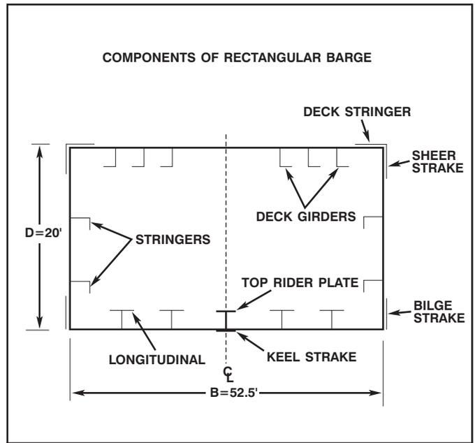
Figure 5-22. Cross Section of a Barge for Example 5-7.
