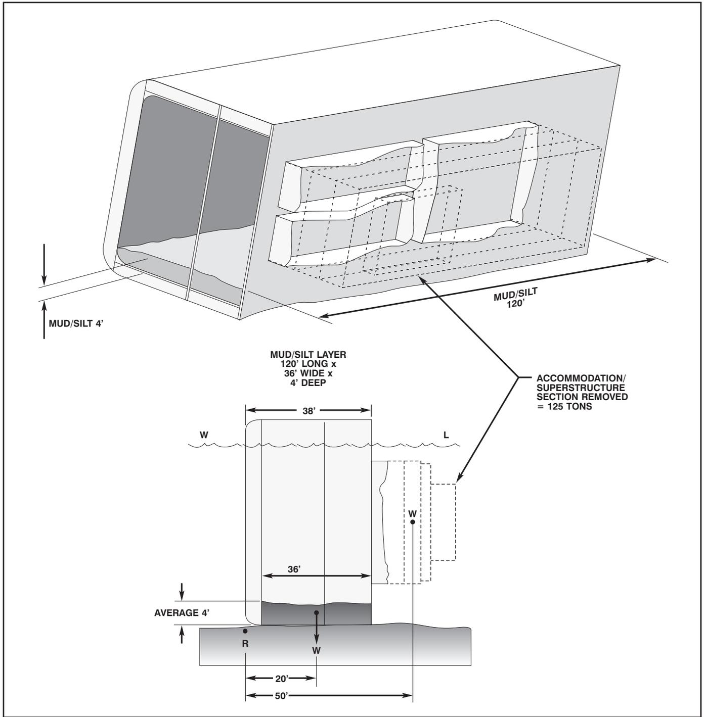
Figure 7-27. Measurements for Weight Removal.
