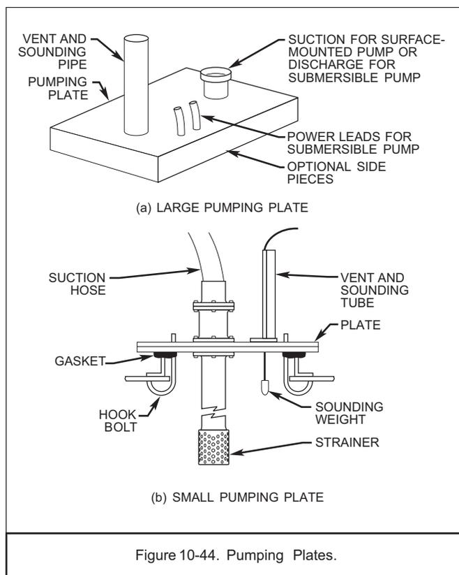
Figure 10-44 shows the features of pumping plates.
