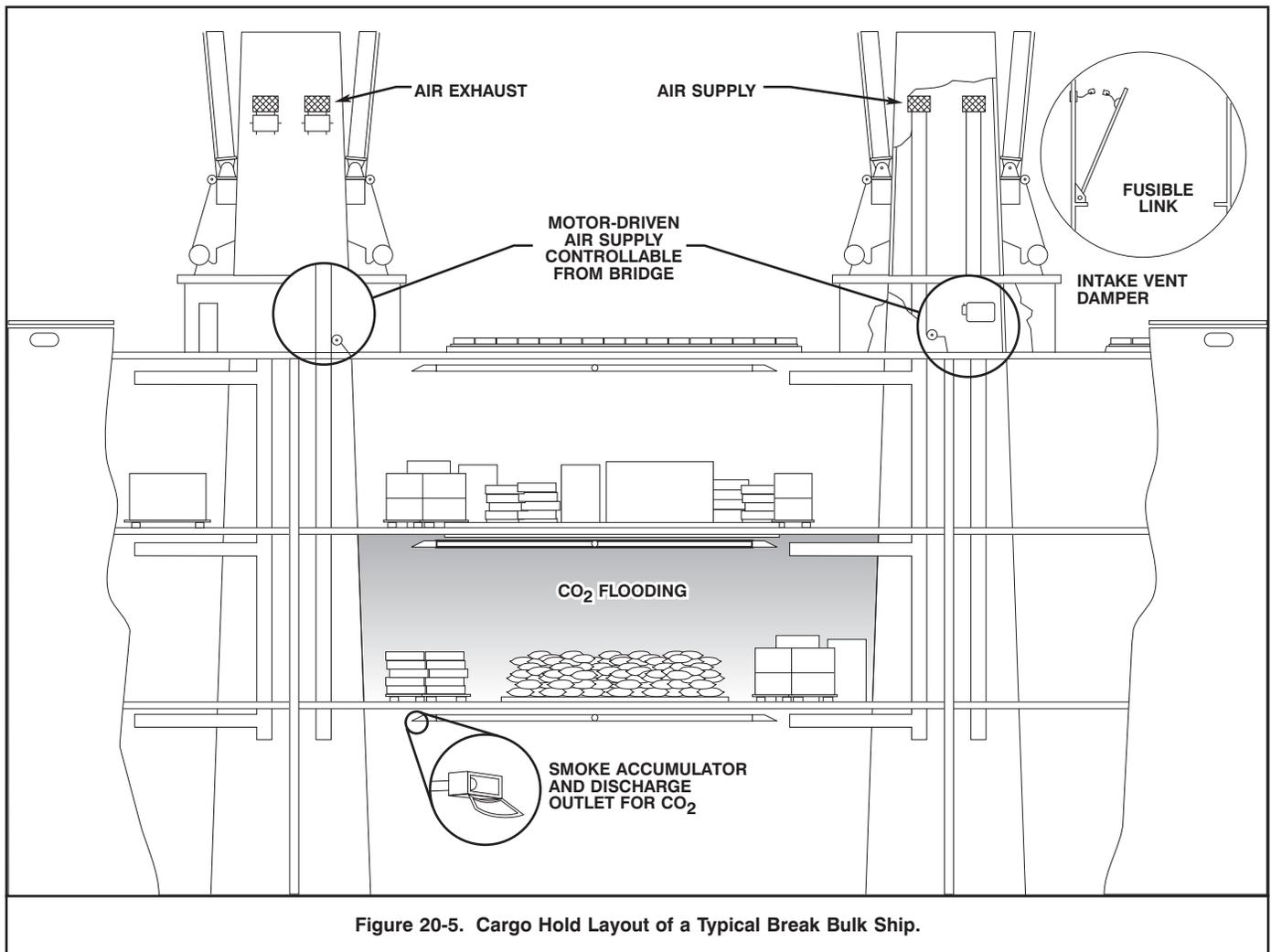
Figure 20-5. Cargo Hold Layout of a Typical Break Bulk Ship.
