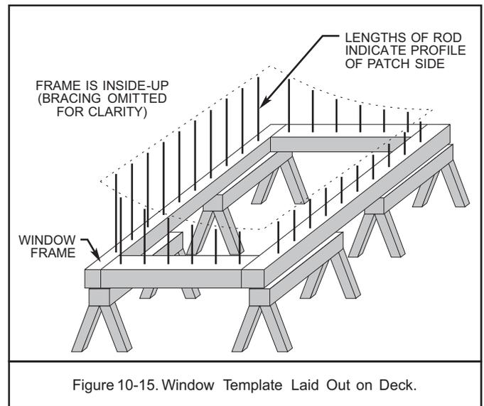
Figure 10-15. Window Template Laid Out on Deck.
