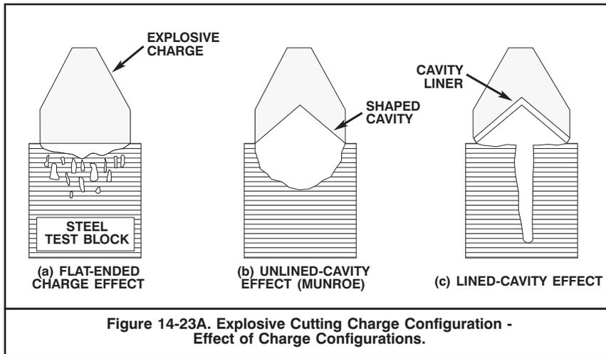
Figure 14-23A. Explosive Cutting Charge Configuration - Effect of Charge Configurations.
