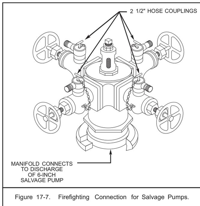
Figure 17-7. Firefighting Connection for Salvage Pumps.
