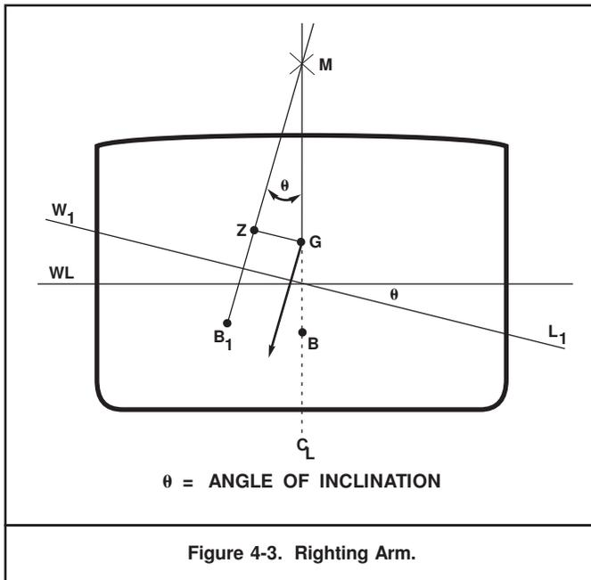
The length of the righting arm varies with the angle of inclination. The ratio of the righting arm to the metacentric height,  $GZ/GM$ , is equal to the sine of the angle for any small angle. If the sine of the angle is represented by  $\text{Sin } \theta$ , the equation can be written as:
