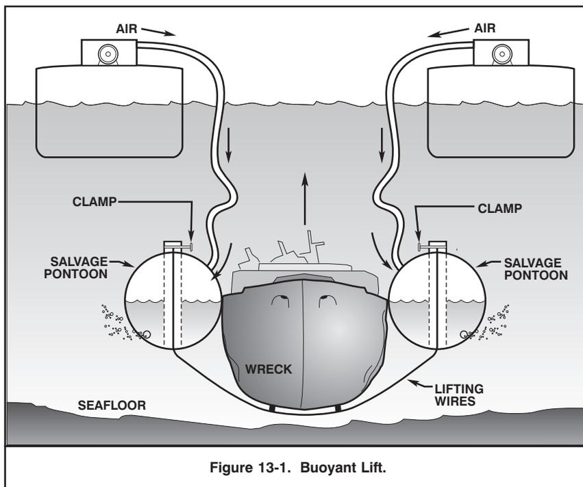
Figure 13-1. Buoyant Lift.
