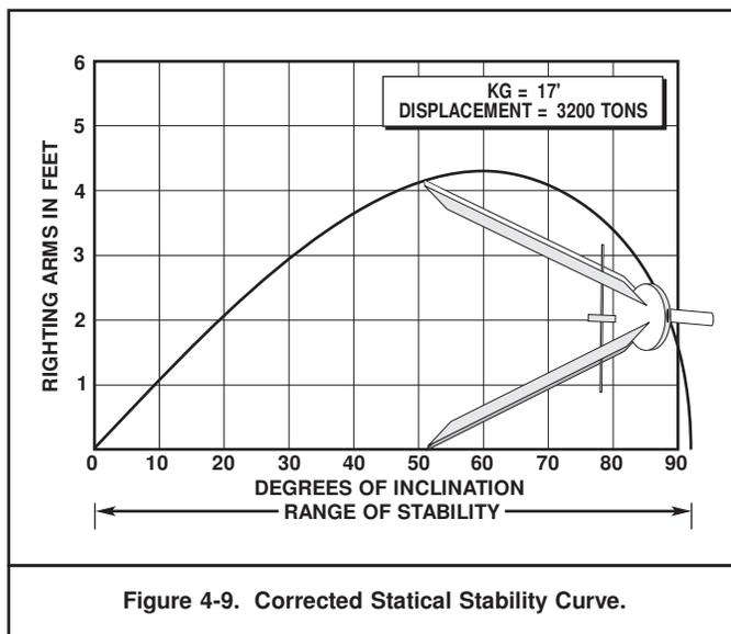
Figure 4-9. Corrected Statical Stability Curve.
