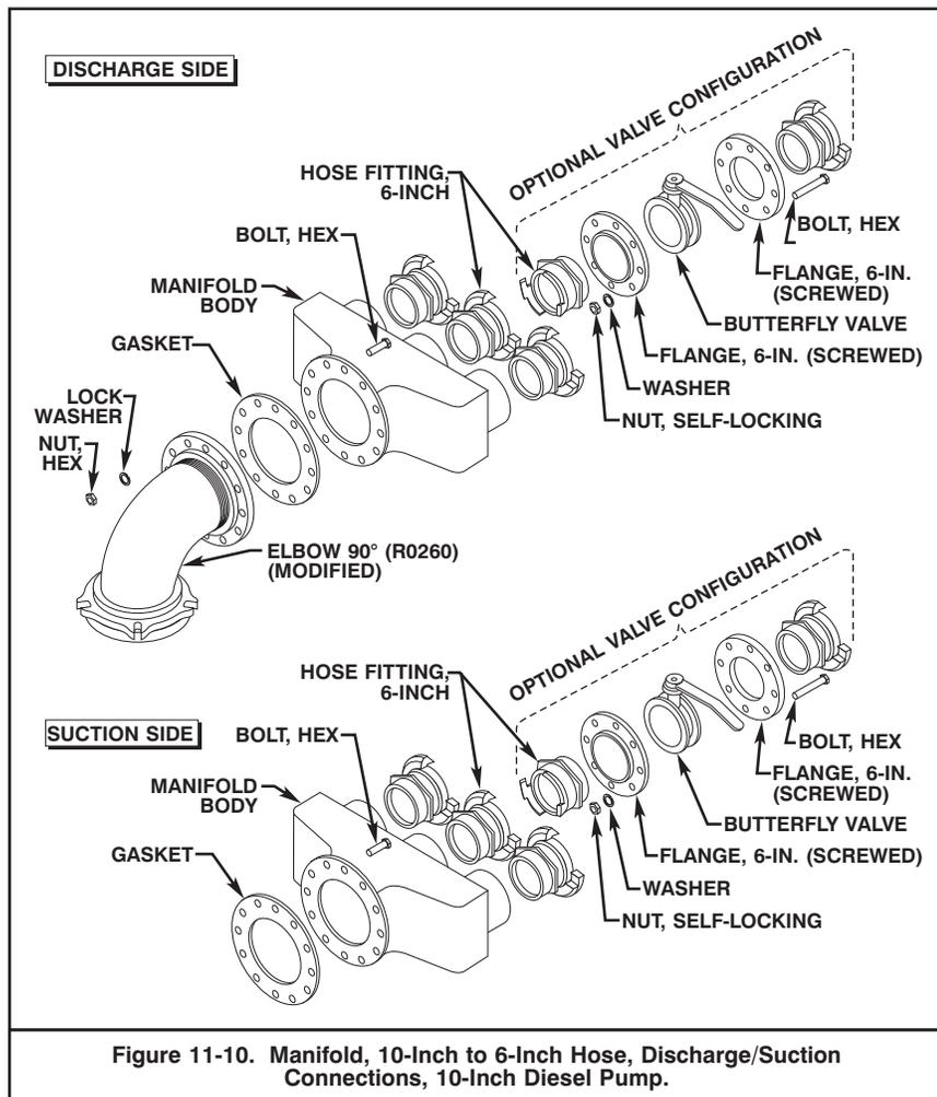
Figure 11-10. Manifold, 10-Inch to 6-Inch Hose, Discharge/Suction Connections, 10-Inch Diesel Pump.
