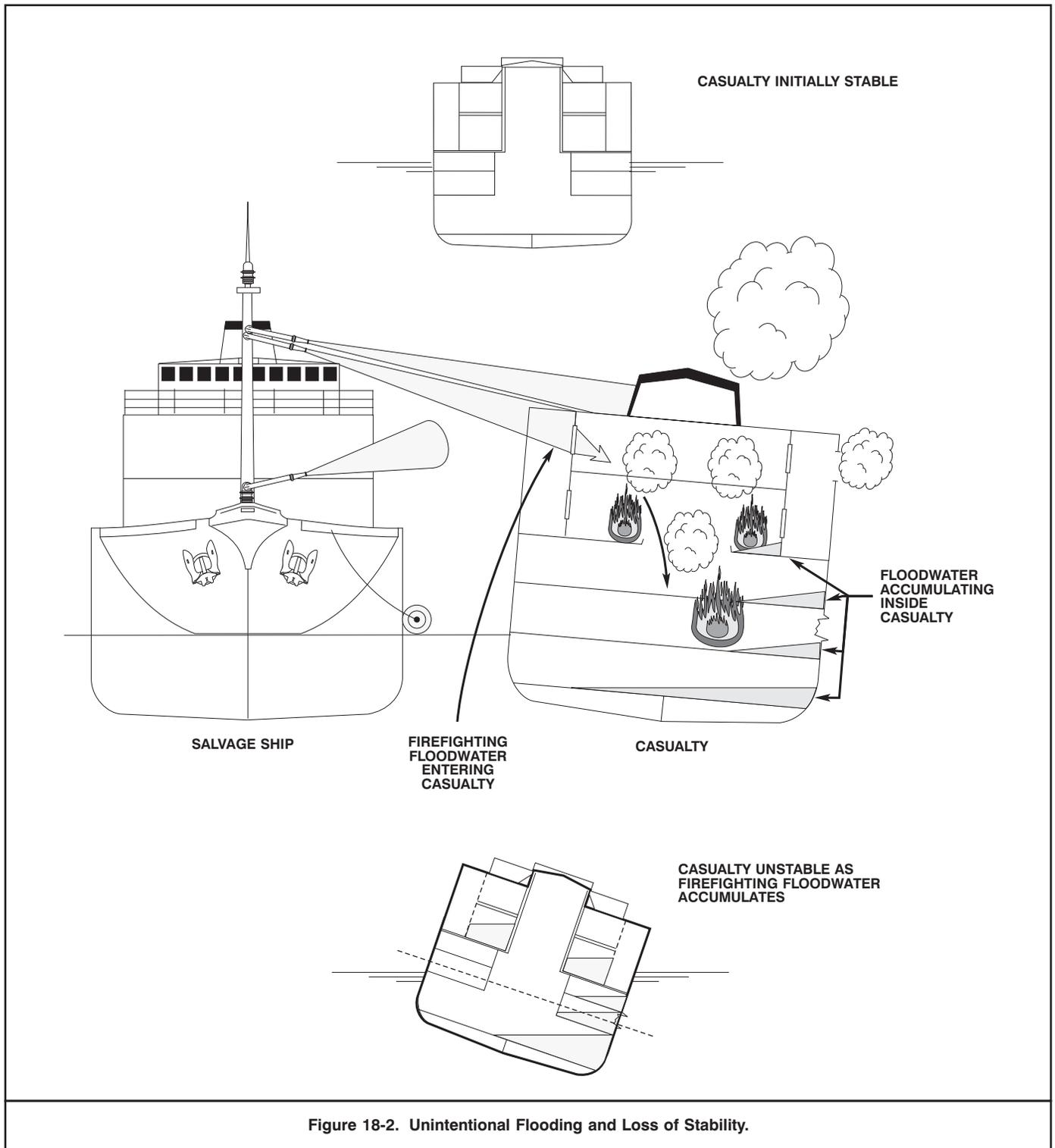
**Figure 18-2. Unintentional Flooding and Loss of Stability.**
