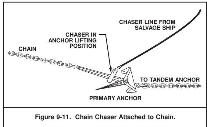
Figure 9-11. Chain Chaser Attached to Chain.
