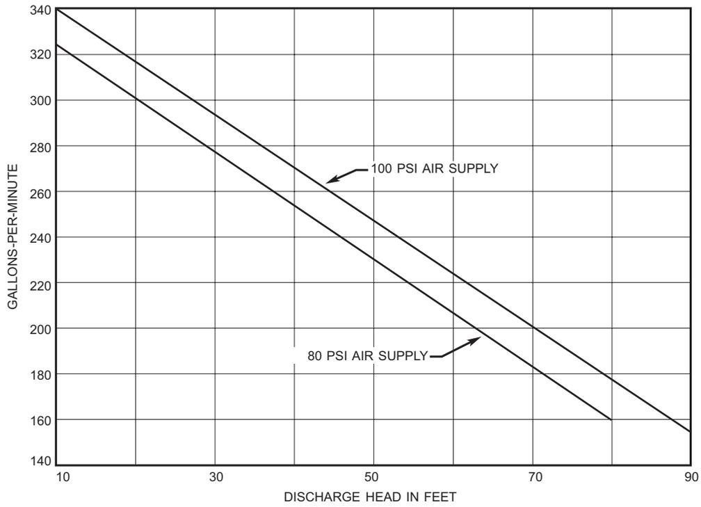
Figure H-4. 2 1/2-Inch Pneumatic Submersible Pump Performance Curves.
