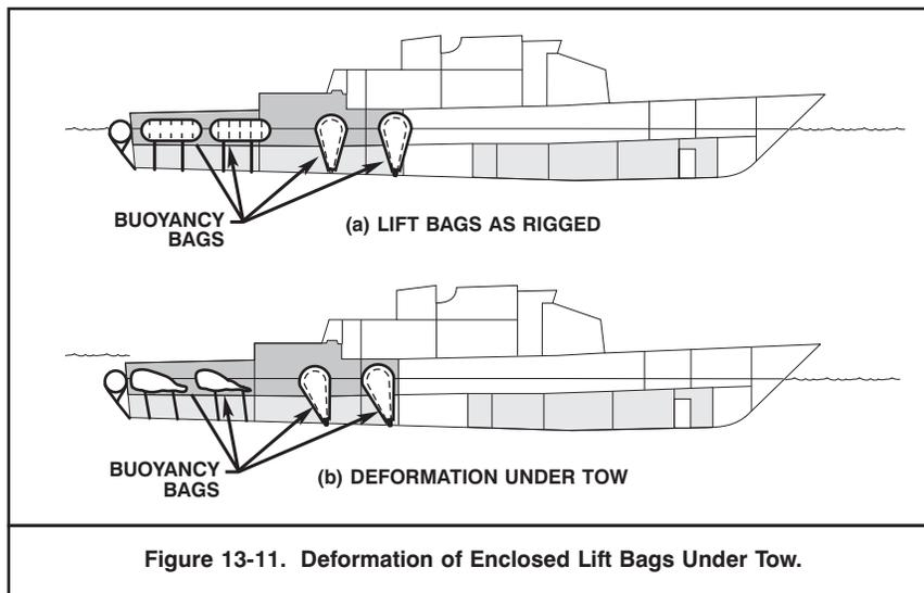
Figure 13-11. Deformation of Enclosed Lift Bags Under Tow.
