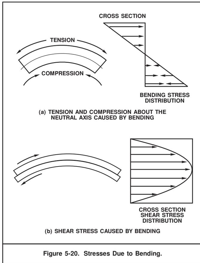
Figure 5-20. Stresses Due to Bending.
