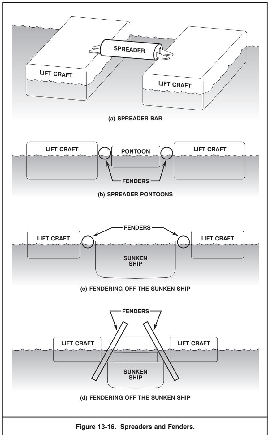
Figure 13-16. Spreader Bars and Fenders.
