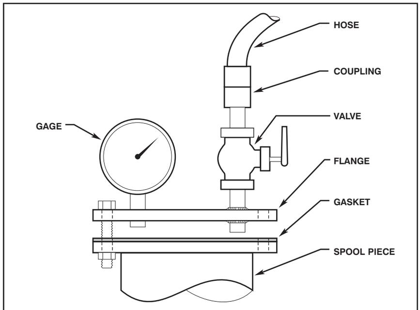
Figure 11-12. Blowing Fitting.
