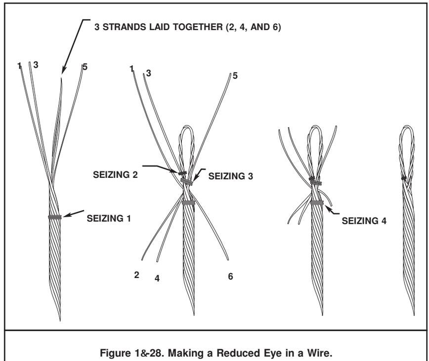
Figure 1&-28. Making a Reduced Eye in a Wire.
