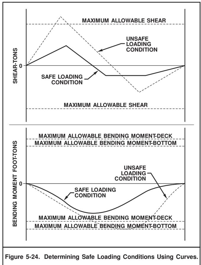
Figure 5-24. Determining Safe Loading Conditions Using Curves.
