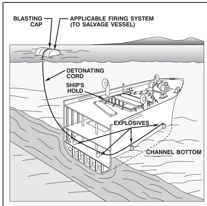
Figure 14-29. Charge Placement for Wreck Settling.
