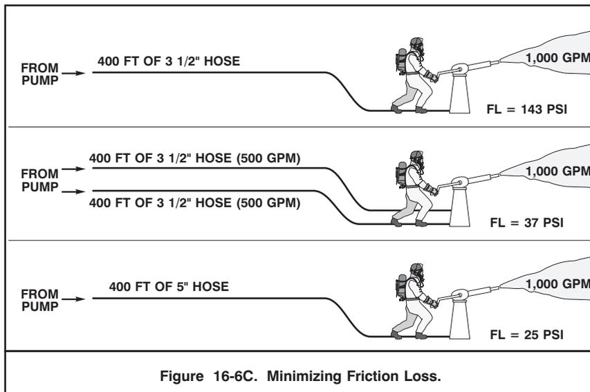
Figure 16-6C. Minimizing Friction Loss.
