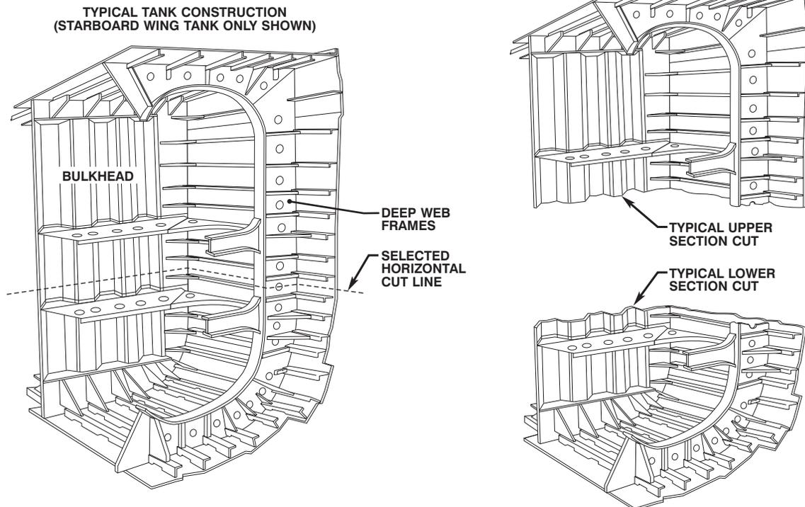
Figure 14-6. Transverse Cutting Plan for Midships Section.
