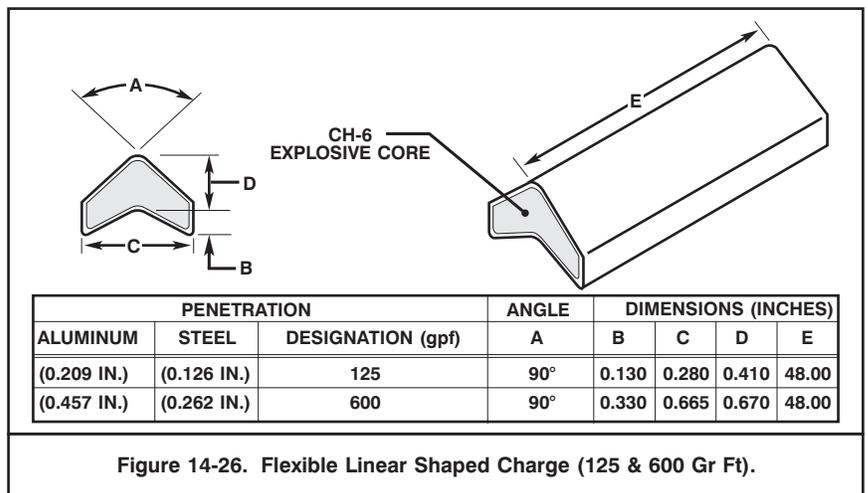
Figure 14-26. Flexible Linear Shaped Charge (125 & 600 Gr Ft).
