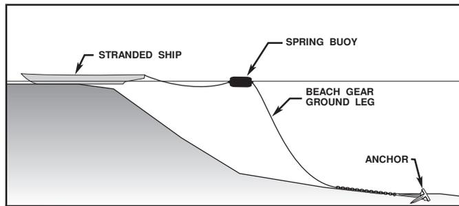
Figure 8-25. Spring Buoy Rigged into Ground Leg.
