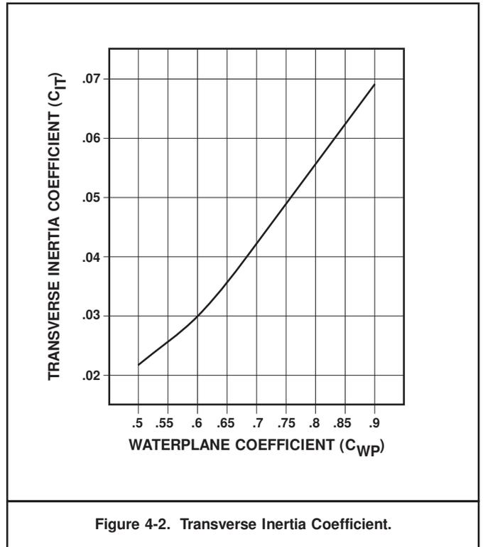
Figure 4-2. Transverse Inertia Coefficient.
