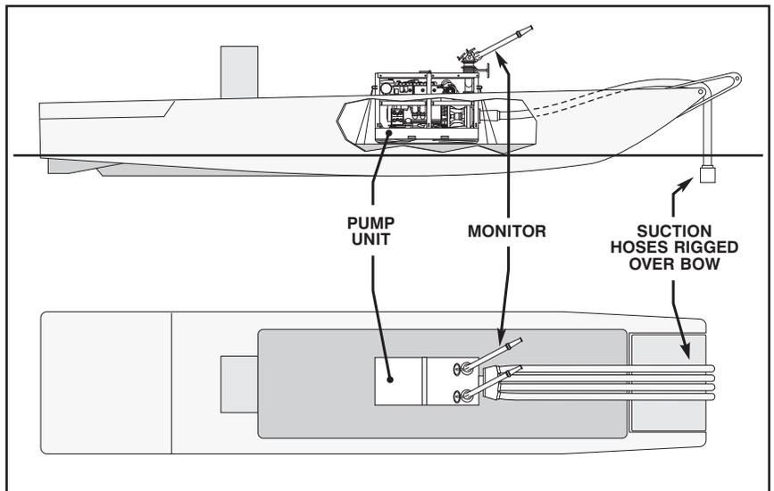
Figure 20-2. Typical Deployment of Portable Firefighting Pump Unit on Standard 35-Foot Salvage Work Boat.
