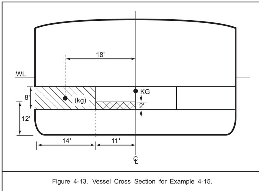
Figure 4-13. Vessel Cross Section for Example 4-15.
