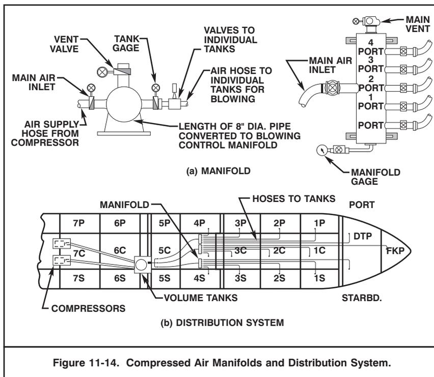
Figure 11-14. Compressed Air Manifolds and Distribution System.
