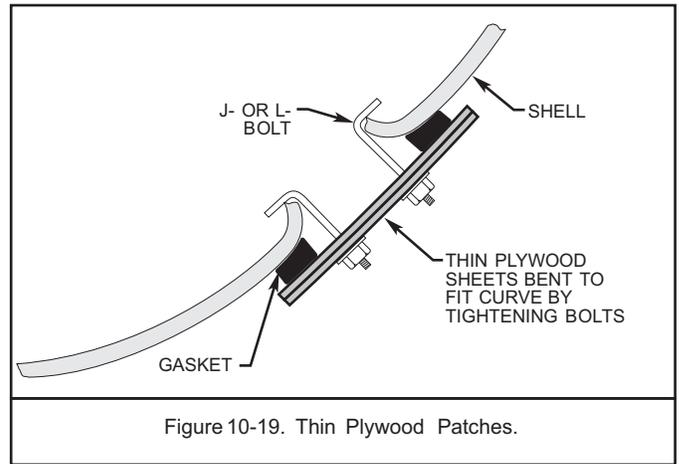
Figure 10-19. Thin Plywood Patches.
