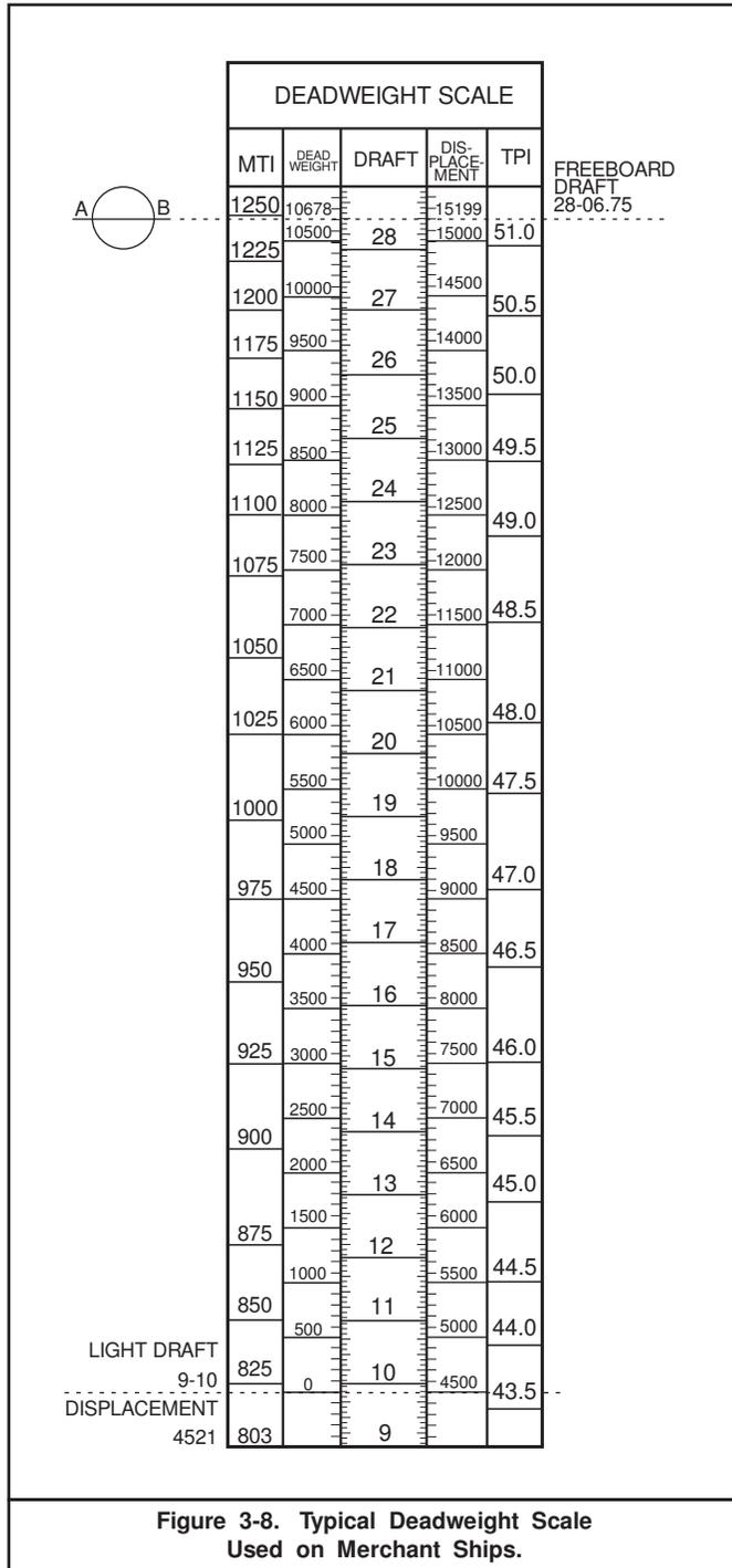
Figure 3-8. Typical Deadweight Scale Used on Merchant Ships.
