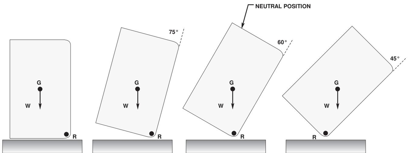
Figure 7-6. Movement of Center of Gravity and Effect of W as Ship is Rotated Upright.
