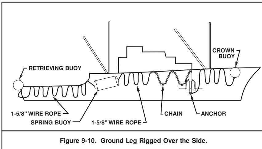
Figure 9-10. Ground Leg Rigged Over the Side.
