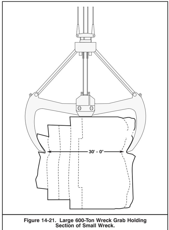
Figure 14-21. Large 600-Ton Wreck Grab Holding Section of Small Wreck.
