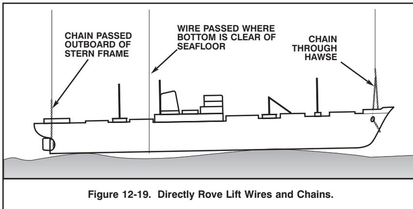
Figure 12-19. Directly Rove Lift Wires and Chains.
