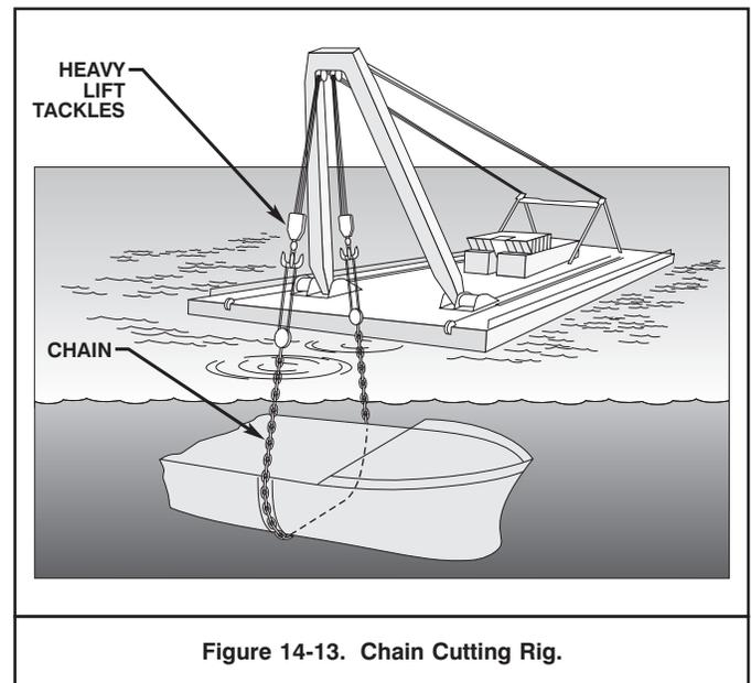
Figure 14-13. Chain Cutting Rig.
