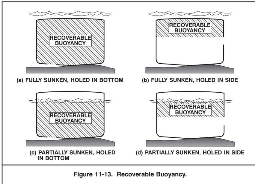
Figure 11-13. Recoverable Buoyancy.
