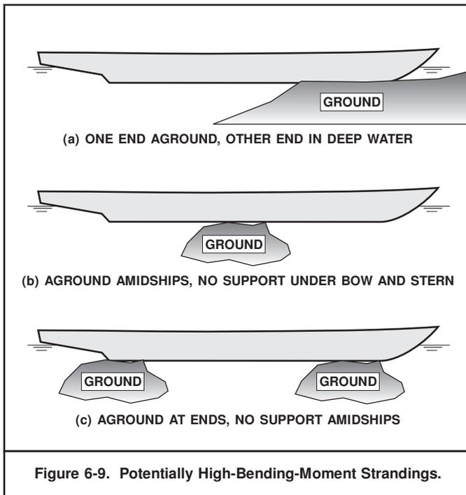
Figure 6-9. Potentially High-Bending-Moment Strandings.
