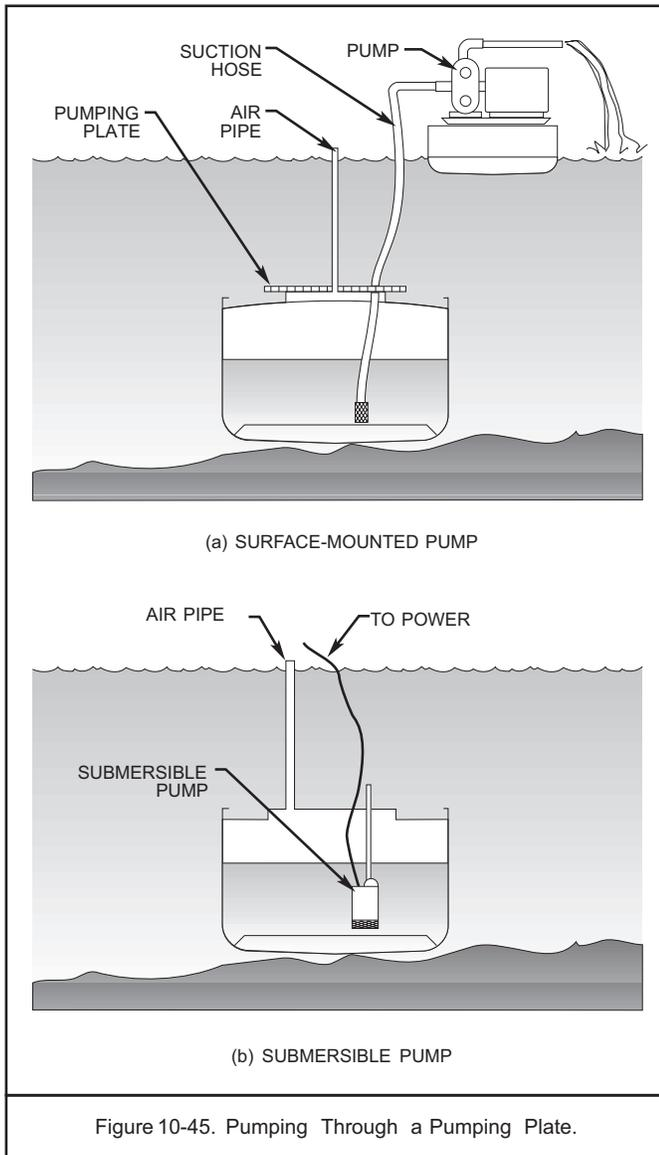
Construction of pumping plates for shallow water work is not a particularly difficult task. If the technique is applied in more than 6 feet of water, the deck and plate must be shored against the water pressure.
