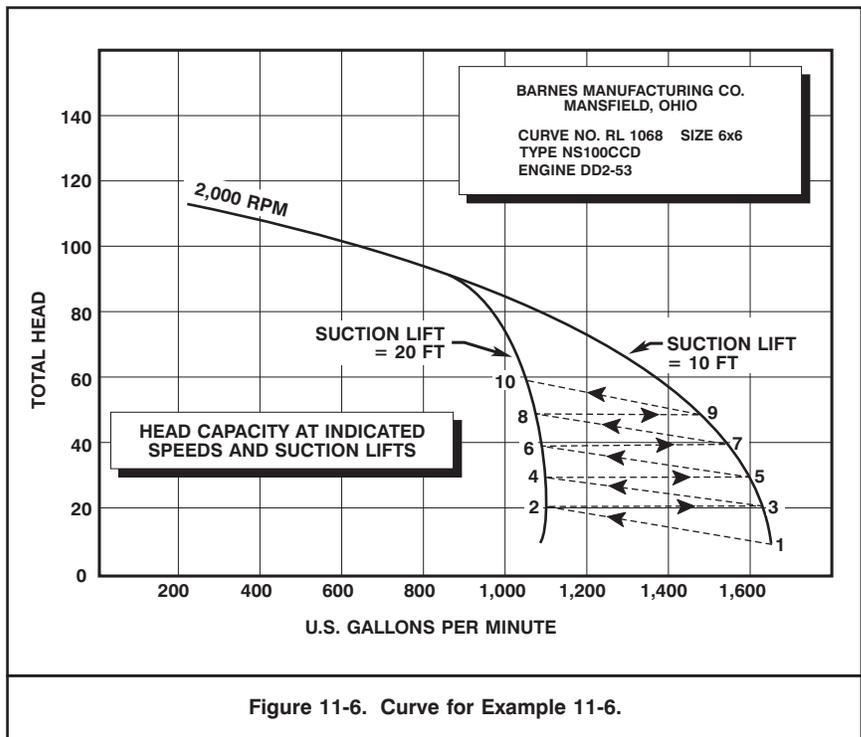
Figure 11-6. Curve for Example 11-6.
