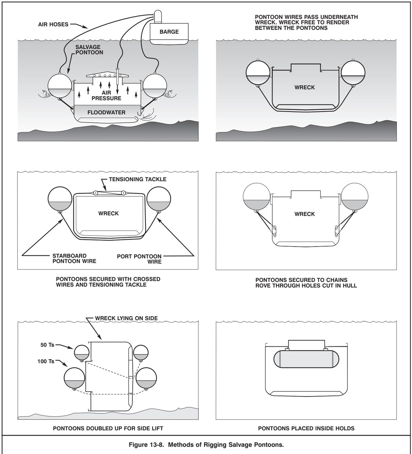
Figure 13-8. Methods of Rigging Salvage Pontoons.
