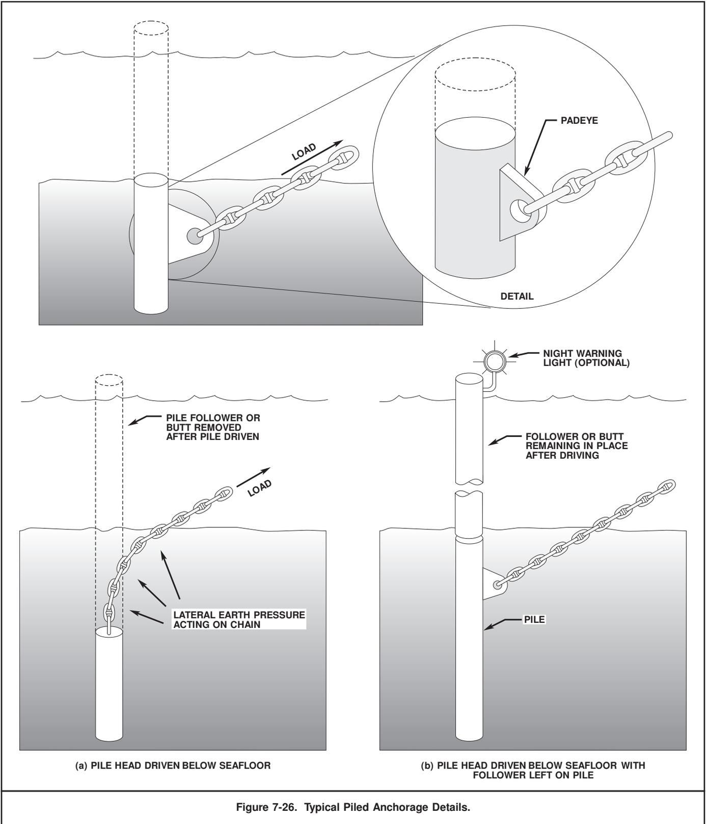
Figure 7-26. Typical Piled Anchorage Details.
