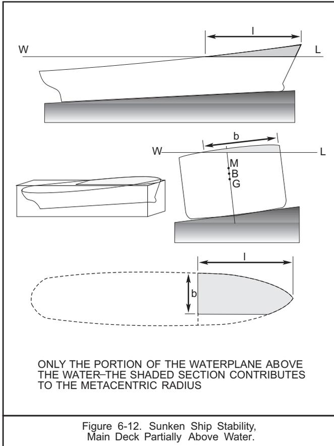
Figure 6-12. Sunken Ship Stability, Main Deck Partially Above Water.
