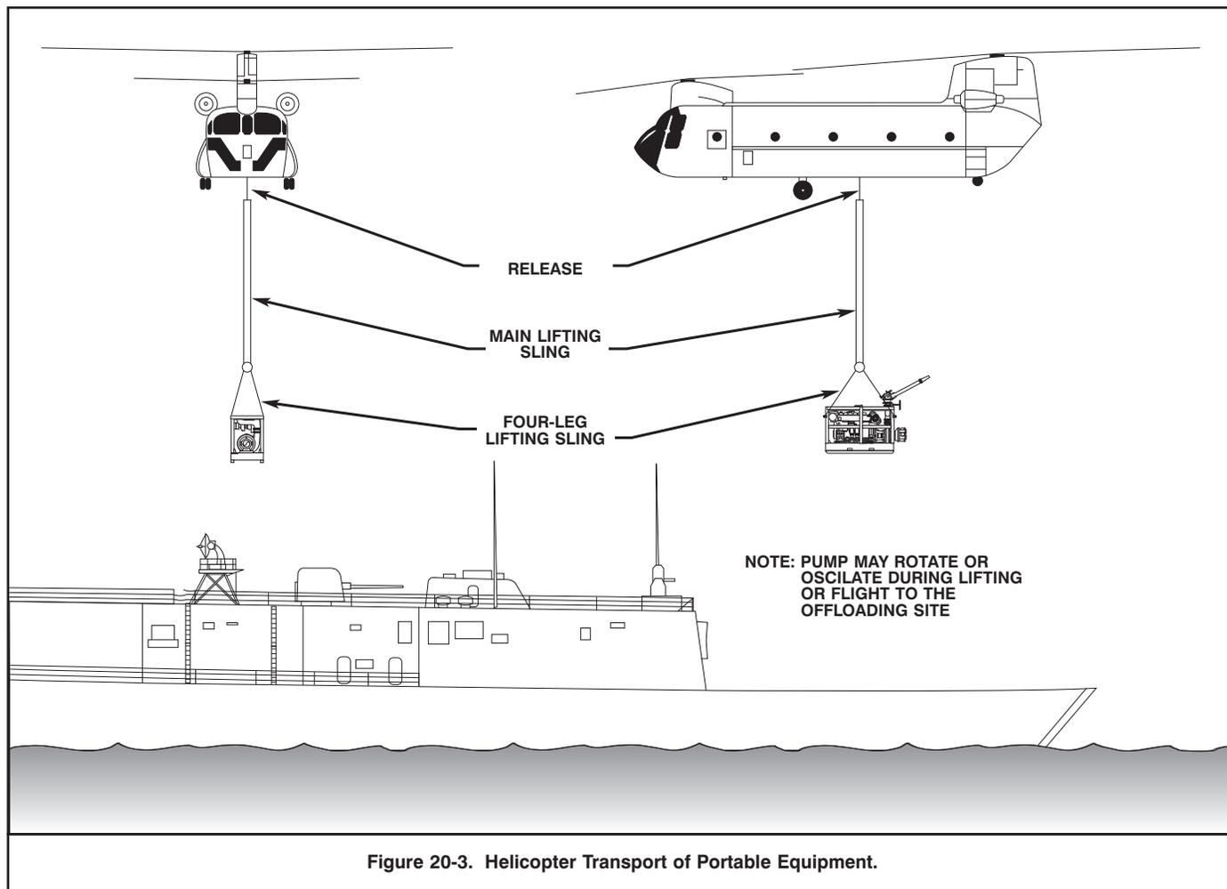
**20-2.2.4 Use of Helicopters.** The advantage to using helicopters in a salvage and firefighting scenario at sea is that helicopters are the fastest means of transporting salvage firefighting teams to a casualty. Circumstances permitting, helicopters can assist in rapid deployment of firefighting equipment and personnel to the casualty.
