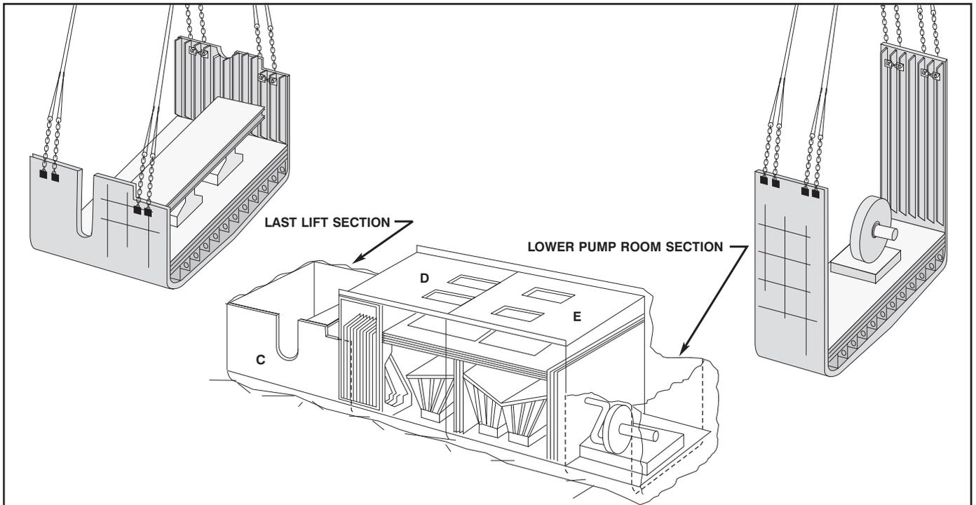
Figure 14-9. Wreck at Intermediate Stage of Demolition.
