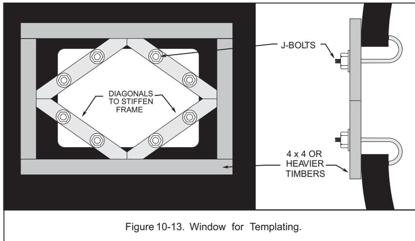
Figure 10-13. Window for Templating.
