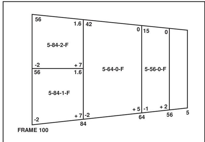
Figure 3-5. Sample Liquid-Loading Diagram Format.
