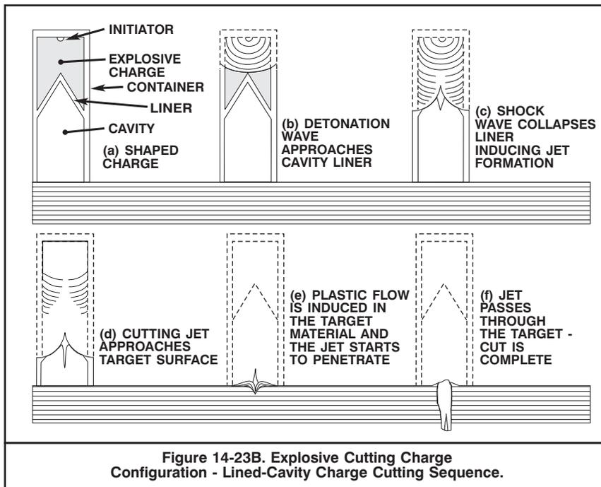
Figure 14-23B. Explosive Cutting Charge Configuration - Lined-Cavity Charge Cutting Sequence.
