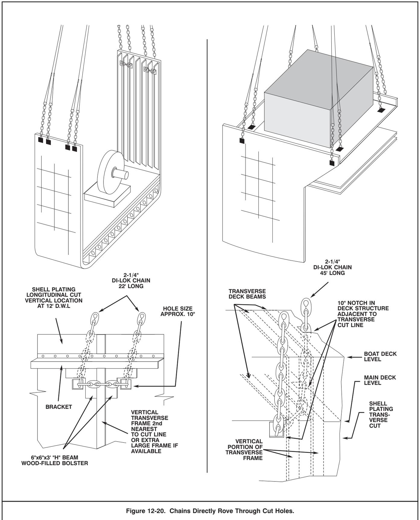
Figure 12-20. Chains Directly Rove Through Cut Holes.
