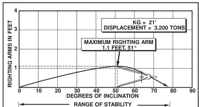
Figure 4-7. Corrected Statical Stability Curve.
