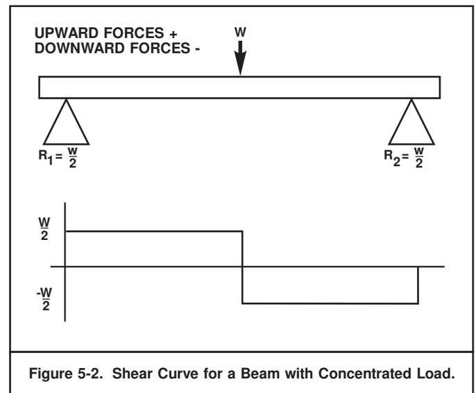
In the beam in Figure 5-2, the only force to the left of any point between  $R_1$  and  $W$  is the upward force (equal to  $+W/2$ ) at the support; shear force at this point is therefore  $+W/2$ . The shear force can be calculated at several points along the length of the beam and plotted on a graph as a shear curve. Shear is determined for points immediately to the right and left of concentrated loads and assumed to change abruptly at the point of loading.
