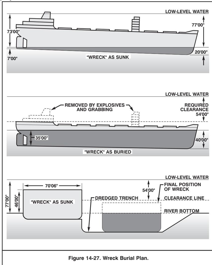
Figure 14-27 shows a profile of a sunken wreck as sunk and final position of the wreck after trenching and burial operations.
