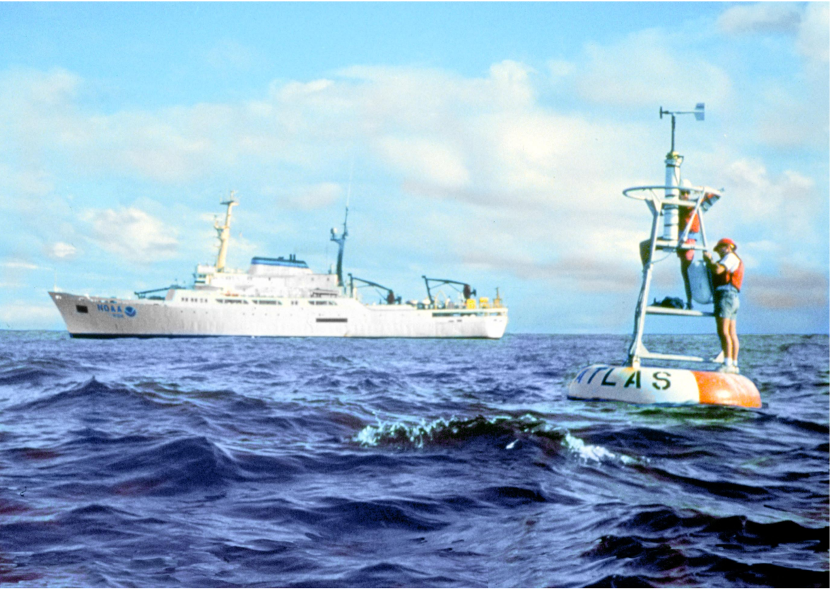
The NOAA ship Ka'imanoana supports oceanographic and climate research in the equatorial Pacific Ocean. The ship's primary mission is to deploy, recover, and service deep sea moorings that measure ocean currents, ocean temperatures, and atmospheric conditions throughout the equatorial regions of the Pacific Ocean. The Ka'imanoana supports a series of 70 buoys known as the Tropical Atmosphere-Ocean (TAO) array, which were first deployed as part of an international oceanographic research program to learn how to predict the El Niño/Southern Oscillation phenomenon. The buoys measure wind direction and speed, air temperature and humidity, and temperature of the ocean at the sea surface and at various depths to 500 meters. A few buoys also measure currents, rainfall and solar radiation. These buoys help scientists learn more how warm water of the equatorial Pacific affects world-wide climate, and are providing critical data about the El Niño event.
