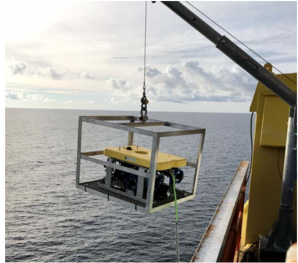
FIGURE 8: LAUNCHING OF ROV FROM PLATFORM DECK TO UNDERWATER USING DAVIT.
