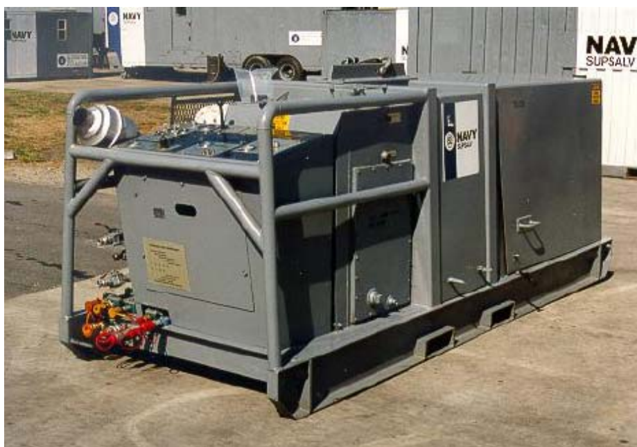
Hydraulic Power Unit PW0924
