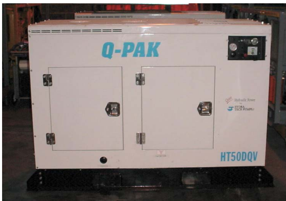
Hydraulic Power Unit PW0050
