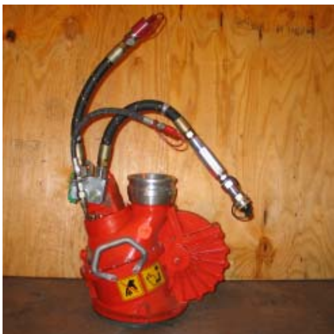
Heavy Oil Transfer Pump PU0851
