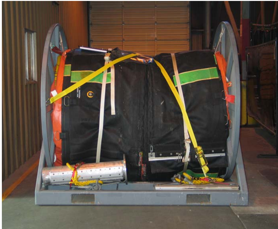
High Speed Current Buster Reel RL0051 (With NOFI Skimmer and USS-26 Boom)
