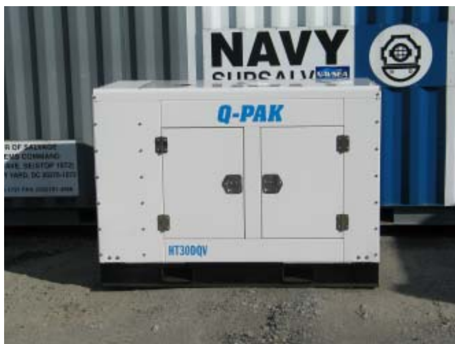
Hydraulic Power Unit PW0051
