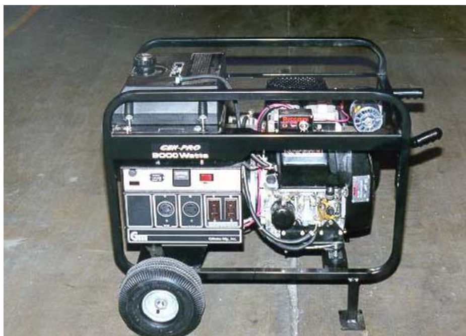
9-kW Generator GE0470
