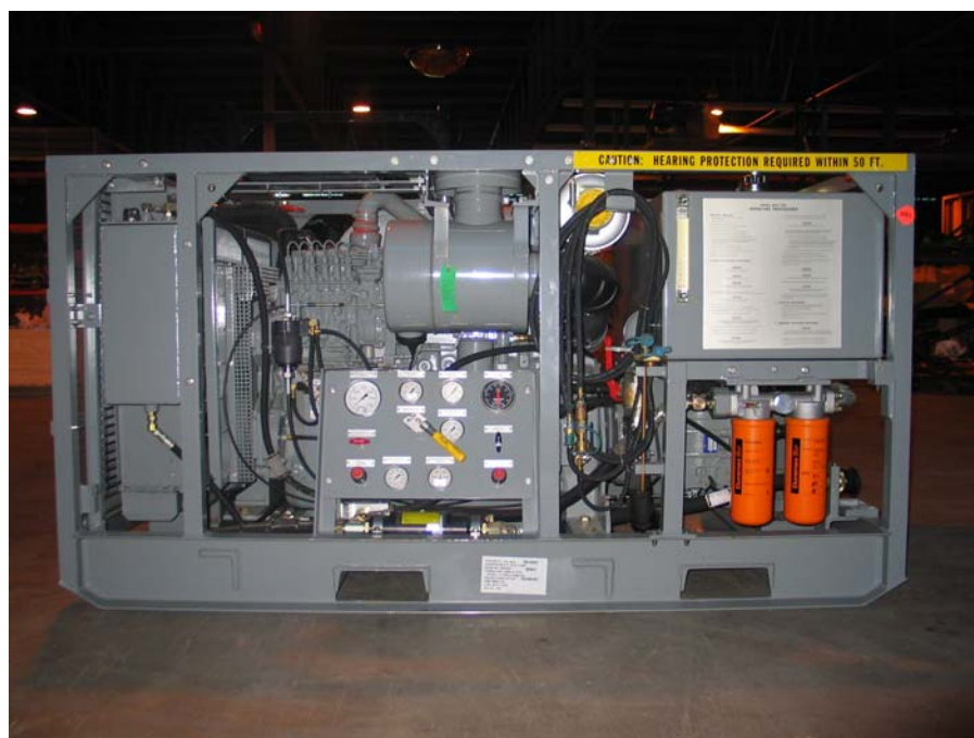
Mod 8 Hydraulic Power Unit PW0200B
