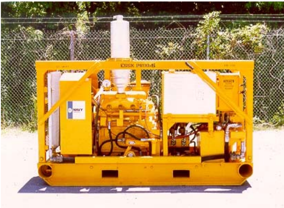
Mod 6 Hydraulic Power Unit PW0045
