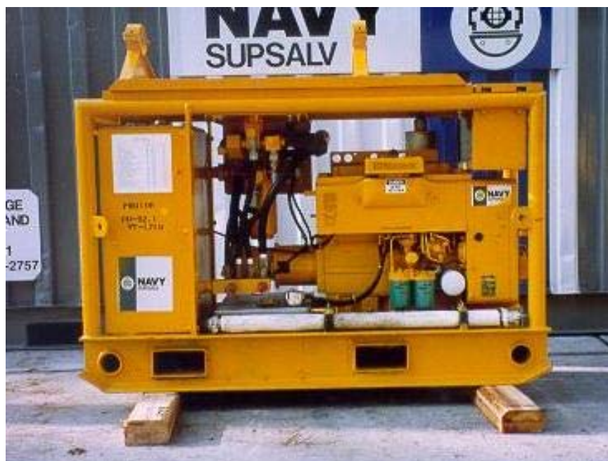
Mod 2 Hydraulic Power Unit PW0108
