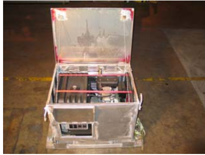
6.2-kW Diesel Generator GE0430
