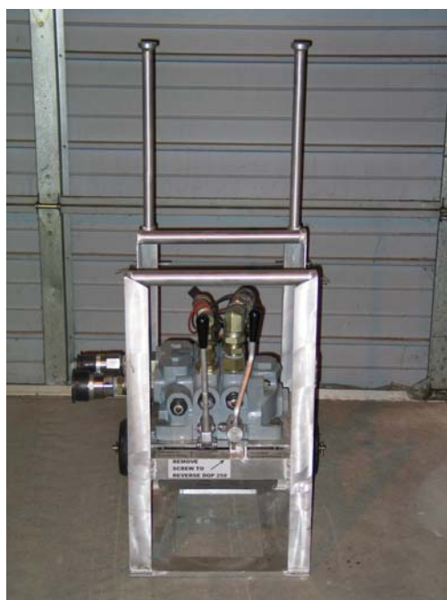
Control Block for the 6" Hydraulic Pump (PU0310) PU0311
