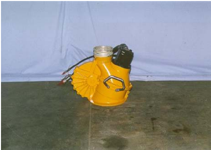
Heavy Oil Transfer Pump PU0851
