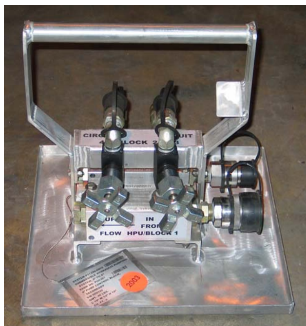
Secondary Control Block for 4" Hydraulic Pump (PU0305) PU0307
