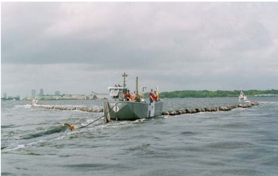
Vessel Skimmer System P16400 (Towboats not part of this system.)
