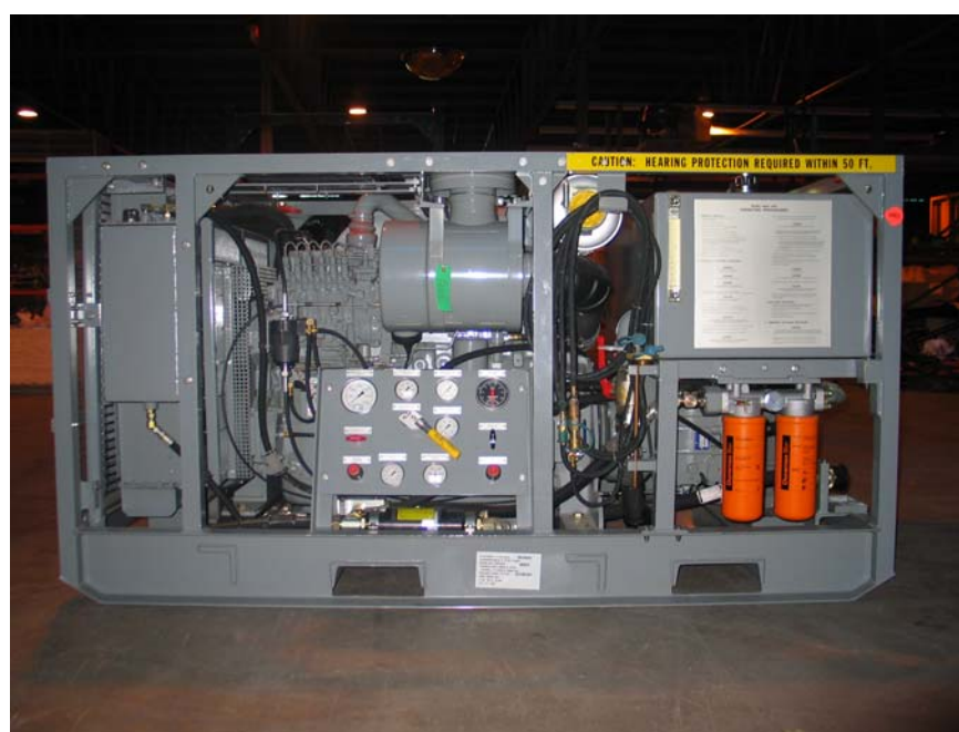
Mod 8 Hydraulic Power Unit PW0200B
