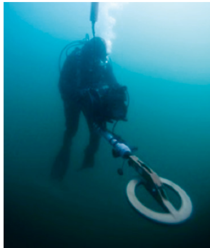
Figure 11 A scuba diver descending with a Shark Marine Navigator with integrated metal detector.
