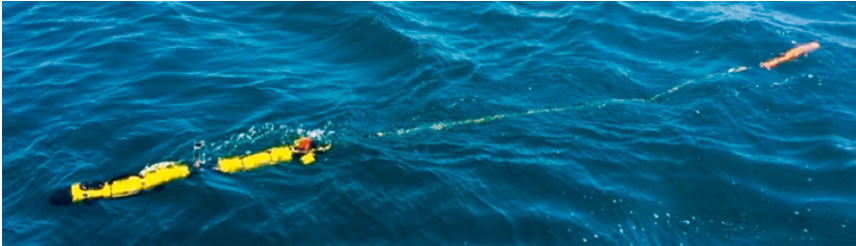
Figure 14 Marine Magnetics Explorer magnetometer towed behind an Iver3 AUV with SSS.
