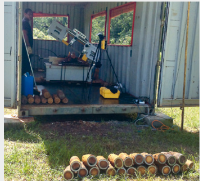
Figure 21 RSIPF using a mobile cutting system to cut ordnance before disposal in a burn pit.
