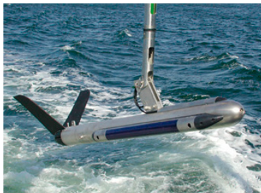
Figure 10 Deployment of a Klein 3000 side-scan sonar for a technical survey.
