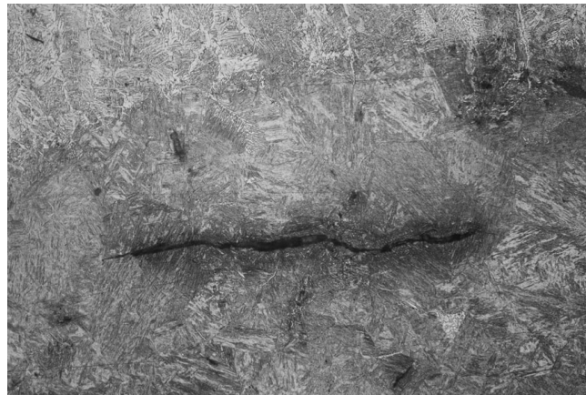
Fig. 6. Microphotograph of the cold crack in the bainite structure of heat affected zone [18]
