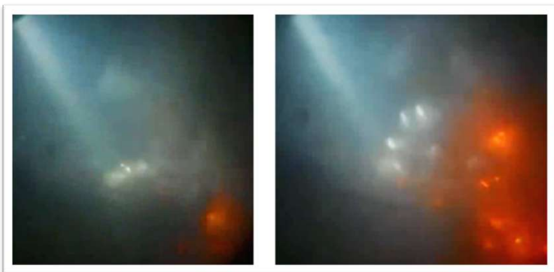
Fig. n° 48: Possible vapour explosion by accumulation of incandescent slag in front of a sheet pile slot (68).
