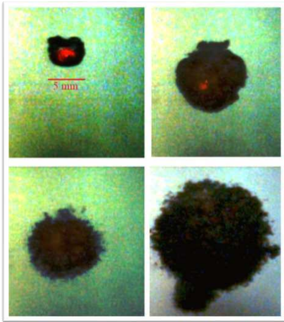
Fig. n° 45: Steam explosion of an incandescent ball (62).
