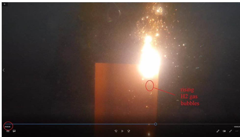
Fig 27: Rising H_2 ready to enter into contact with the flame
