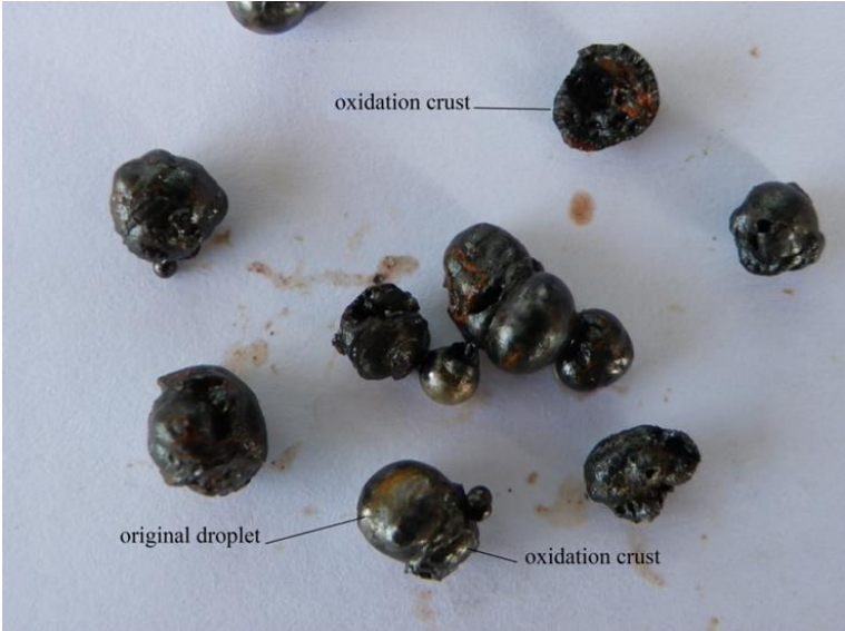
Fig 4: Final slag products
