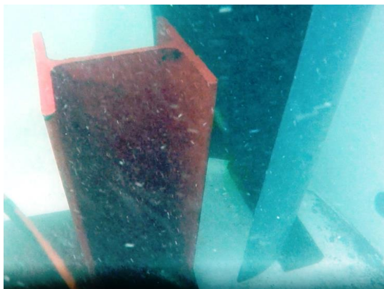
Fig 19: Installation of the metal piece into the gas recovery tube
