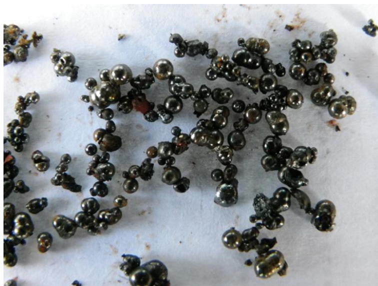
Fig 30: Residual slag droplets
