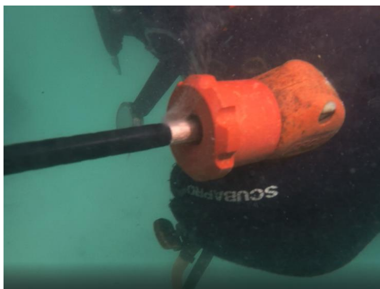
Fig 8: Electrolysis at the back of the rod
