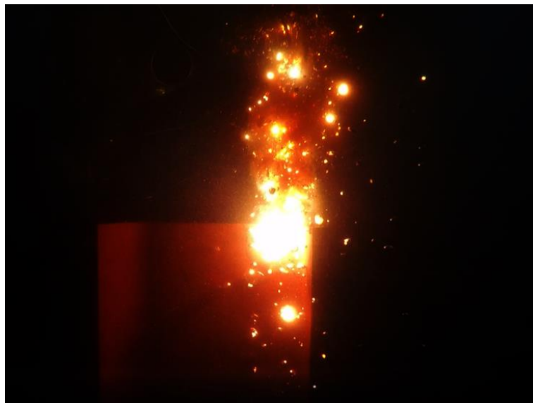
Fig 30: Residual slag droplets
