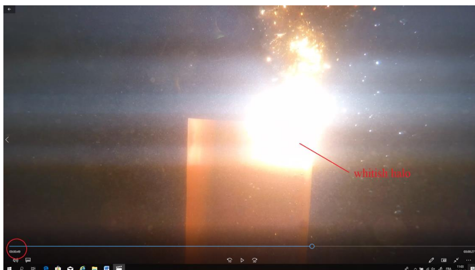
Fig 28: H_2 entering into contact with the flame
