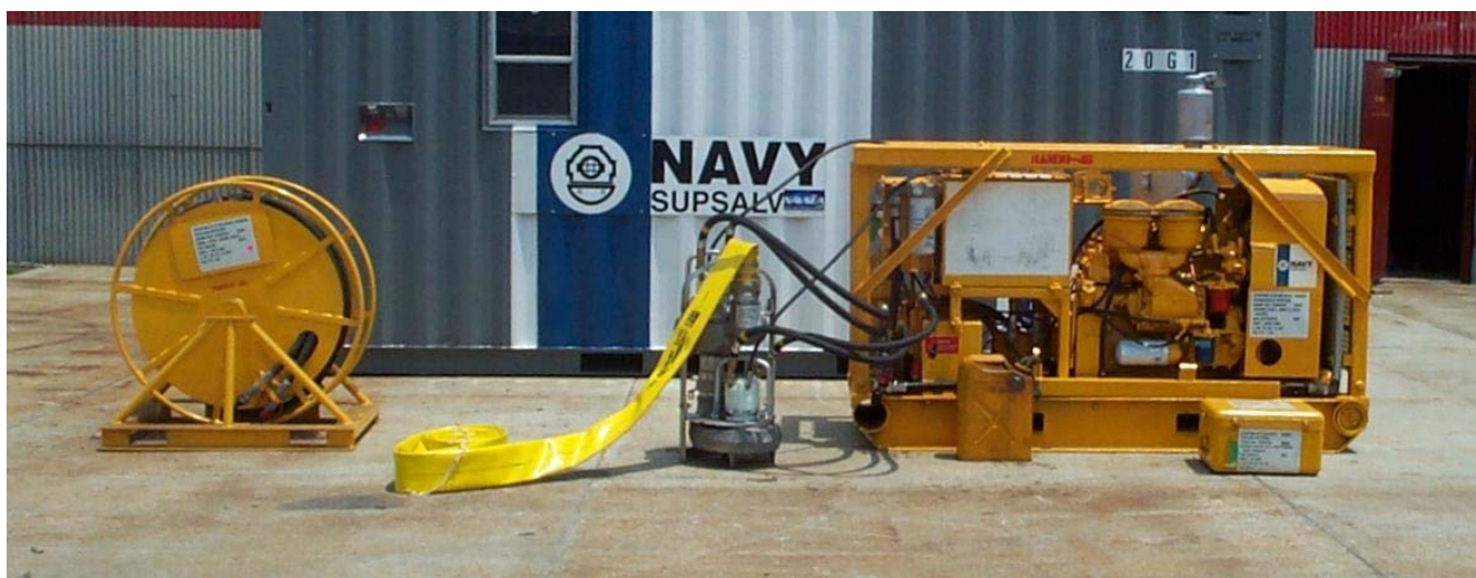
4-Inch Hydraulic Submersible Pumping System S18800 in Double Pump Configuration
