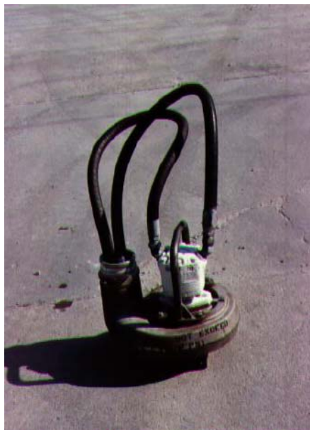
4" Hydraulic Submersible Pump in Single Pump Configuration
