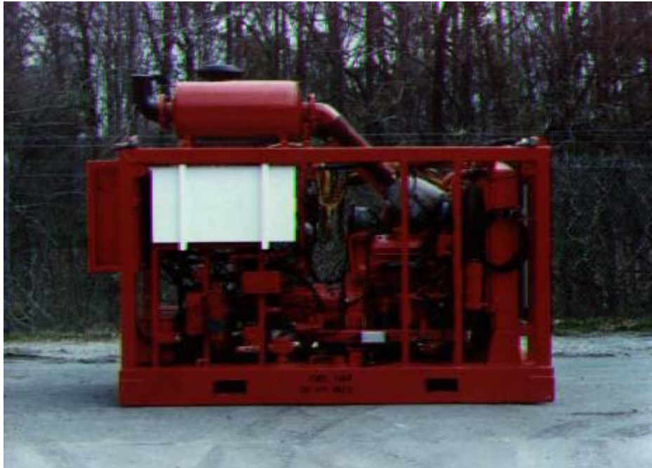
60-Kip FADOSS Hydraulic Power Unit (HPU) TU0220
