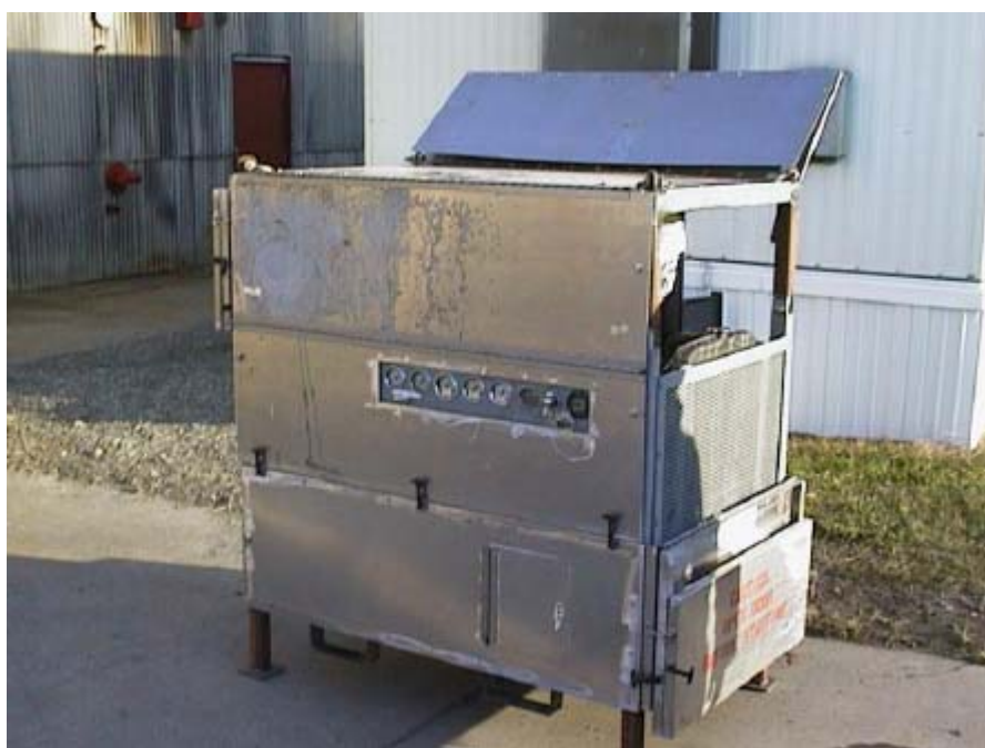
15-Cfm Diesel Air Compressor AC0600
