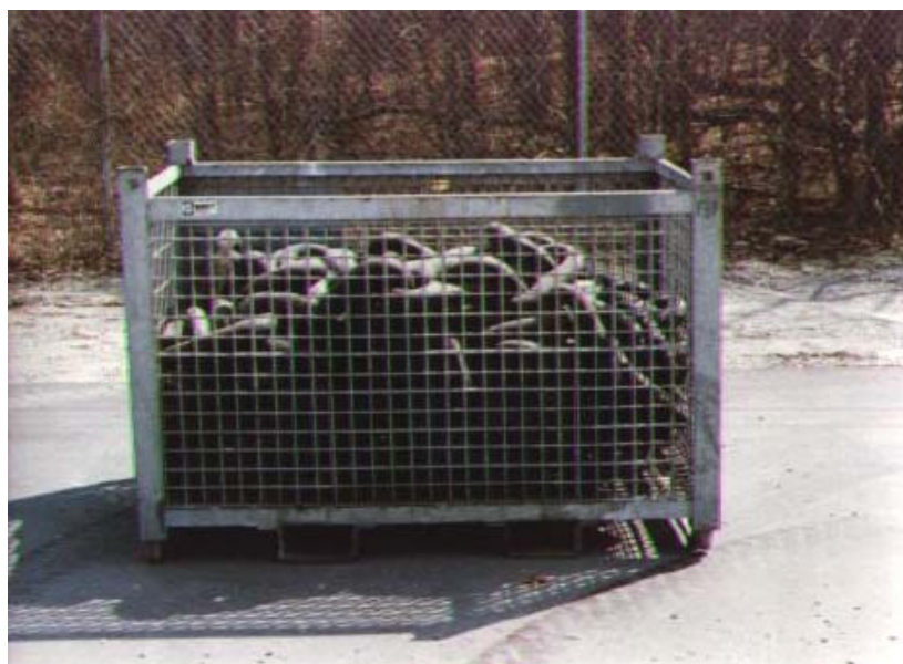
2 1/4-Inch x 90-Foot Stud Link Chain CH 2017 and Shipping Container
