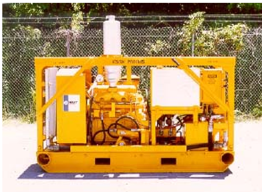
Mod 6 Hydraulic Power Unit PW0045
