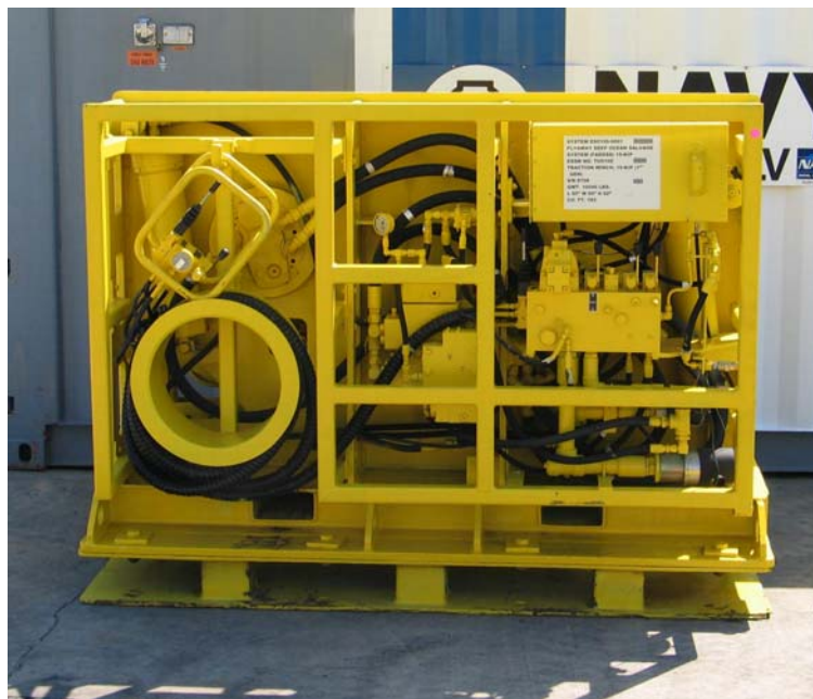
15-Kip FADOSS Traction Winch TU0100
