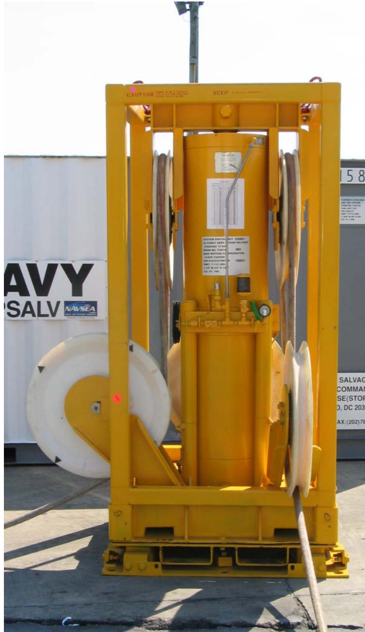
15-Kip FADOSS Ship Motion Compensator TU0121
