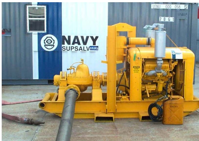
Overview of 2 1/2-Inch Jetting Pump System Using PU0229
