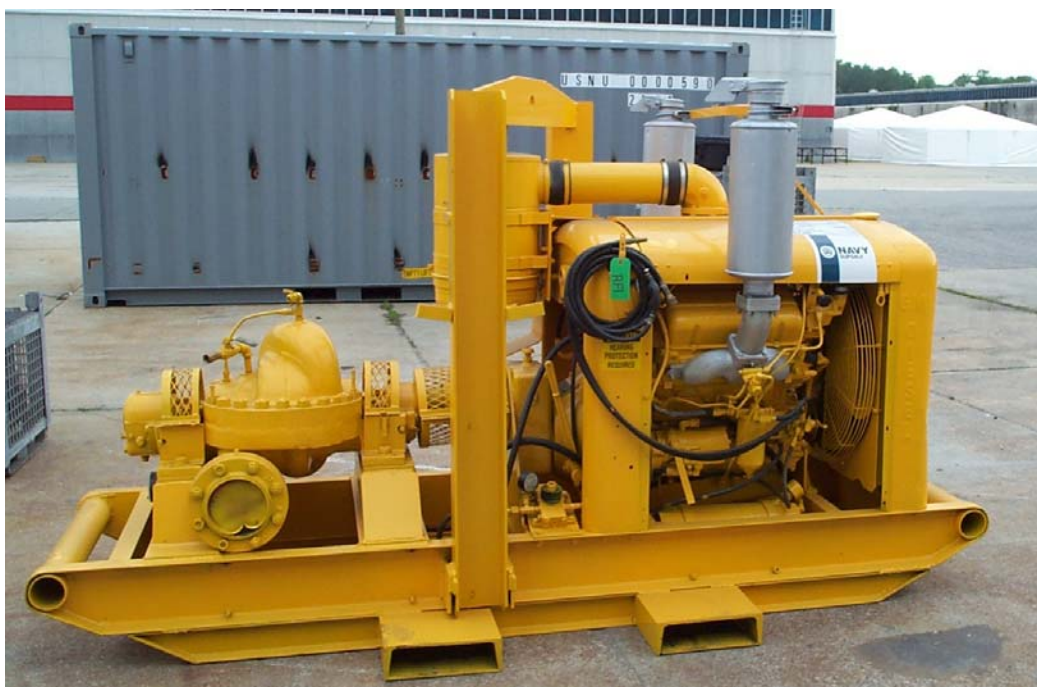
500-Gpm @ 150-Psi Jetting Pump (1st Generation) PU0230
