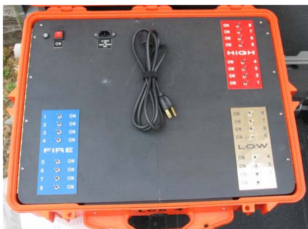
Local Control Station Operator's Panel
