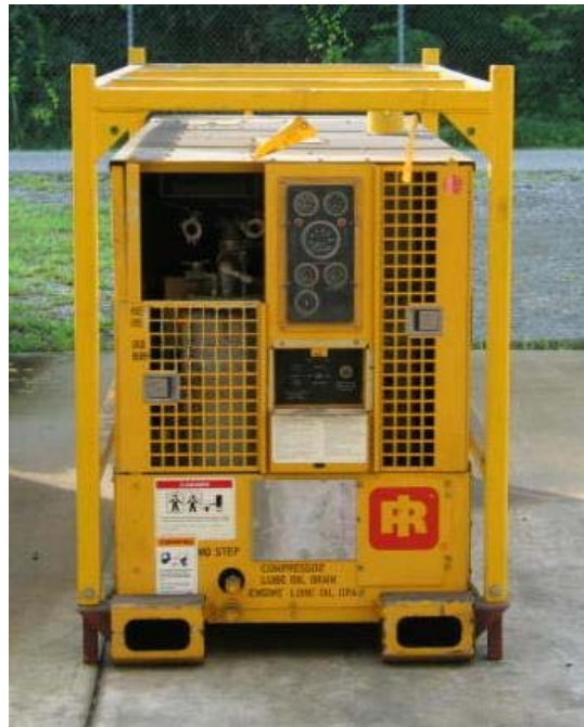
175-Cfm Air Compressor Controls and Gauges
