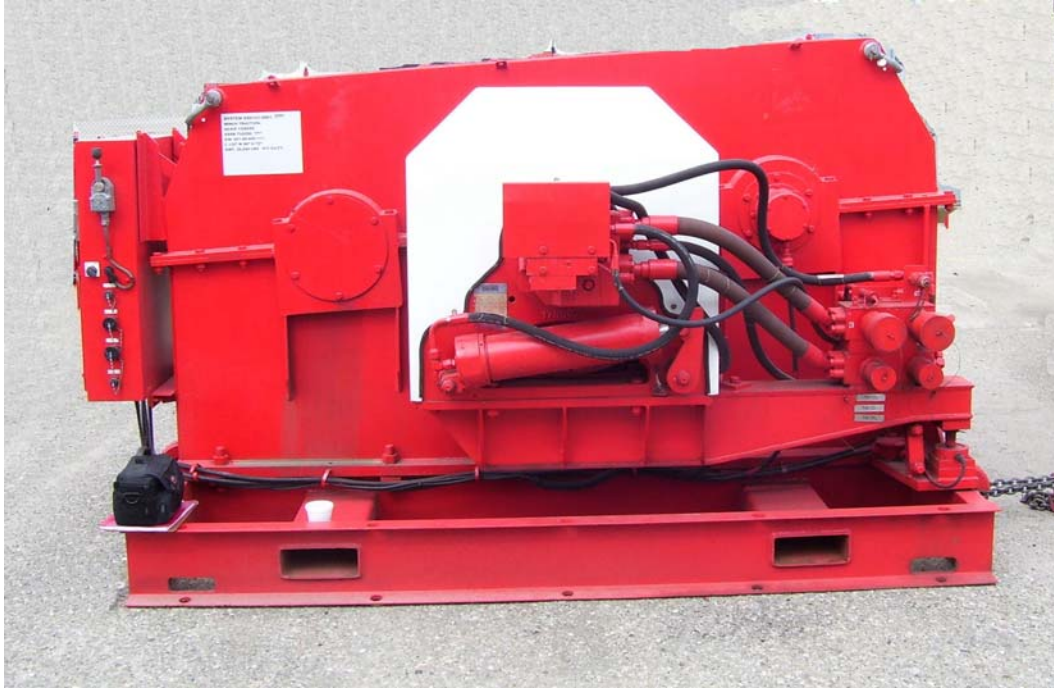
60-Kip FADOSS Traction Winch Hydraulic Motors
