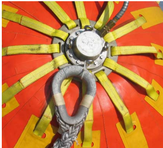
Rope-Lifting Pendant Showing Cable Tie Attachment
