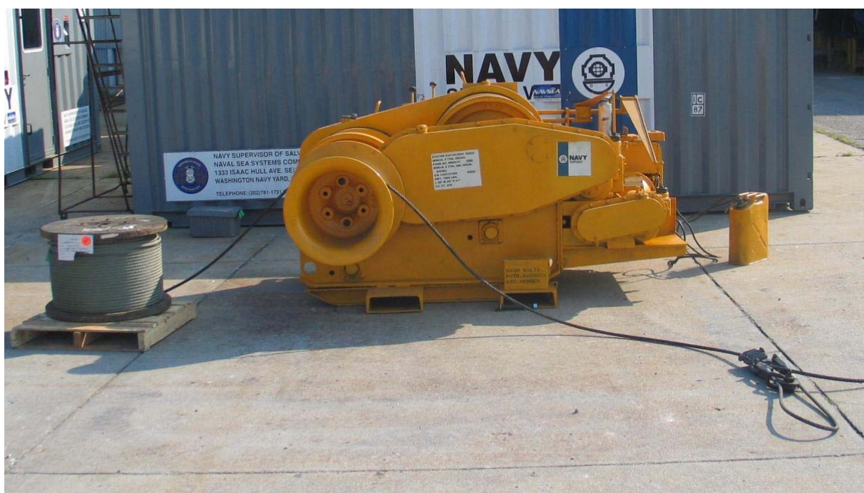
8-Ton Diesel Winch System S30100
