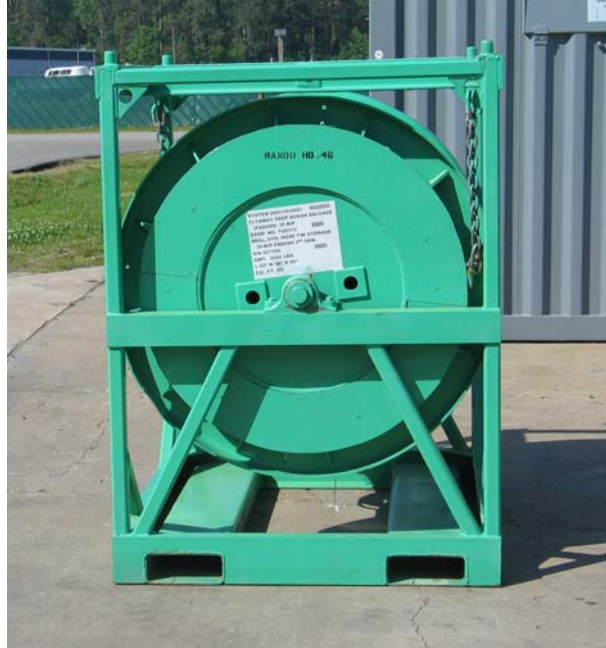
30-Kip FADOSS Traction Winch Hydraulic Hose Reel Assembly TU0312
