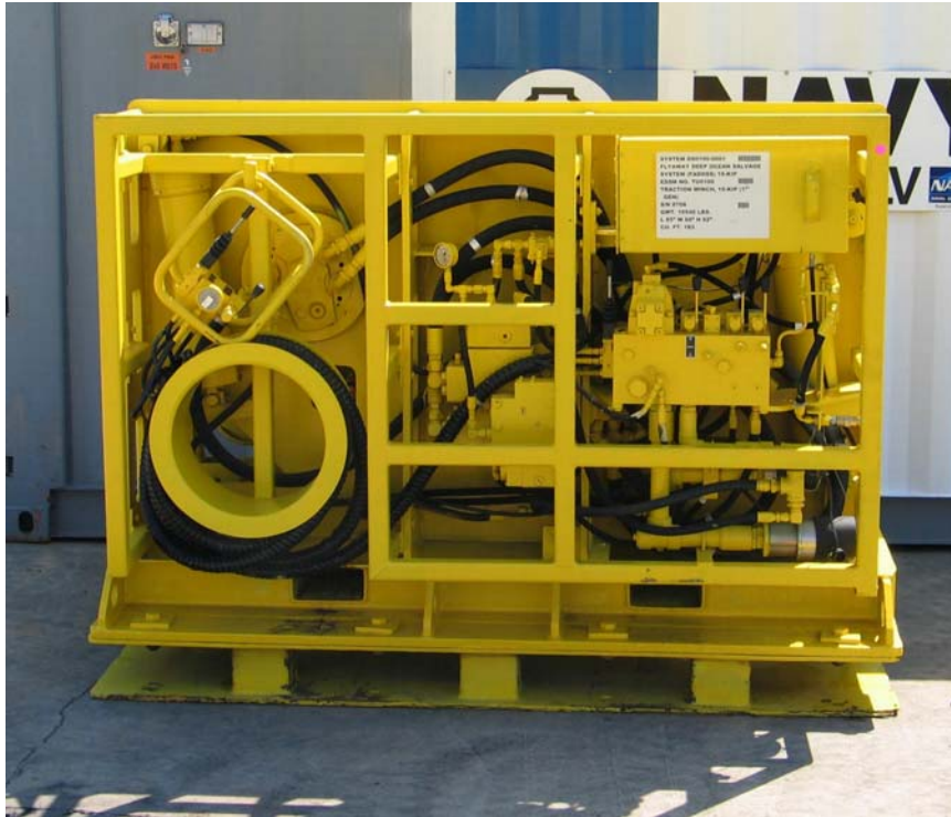
15-Kip FADOSS Traction Winch (2nd Generation) TU0120
