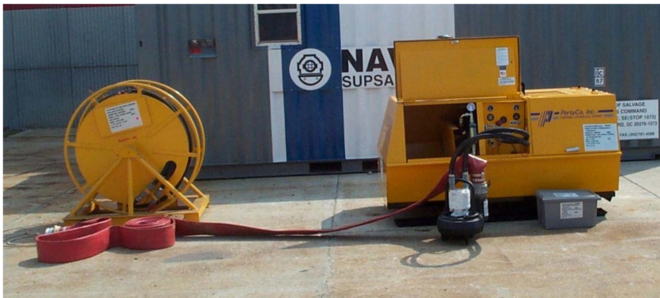
4-Inch Hydraulic Submersible Pumping System S18800 in Single Pump Configuration
