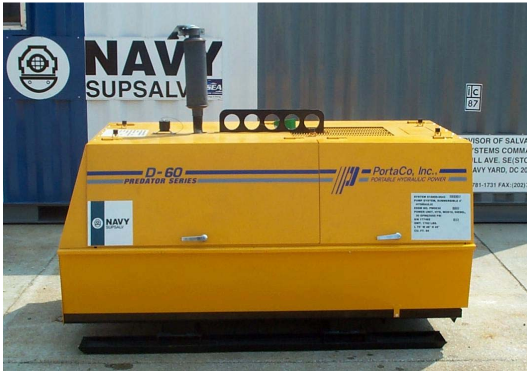
Mod 10 Hydraulic Power Unit PW0030
