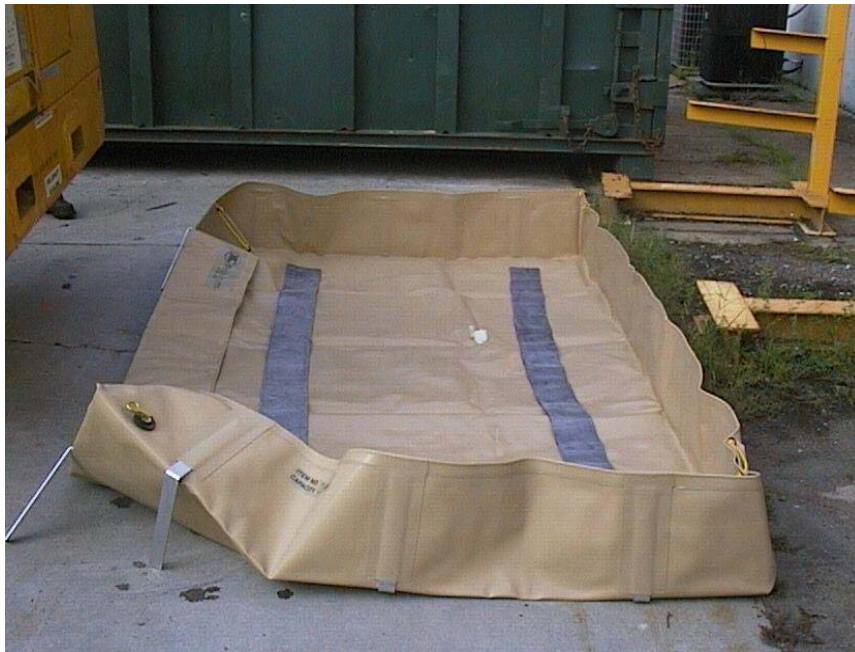
Machinery Containment Pool CP3020 (In-Use Configuration)
