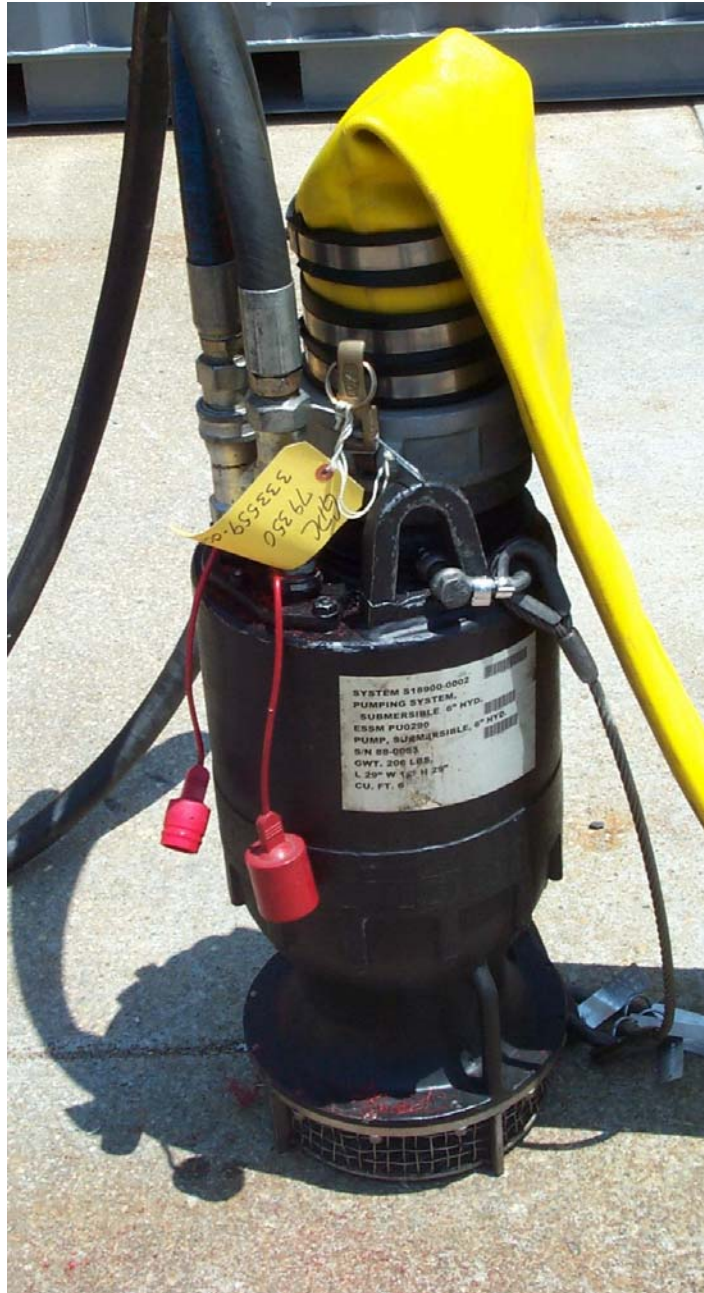
6" Hydraulic Submersible Pump PU0290
