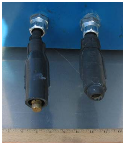
Switchbox Connectors Showing Standard Series Male and Female Cable Connectors
