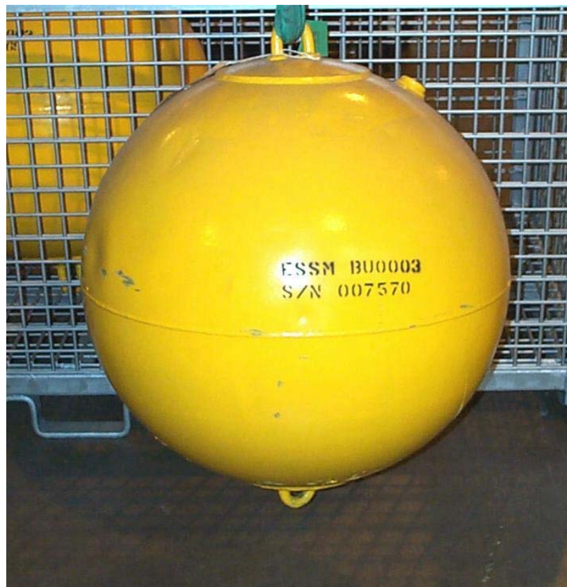
42-Inch Diameter Crown Buoy BU0003
