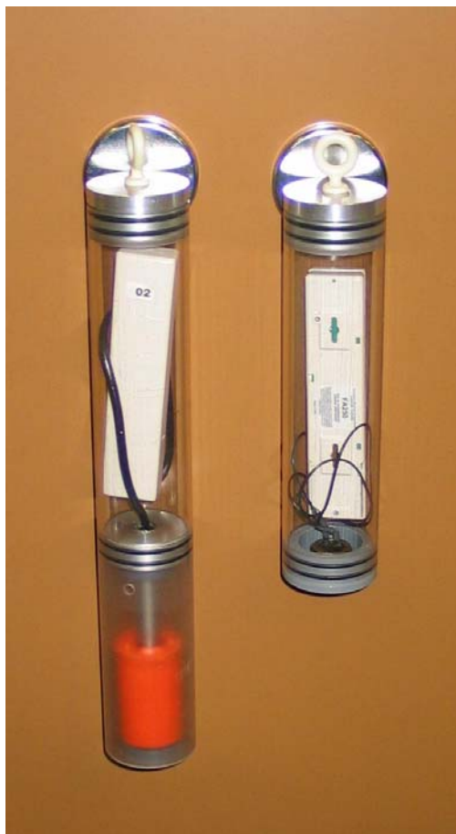
Wireless Tow Alarm System Flooding and Heat Sensors
