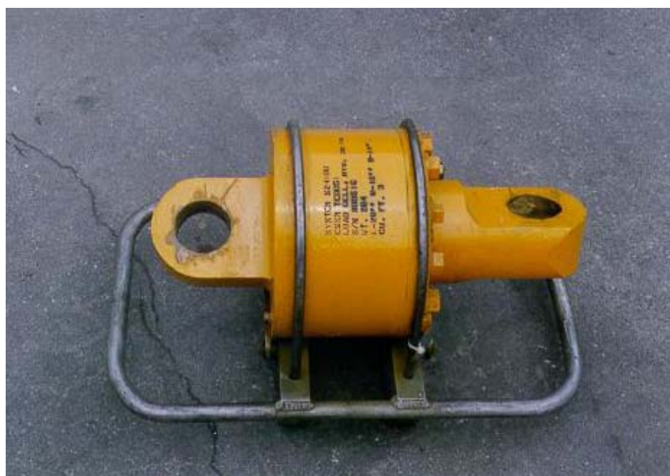
50-Ton Hydraulic Load Cell TE0051
