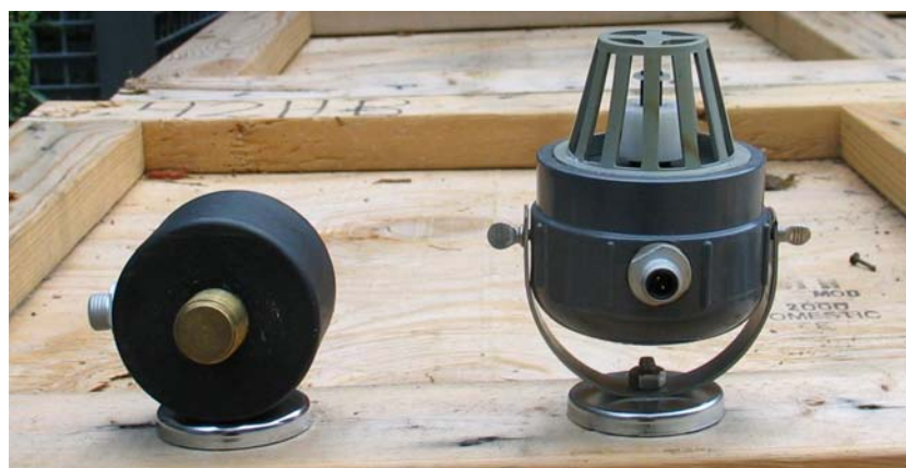
Heat and Water Level Sensors
