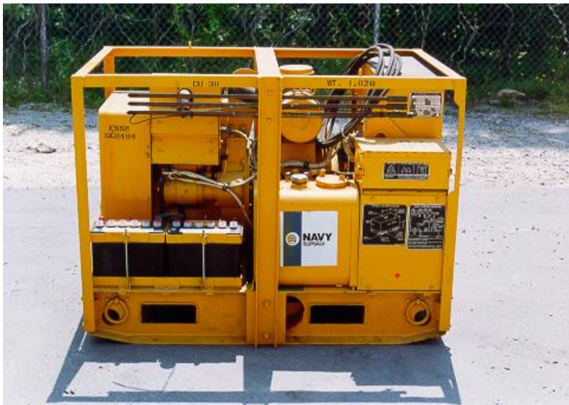
5-kW Diesel Generator GE0404
