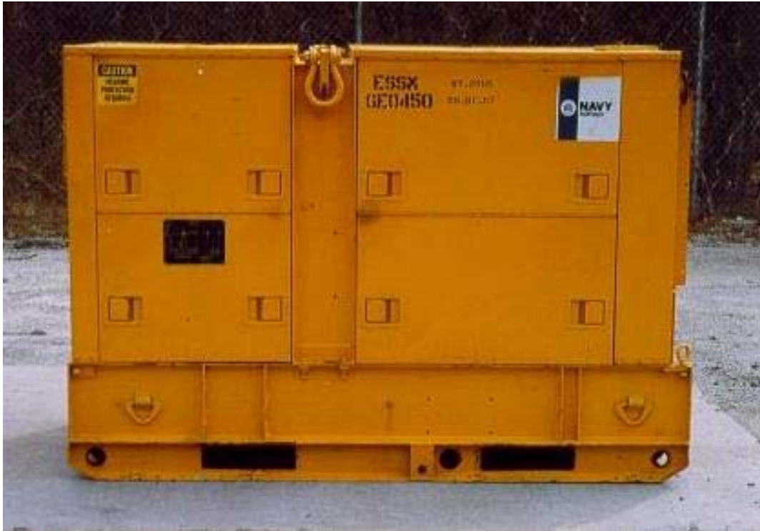
30-Kw Diesel Generator GE0450
