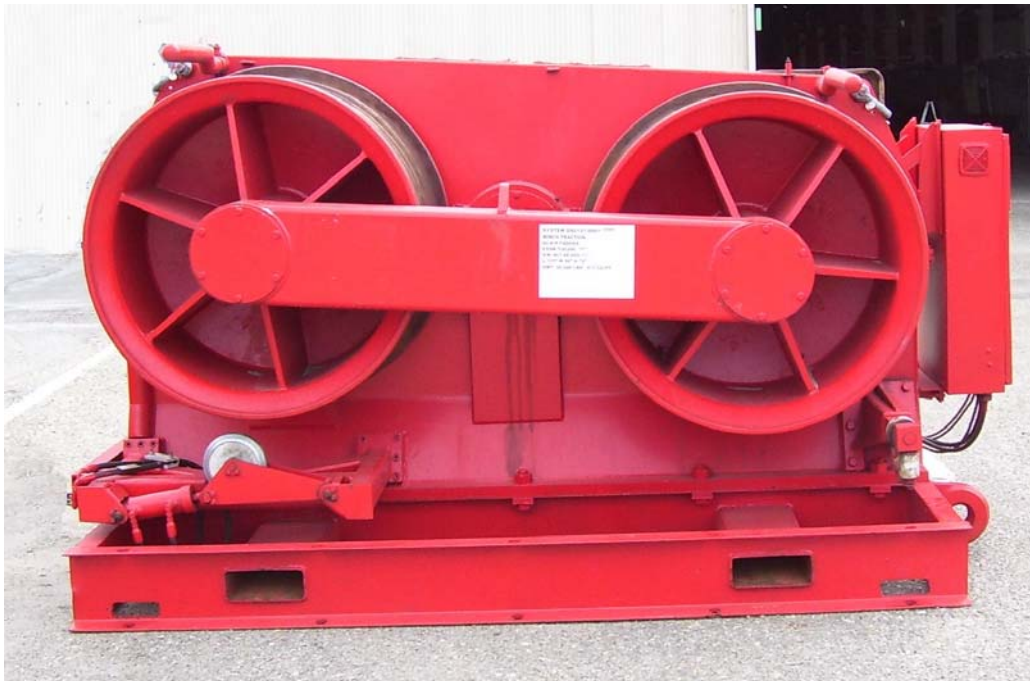
60-Kip FADOSS Traction Winch Drums
