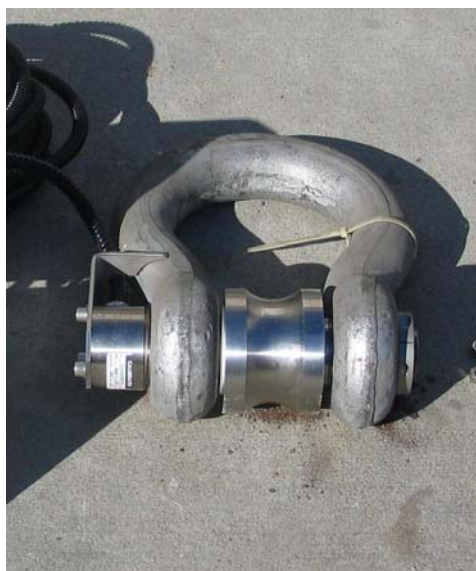
2 1/2-Inch Shackle with Clevis Pin Tension Link Installed
