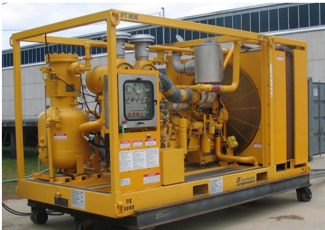
Submarine Salvage Air Compressor AC0245
