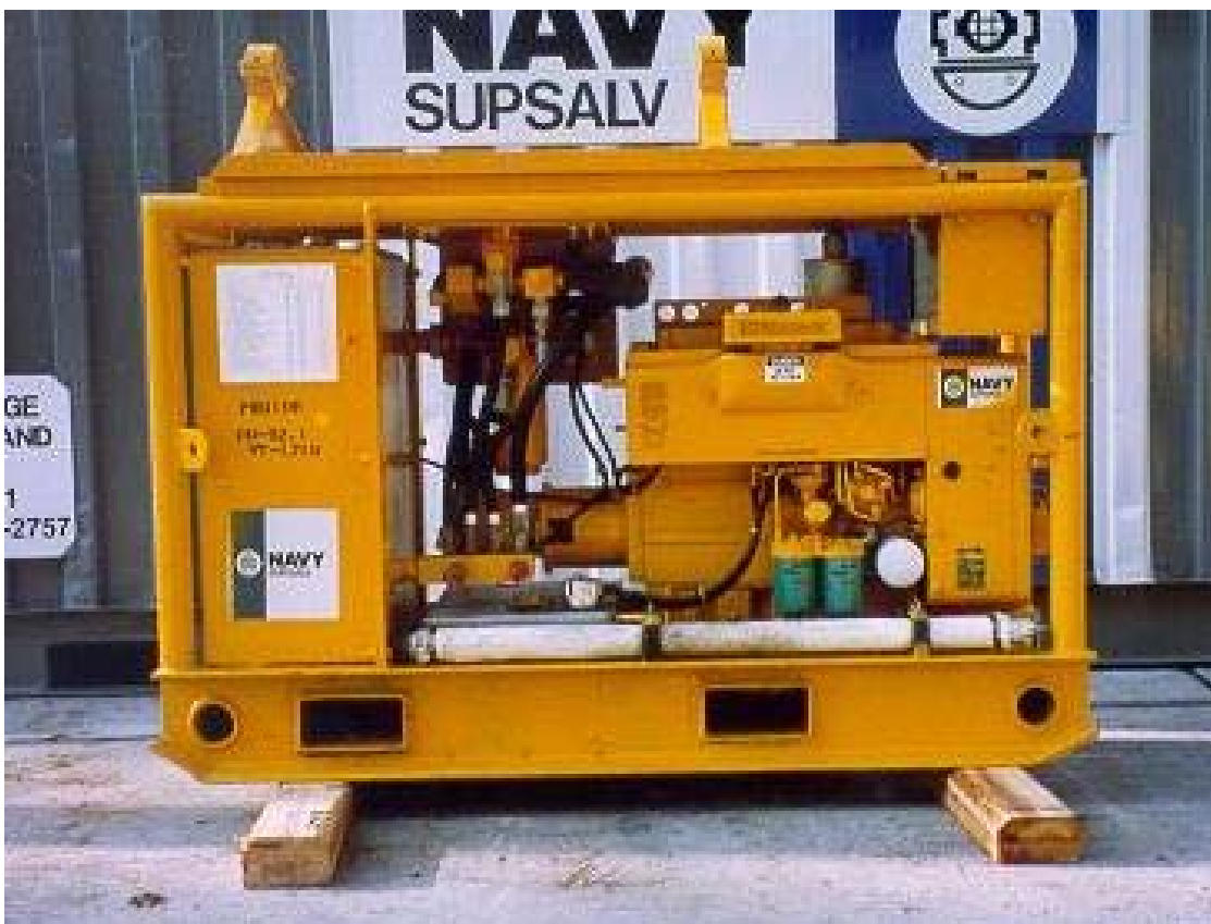
Mod 2 Hydraulic Power Unit PW0108
