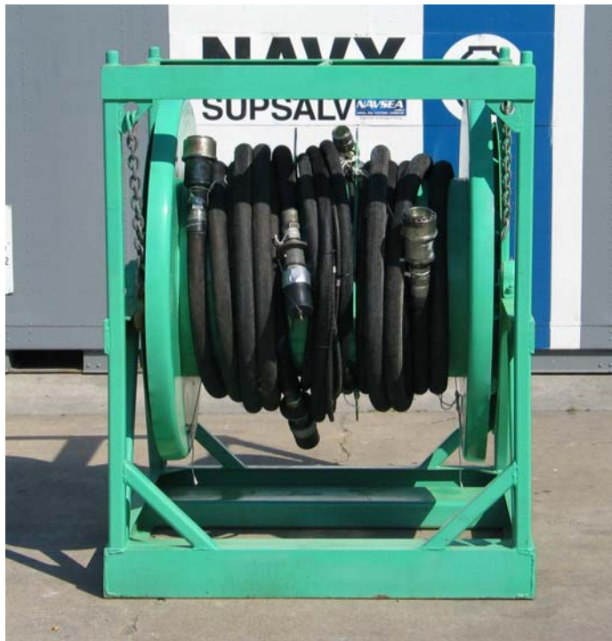
30-Kip FADOSS Traction Winch Hydraulic Hose Reel Assembly TU0311
