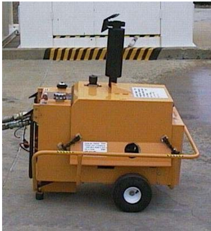
Mod 9 Hydraulic Power Unit Right Side View
