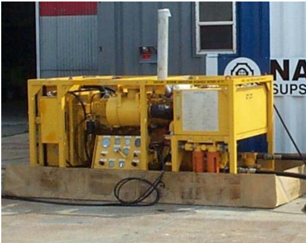
Mod 8 Hydraulic Power Unit PW0200A
