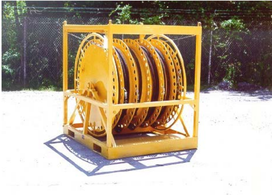
15-Kip FADOSS Take-up/Storage Reel Hydraulic Hose Reel Assembly TU0126
