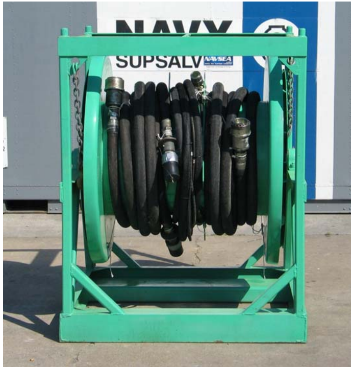
30-Kip FADOSS Traction Winch Hydraulic Hose Reel Assembly TU0312
