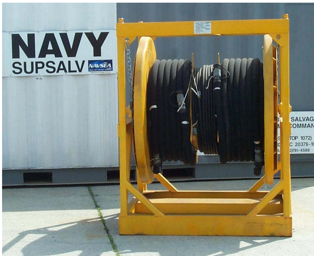
Hose Reel Assembly PW0201
