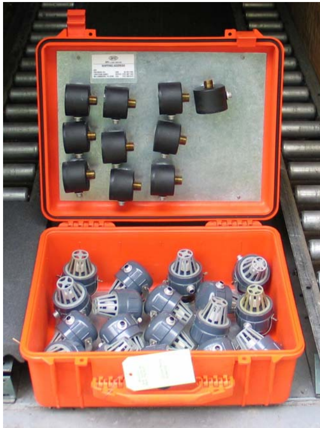
Flooding and Heat Sensors AL0023
