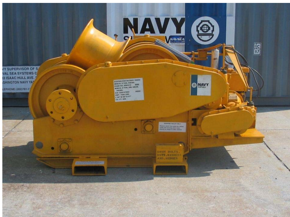
8-Ton Double Drum Diesel Winch WN0010
