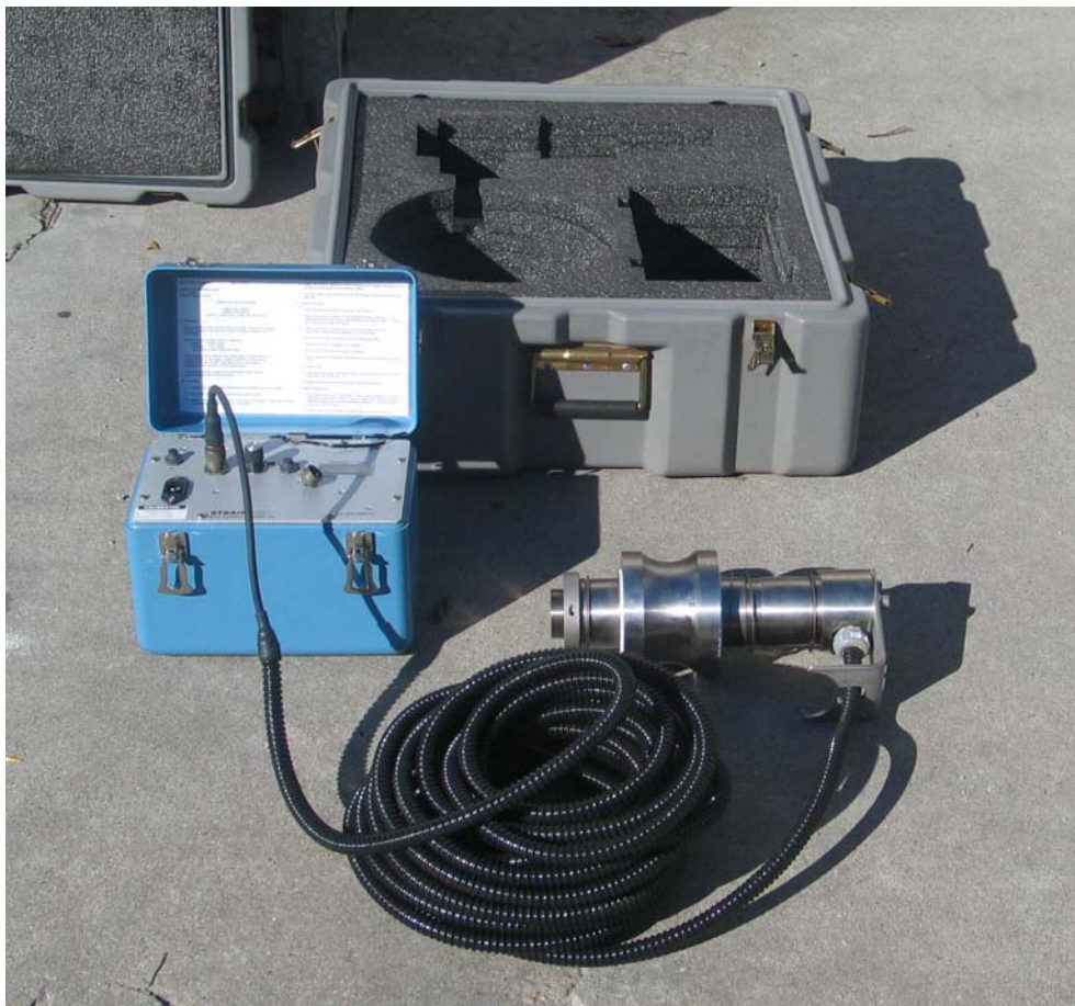
160K Load Sensing Clevis Pin Tension Link TE0056
