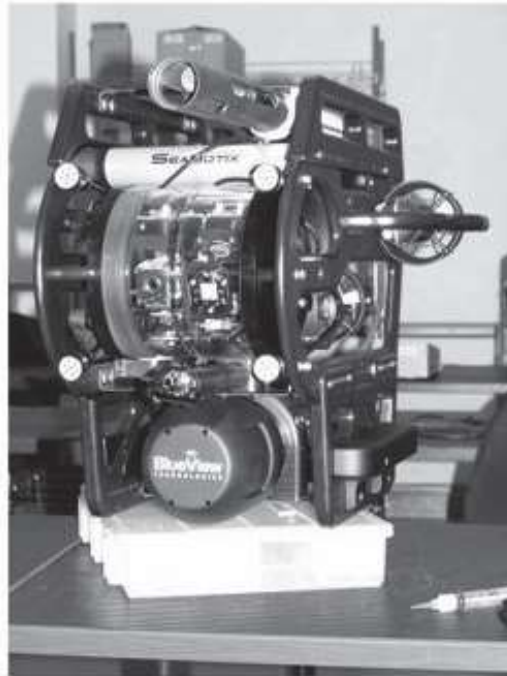
Figure 1. The ROV Shearwater , a Seabotix (San Diego) LBVs 6 remotely operated vehicle fitted with a Blueview (Seattle, WA) P900-130 2-D sonar on the lower tool skid and a Hach Hydromet (Loveland, CO) MS5 water quality sonde on the top tool skid.
