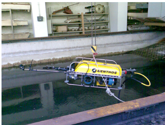
Fig. 4. StingRay ROV with installed Micron scanning sonar
