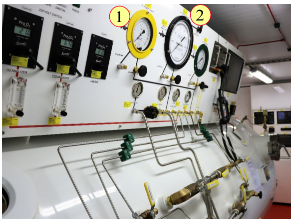
Control panel designed by Smart Dives with bourdon tubes depth gauges of 120 mm (#1) completed by a unit of 200 mm (#2) connected to the main lock.
