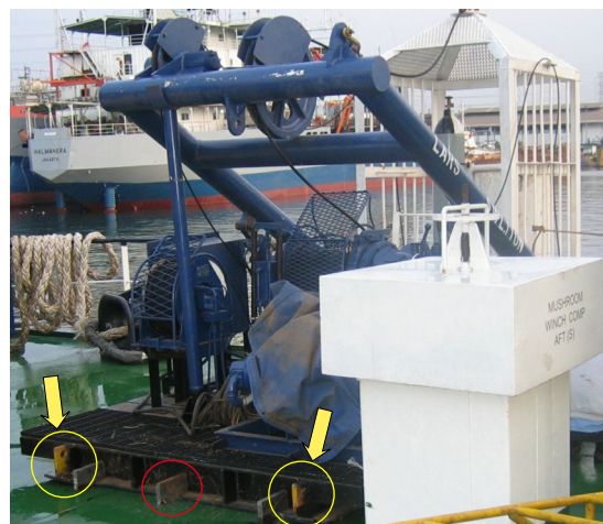
Fastening wedges and lifting points (in yellow)
