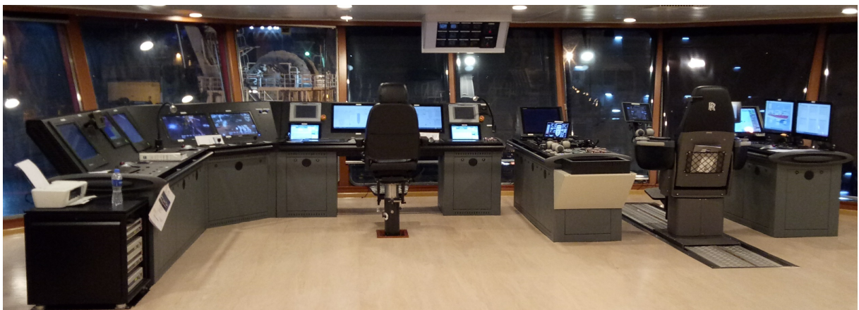
Dynamic positioning control station UDS Picasso
