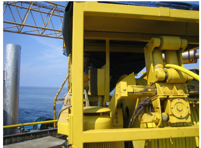
Umbilical winch installed below the jib of the crane. Note that the wire winch is on the jib.
