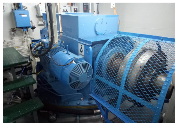
Topside parts of Azipull: portside.
