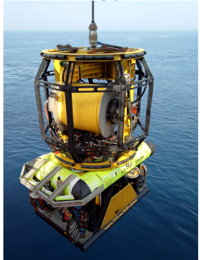
Top-hat type TMS: Note the fixation to the armoured lifting umbilical, and the mechanism of the system.
