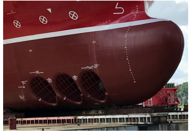
Tunnel thrusters of UDS Van Gogh
