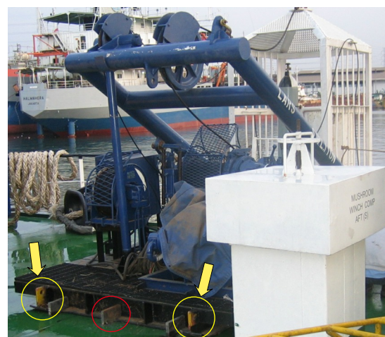
Fastening wedges and lifting points (in yellow)
