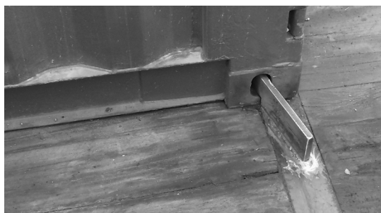
Welded wedge securing an ISO fitting
