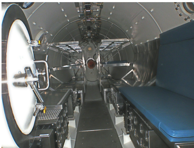
Chamber 24 divers designed by Flash tekk engineering: It provides 12 bunks and the equivalent number of seats
