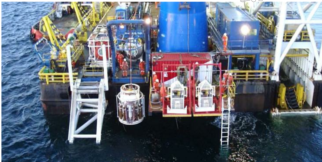
Launching platform at the stern of a lay barge
