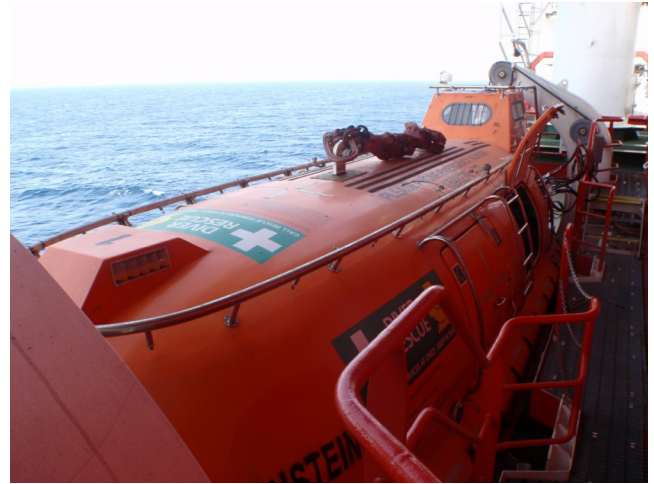
Self-Propelled Hyperbaric Lifeboat – SPHL
