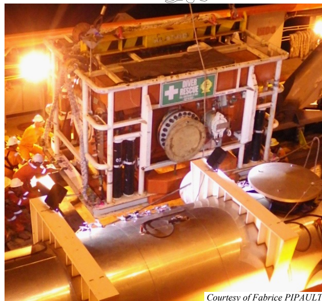
Exercise of transfer of the HRU. The descent is done with the crane instead of the A-frame at the stern of the vessel.
