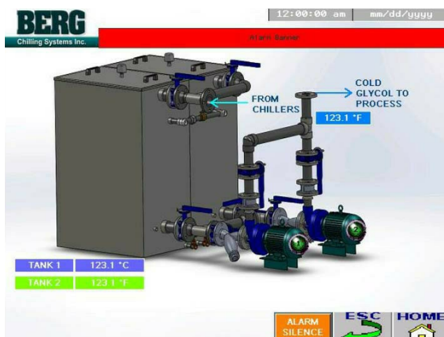
Temperature of the cold water/glycol mix in holding tanks
