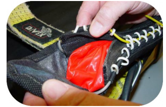
2 - Counterlung in its enclosure (see the photos above)
