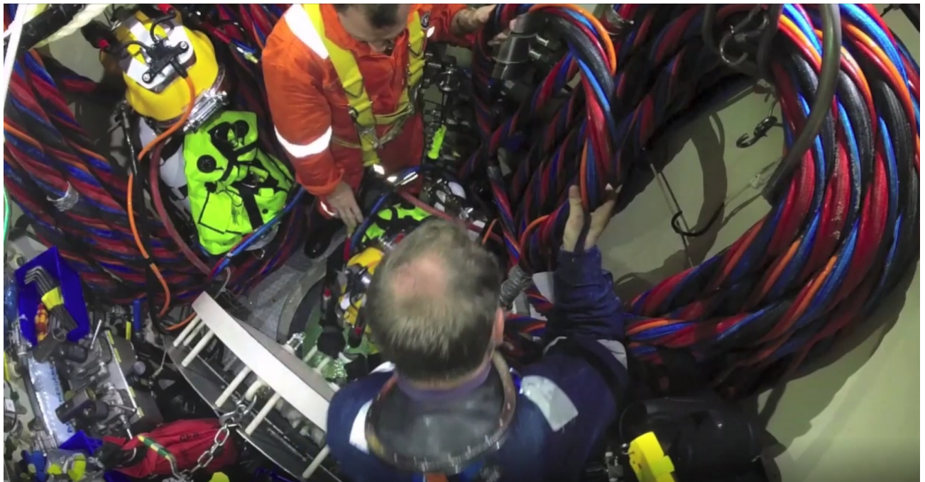
BCDs mounted on twin bottles sets used for shallow saturation diving in one of the bells of UDS Lichtenstein
