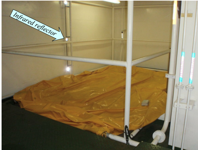
Gas bag cage. Note the infrared reflectors along the wall
