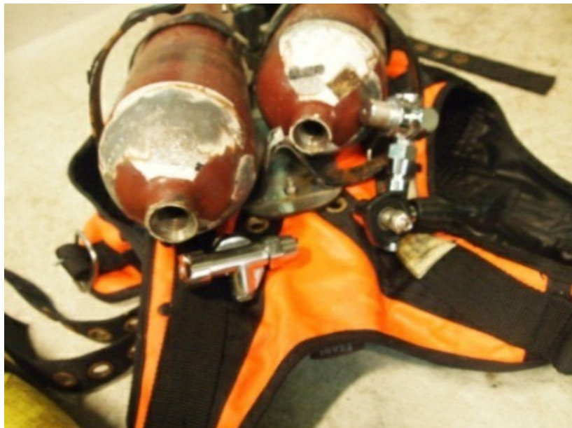
Broken manifold assembly
