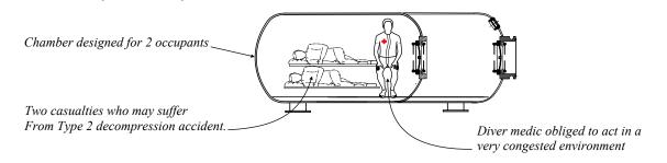
Another extreme scenario is that the divers in decompression cannot perform their stop in the water when the chamber is already occupied by two casualties and the diver medic. In this case, they will have to be transferred into the entry lock and perform their decompression in it. There is a low likelihood that this scenario happens, but it may happen due to this special rule that makes an undesirable event often happen with another one.
