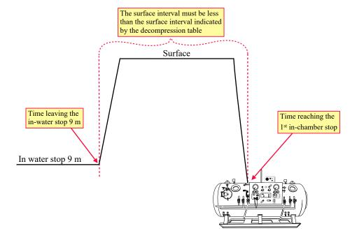
With this procedure, the diver is transferred to the surface without having completed his decompression. It is based on the fact that, generally, a decompression accident is not detectable immediately after surfacing and that a short period is necessary for the process to develop and symptoms becoming visible. Thus, the diver is transferred to the chamber and recompressed during this very short period. It is obvious that the diver must be transferred to the chamber as quickly as possible.
