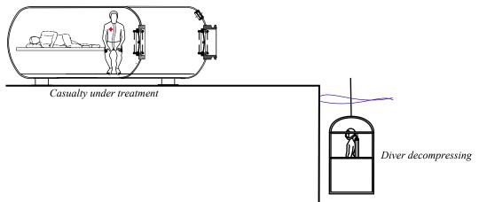
Note that in this case the diving operations are stopped until the treatment in the chamber is completed and the chamber returned ready for use.
