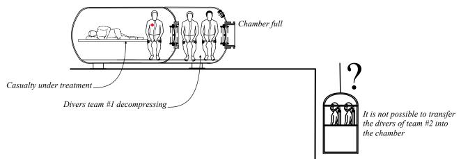
To be in the same condition as what is considered acceptable for "non continuous air diving" the divers at work on the bottom must not have any decompression stop to perform during the time the previous divers are performing their decompression. Thus, the divers at work can be immediately recovered to the deck.
