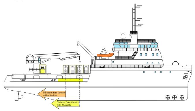
When the surface support is limited by its' size, which is often the case with the vessels used for inspection projects, the team preparing the vessel may be obliged to install additional platforms to secure the items. It is often the case with the boats of opportunity that are designed for another purpose than diving. These platforms must be checked and agreed by a classification society.
