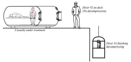
If due to unpredictable reasons the divers decompressing need to be transferred into the chamber, they can perform their stops in the entry lock as with the procedure agreed for "normal" air diving procedure. Because the divers at work have no decompression they can be recovered immediately on deck. It is a condition similar to the one commonly agreed for "normal" in-water decompression diving operations.
