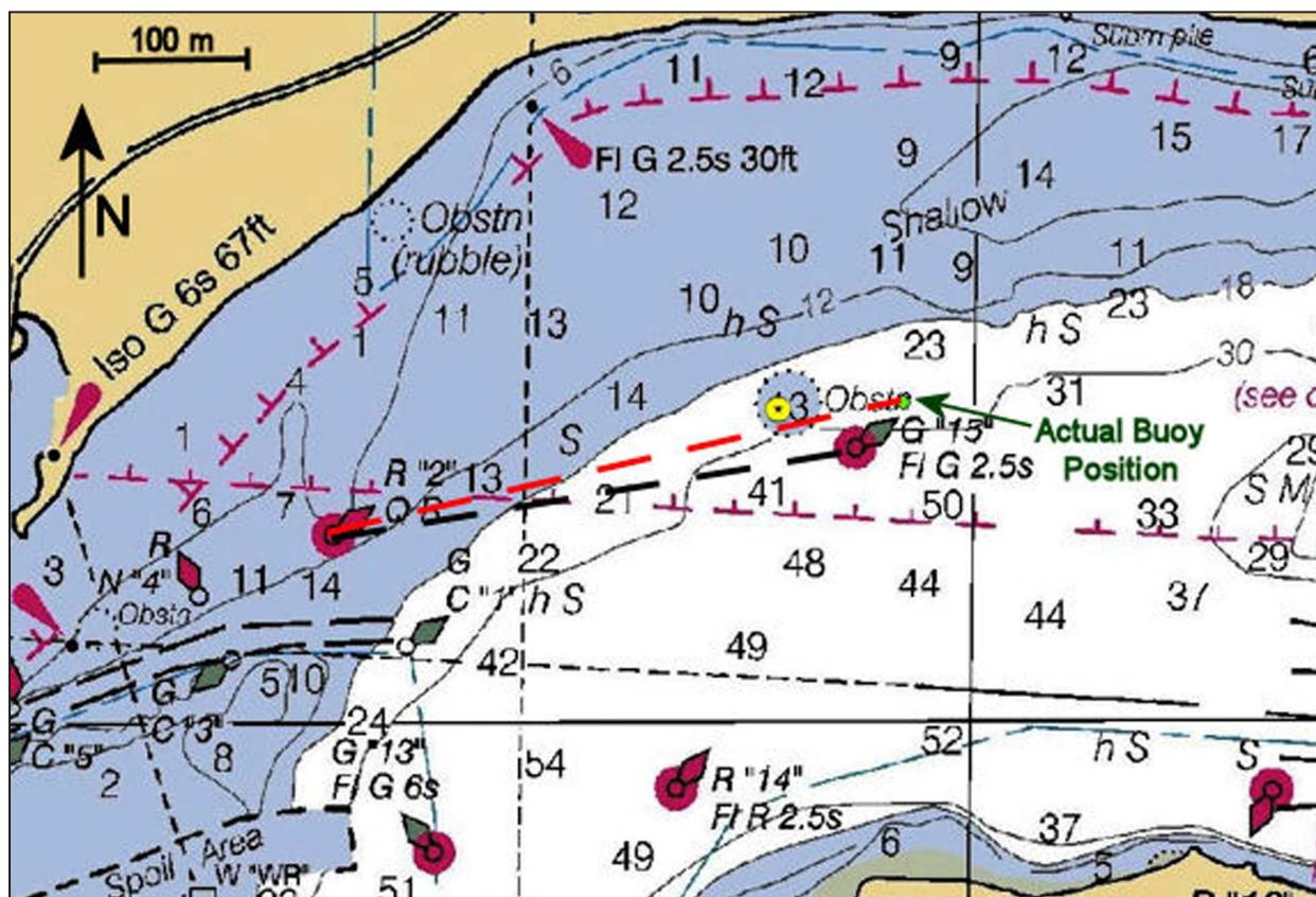
FIGURE 42. Migration of the north channel boundary, soundings in feet. (Figure by author, 2013. Modified from NOAA 2011.)
