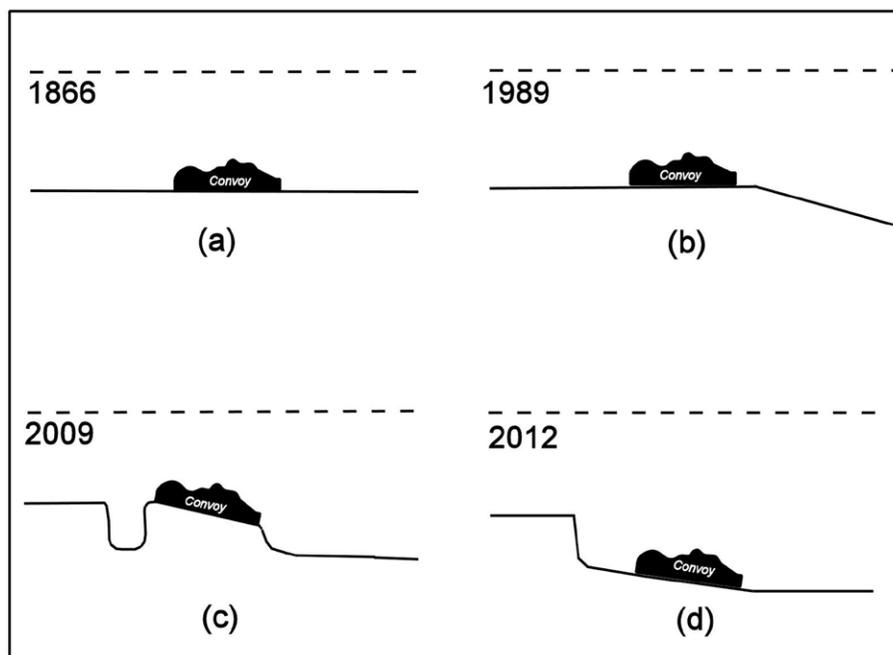
FIGURE 39. Scour and settle process for *Convoy's* wreck site. (Figure by author, 2013. Modified from McNinch et al 2006:294.)
