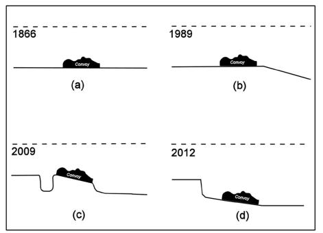
FIGURE 39. Scour and settle process for *Convoy*'s wreck site. (Figure by author, 2013. Modified from McNinch et al 2006:294.)
