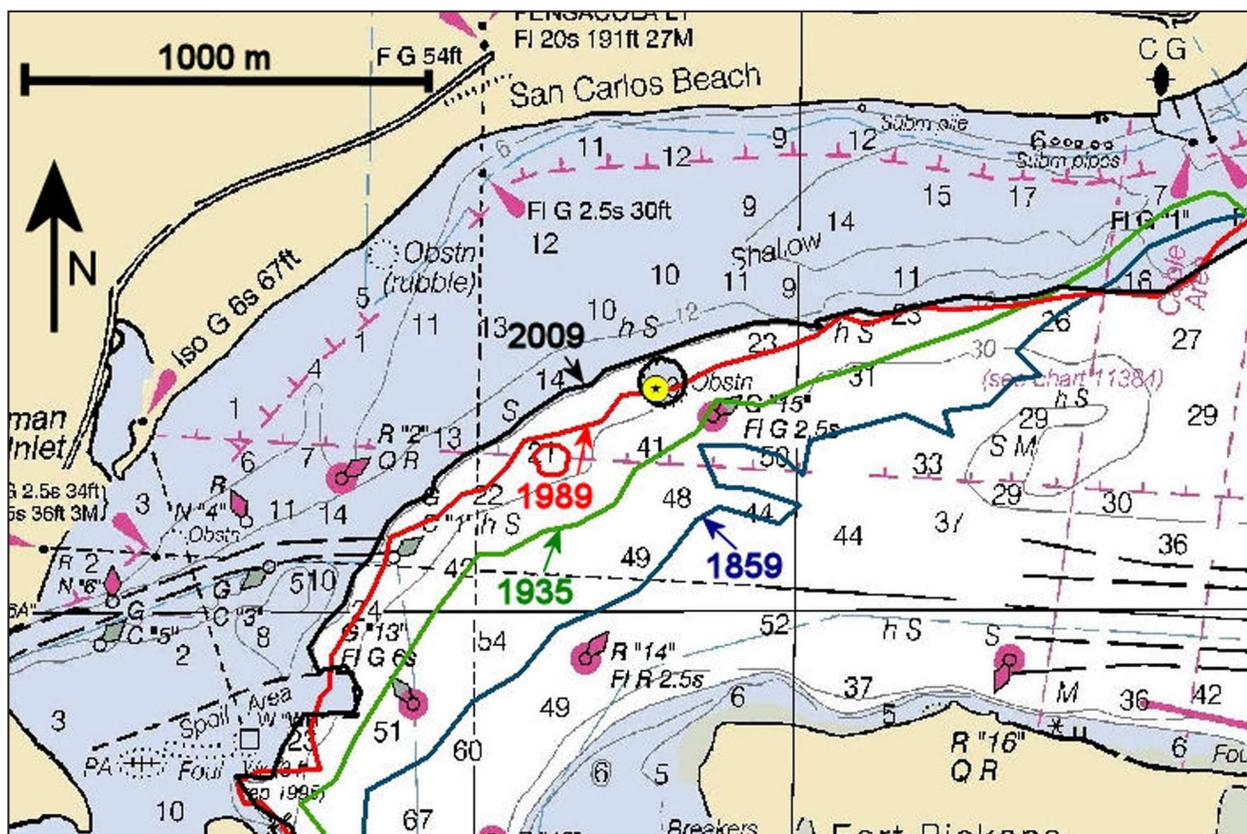
FIGURE 37. Channel scarp migration 1859-2009, soundings in feet. (Figure by author, 2013. Modified from NOAA 2011.)
