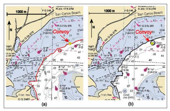
FIGURE 38. NOAA charts showing channel scarp regression, soundings in feet. (Figure by author, 2013. Modified from NOAA 2006 and NOAA 2011.)
