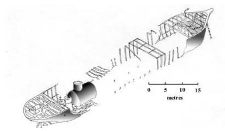
Figure 34. Isometric site plan of the P.S. *Blackbird* site (Goff Hewitt 1997)
