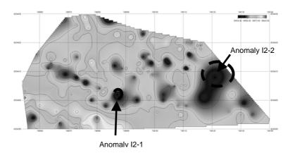
Figure 25. Independence Point magnetometer survey two showing anomalies (Ian Moffat 2006)
