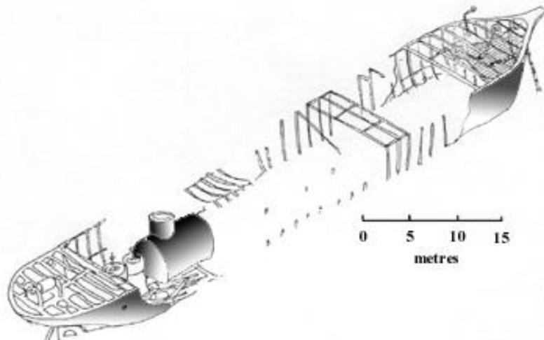
**Figure 34.** Isometric site plan of the P.S. *Blackbird* site (Goff Hewitt 1997)
