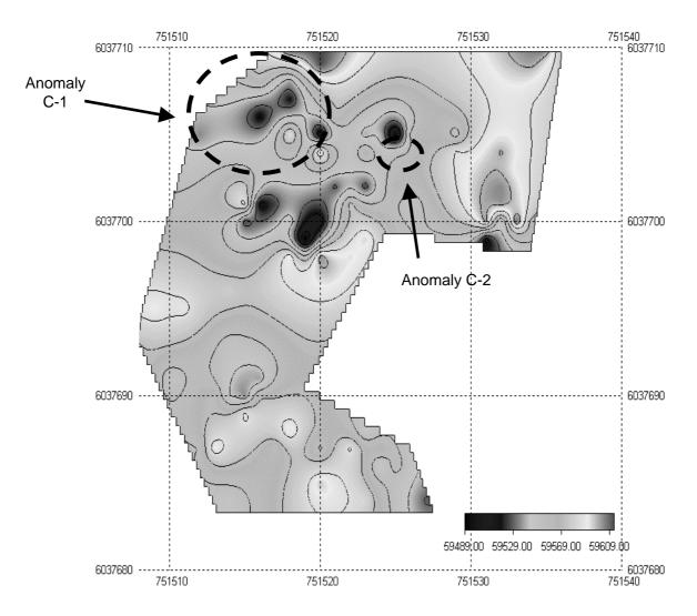
Figure 30. Fish Cannery Track Site magnetometer survey one showing anomalies (Ian Moffat 2006)
