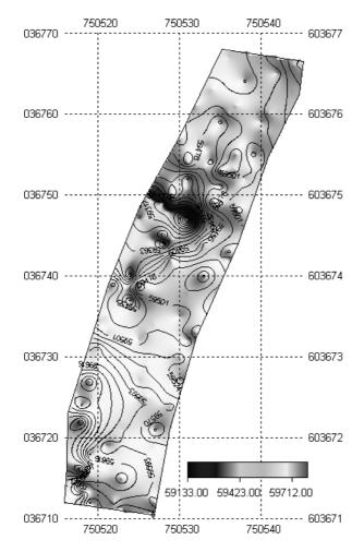
Figure 27. American River Township magnetometer survey two showing anomalies (Ian Moffat 2006)
