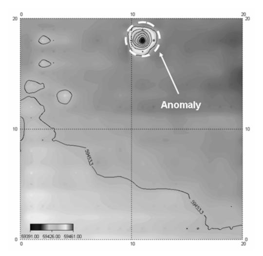
Figure 61. Horseshoe Bay detailed magnetometer investigation map with anomaly highlighted (Ian Moffat 2006)
