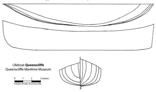
Figure 52. Field draft of *Queenscliffe* lines (Bullers 2006)
