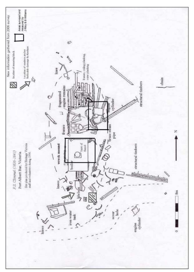
**Figure 35.** *P.S. Clonmel* site plan showing locations of hazard buoy pad and damage from modern anchor and chain (Maritime Heritage Unit 1996)
