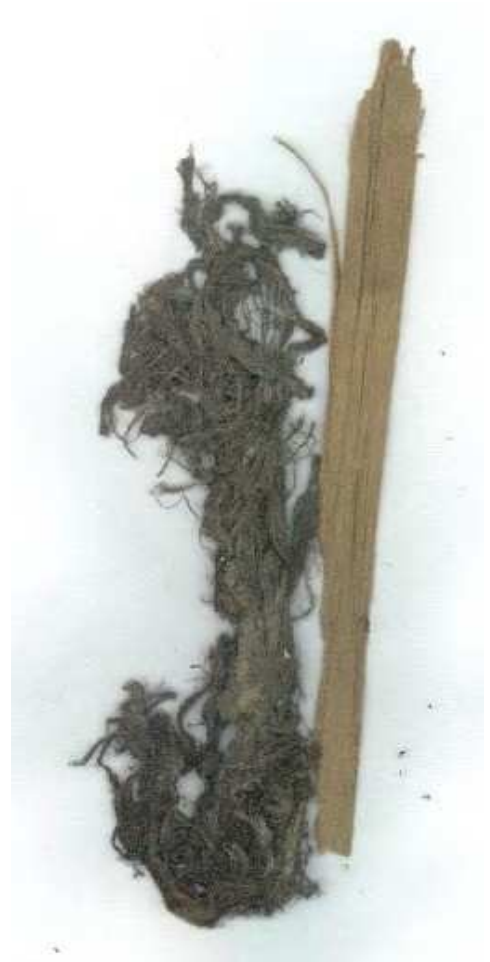
Figure 27: Sample of caulking material taken from LHL-81 in March 1980. The sample was never tested but is assumed to be hemp (Image from Nationalmuseet, Skibshistorisk Laboratorium, 1980).
