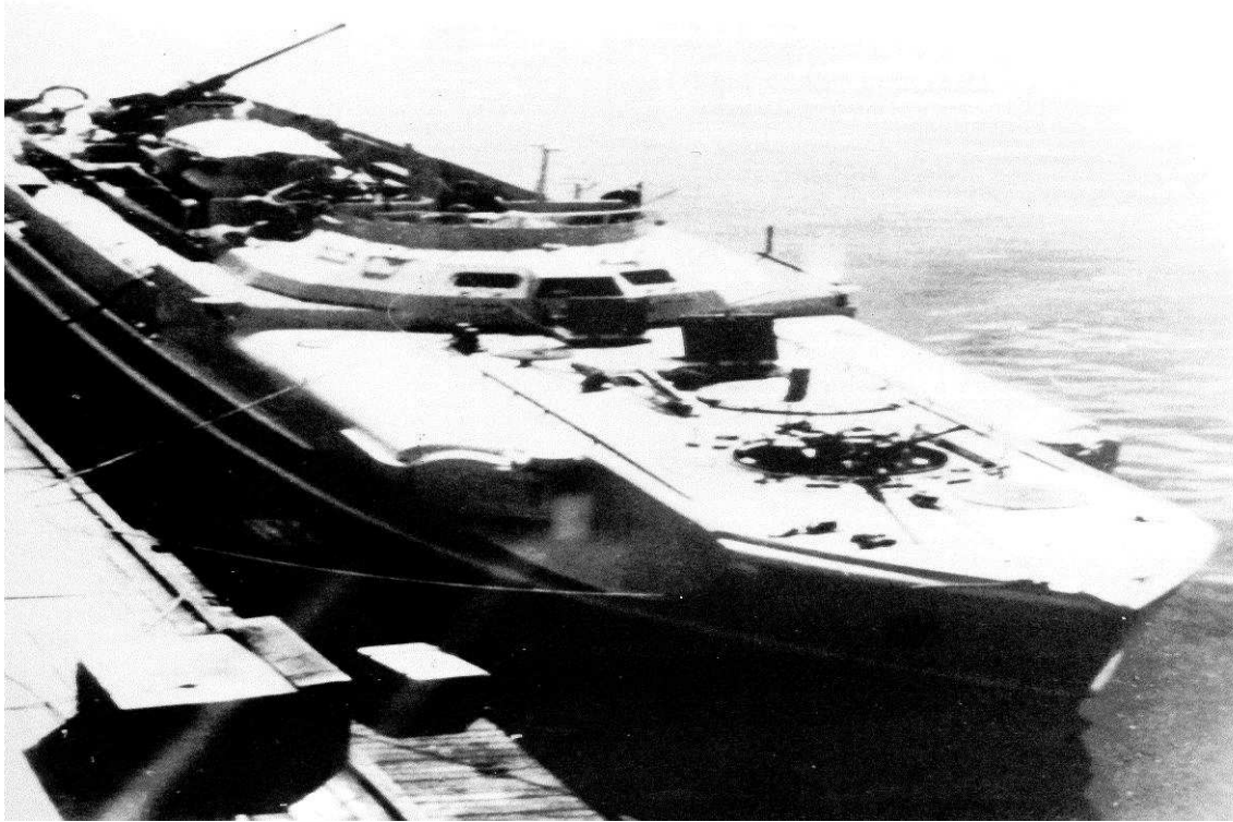
Figure 19 Kalottenbrücke ("Skullcap"), was introduced and armour progressively fitted (Source: (Whitley, 1992) pg.29).
