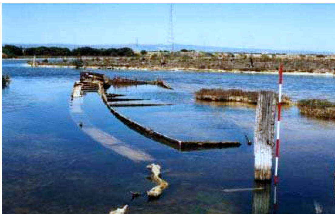
Figure 9.20 Remains of Jupiter , Mutton Cove Ships' Graveyard (Port Adelaide, South Australia) showing pile driven through the bow of the vessel (Photo: Nathan Richards, 12/02/2001)
