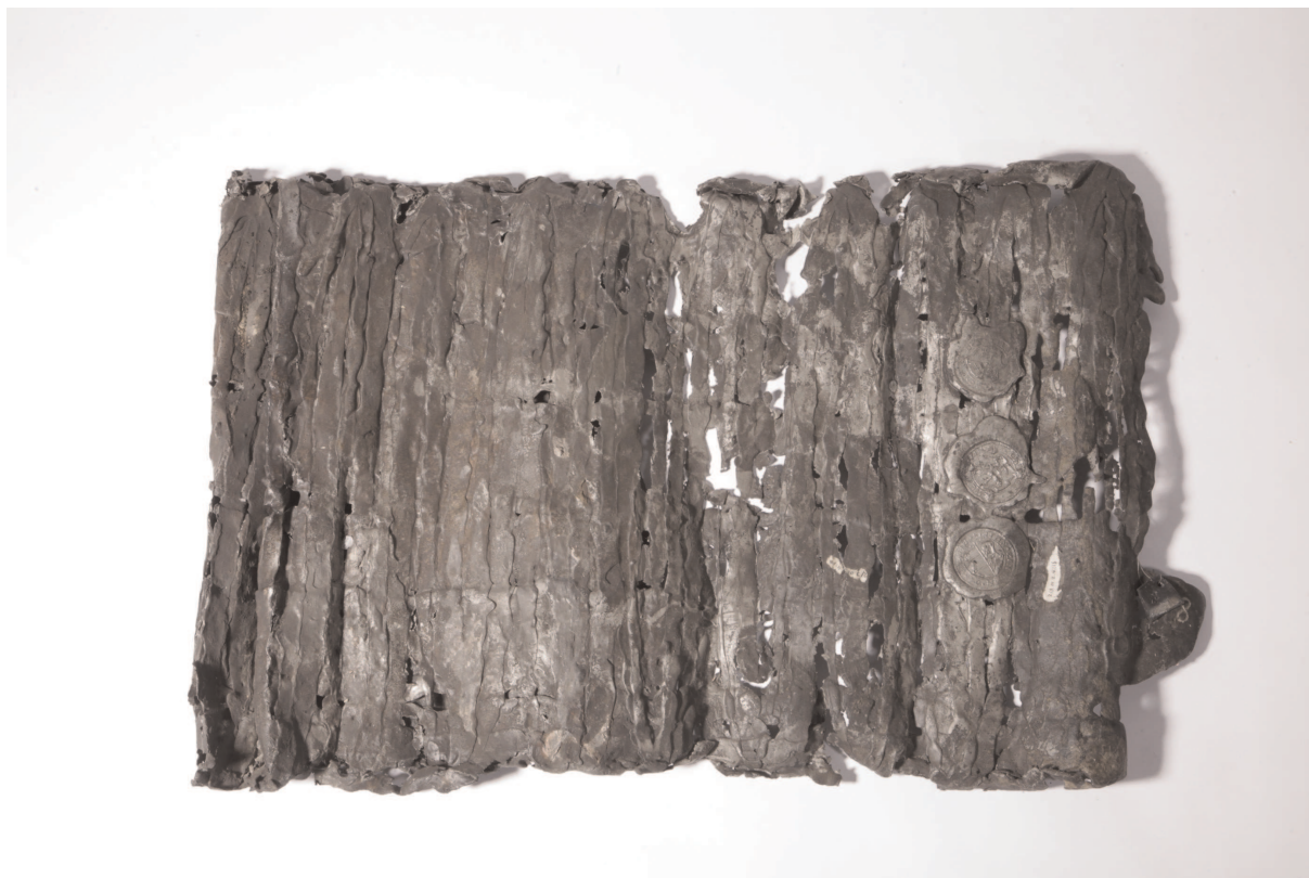
Figure 26 An unrolled sheet (AM-2/3.01.2.4.16) clearly shows that fluid tin was poured on a (copper) plate in the way Agricola describes. The sheet measures 40 x 70 cm (photo: T. Penders (RCE)).
