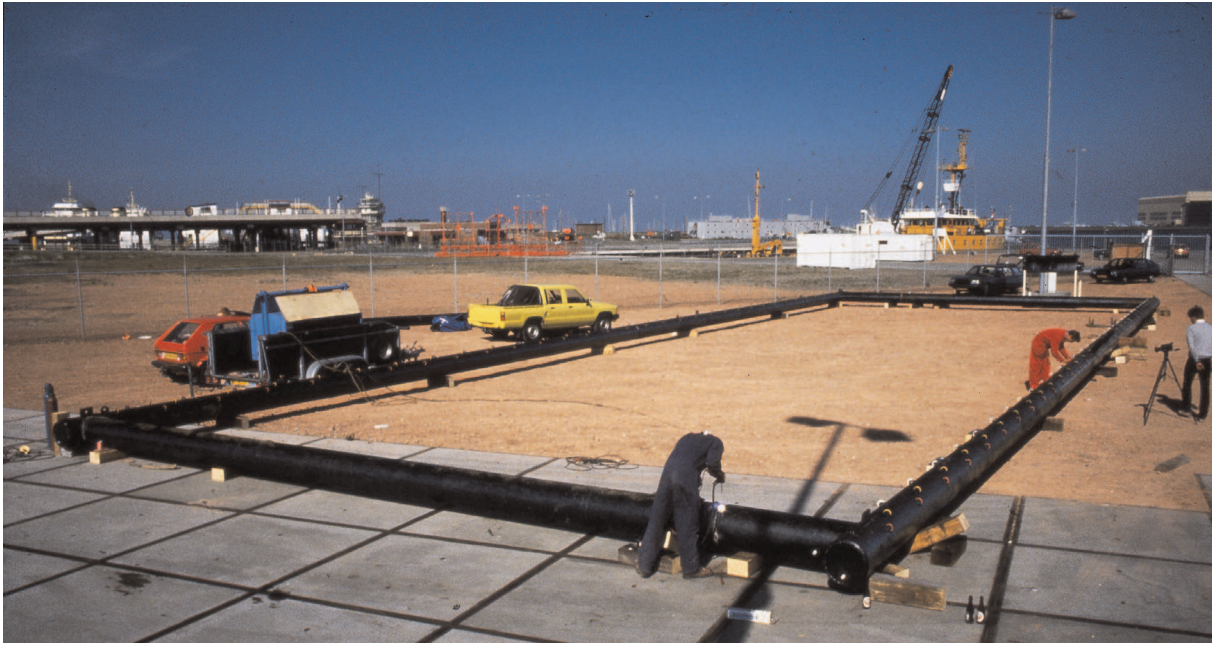
Figure 6 The steel frame at the quay in Den Helder, prior to being sailed out and lowered around the wreck-mound. Note the staggering, colour-coded eyelets at 25 cm intervals along the side of the rectangle. These are meant for attachment and navigation of the floating crossbar that holds the camera. They also served as help in drawing the site plan, in which they are indicated with numbers. The four-legged safety booth that was to be attached to the frame can be discerned in the background (photo: A. Vos (RCE)).
