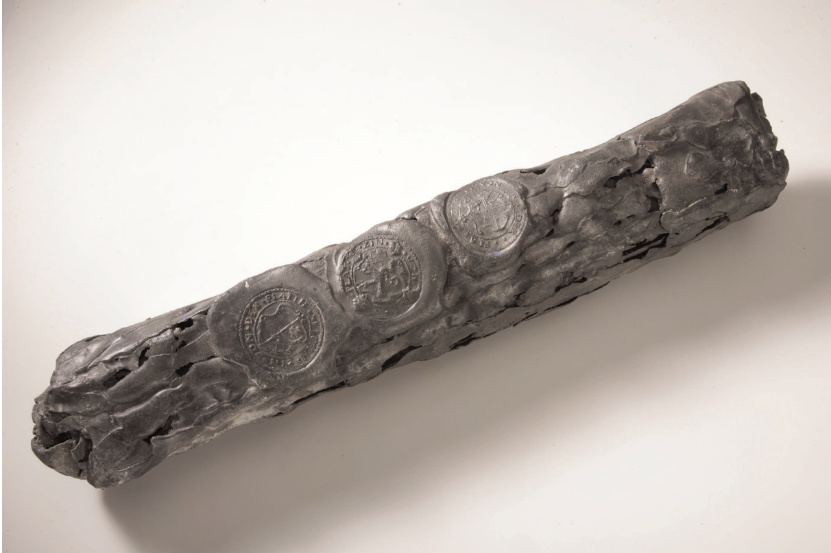
Figure 22 A typical roll of tin (AM-7.8.3) with marks from Horní Blatná, length 42 cm, weight 4210 g (photo: T. Penders (RCE)).
