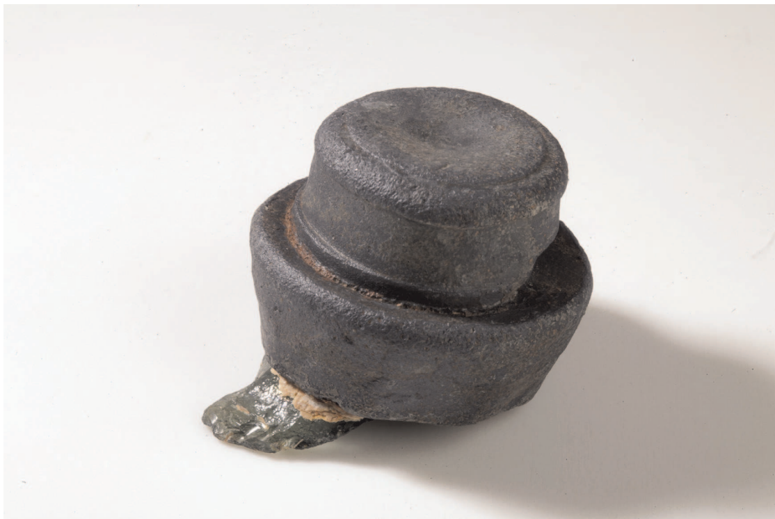
Figure 37 Screw cap with a sherd of glass. Although similar caps are generally referred to as pewter, these caps are 90 to 97% lead. Diameter cap is 3 cm (photo: T. Penders (RCE)).
