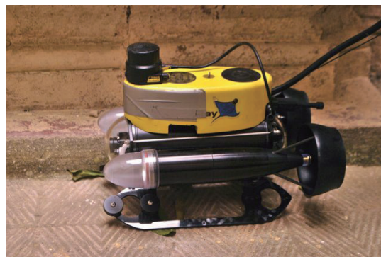
Fig. 1: The VideoRay Pro 3 GTO is an underwater micro-ROV with dimensions 36.8cm x 28.9cm x 21.6cm. It is equipped with depth and compass sensors along with a front and a rear video camera. Additionally, a Tritech Micron scanning sonar can be attached to the ROV.
