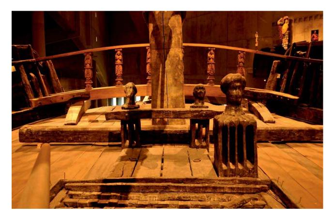
Figure 6.1. The halliard knighthead and topsail sheet bitts at the foremast, as seen from aft. (Photo: the author).
