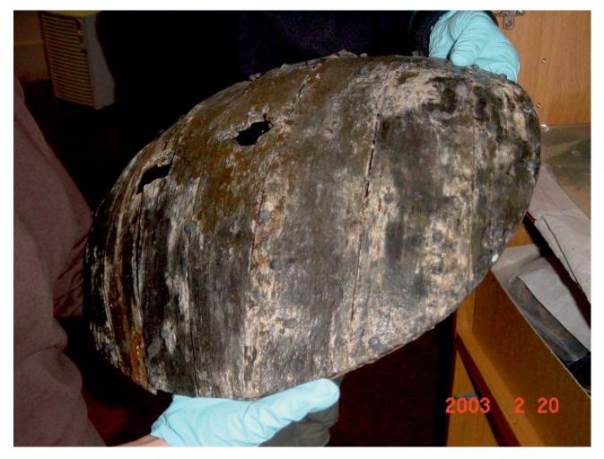
Figure 4.3b. Precipitated acidic sulphate salts on a gun shield from the Mary Rose (1545). (Photo courtesy of Magnus Sandström)
