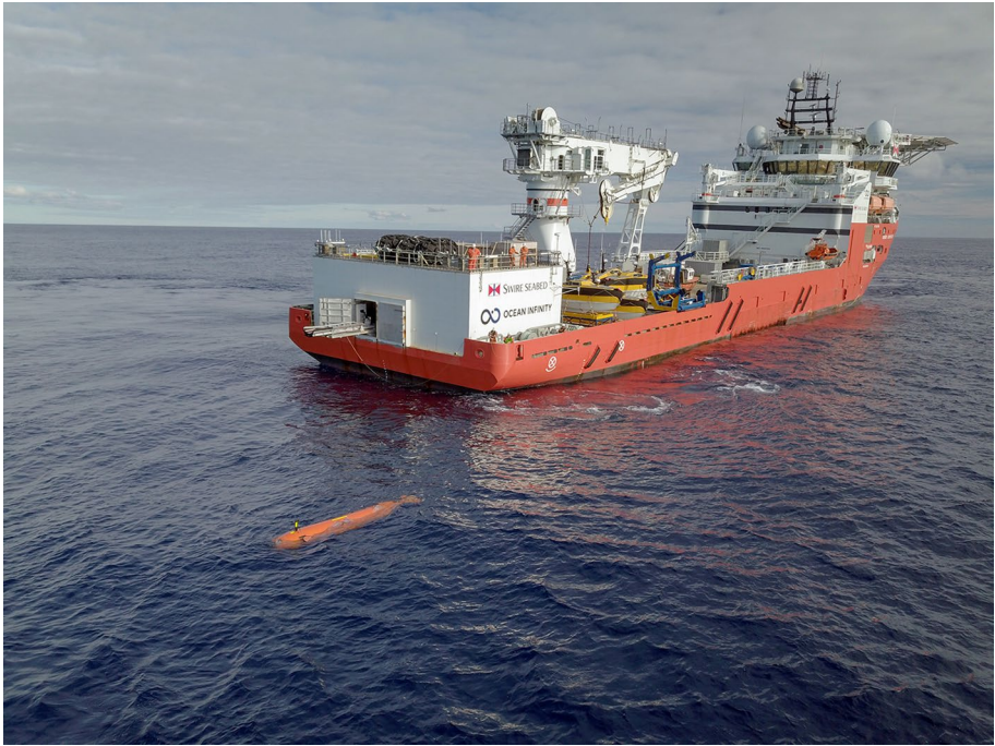
Fig. 3 Launch of HUGIN AUV from Pacific Constructor (Ocean Infinity)
