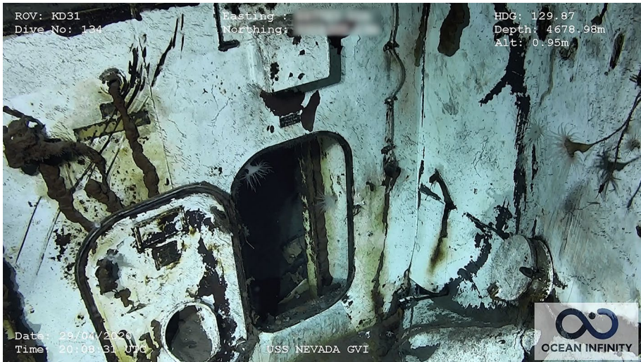
Fig. 17. 5-inch shell handling room and mount for a dual 5-inch/38 gun (Ocean Infinity/SEARCH)
