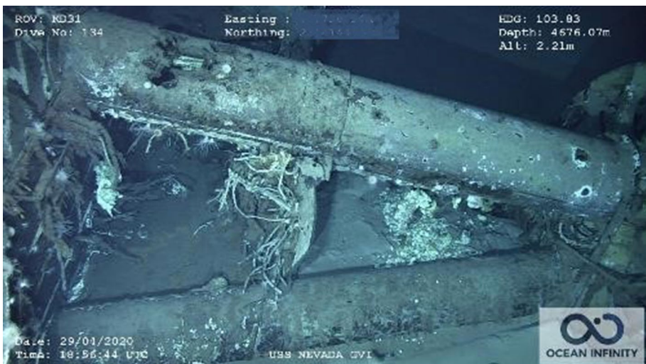
Fig. 19 Shell fire damage to the tripod foremast (Ocean Infinity/SEARCH)
