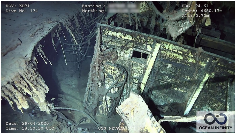
Fig. 20 View aft toward the aft compartment with a watertight bulkhead and hatch, shut for Condition X-Ray (Ocean Infinity/SEARCH)
