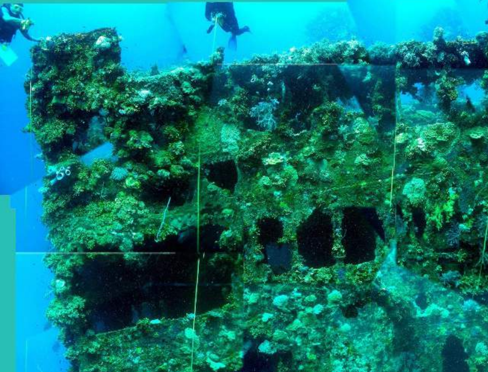
Figure 5-5. Photo-mosaic of the bridge face of Fujikawa Maru showing the impact of dynamite fishing. This area should be totally covered with corals and sponges but many have been killed by dynamite fishing which also greatly weakens the iron structure and renews corrosion. In 2012, Dianne Strong, a frequent visitor to Chuuk reported that the bridge collapsed in the middle. ©Bill Jeffery 2006
