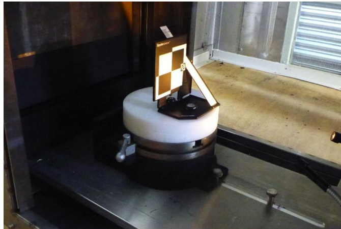
Figure 3. Rotary table in its usual position. On the sample mounting spacers are the Spyder calibration tools used to calibrate the camera. The bolt in the baseplate indicates the position of the rotary stage when small items are examined.
