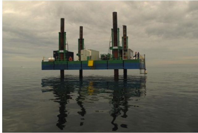
Figure 5. Jack-up Platform Barge 1—the AHSP's diving platform. Photo by A. Viduka.
