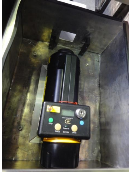
Figure 2. The X-ray source in the source box with the 3D camera removed. The beam-defining aperture can be seen.
