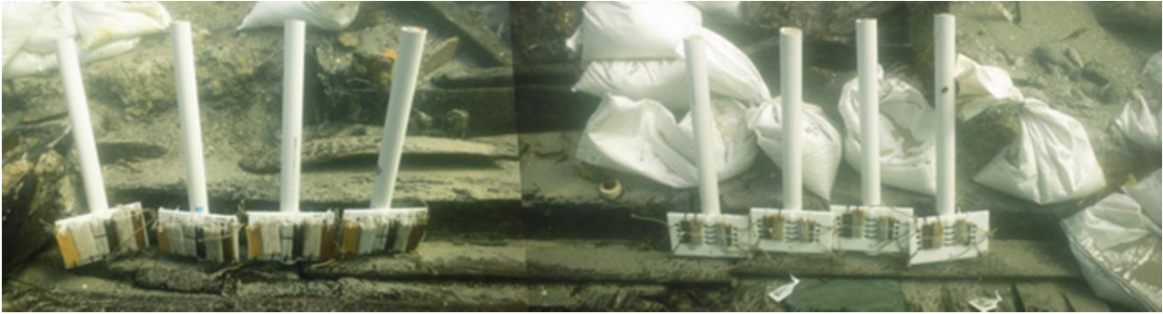
Figure 34. Sacrificial iron and wood samples and wrapped metal artefacts on site prior to reburial. Image by K. Kasi after J. Parkinson.
