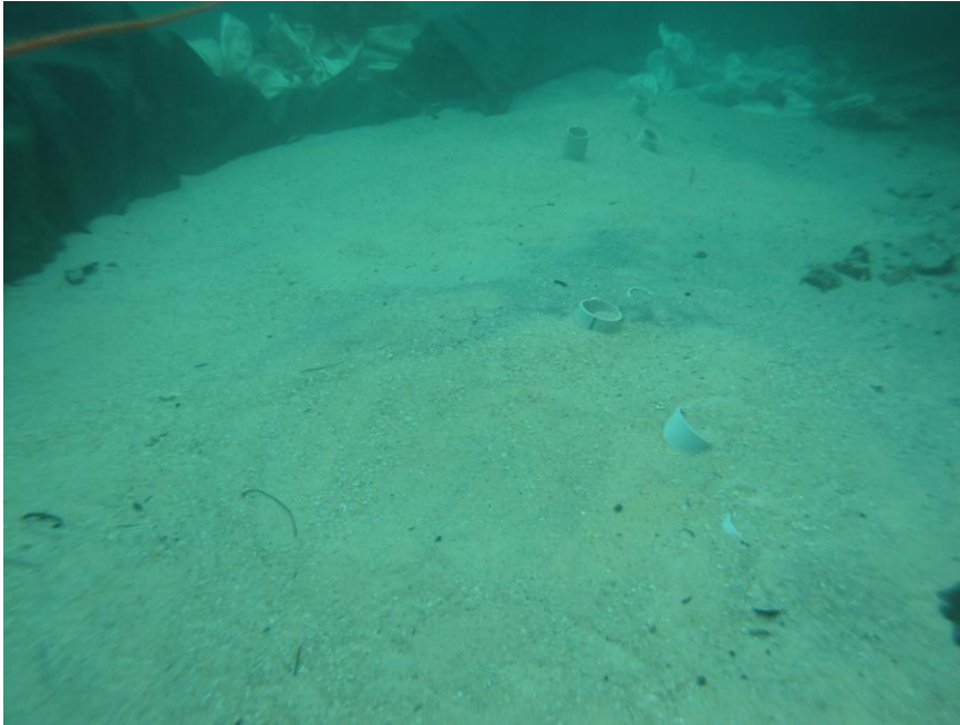
Figure 35. Sacrificial samples covered with 1 m of sand. Photo by AHSP.
