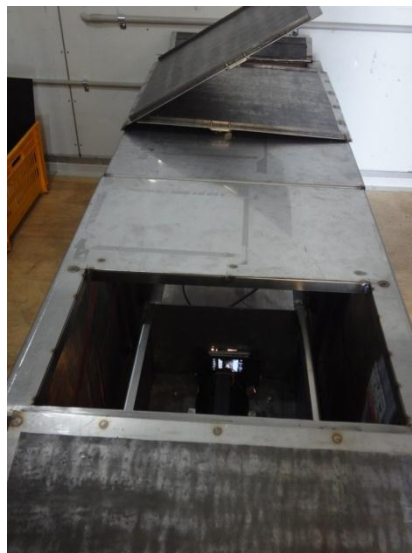
Figure 1. X-ray enclosure showing the access doors for the X-ray source, the specimen stage, and the imaging plates. The X-ray source has been removed, and the camera inserted. The photographic image, presented on the viewing screen of the camera can be seen.
