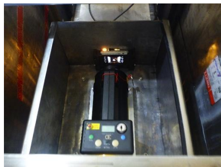
Figure 4. X-ray source and camera in position. Note the camera is removed when X-ray images are to be acquired.
