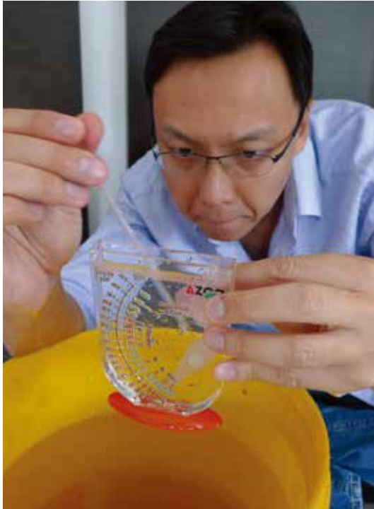
Marco Li monitoring the amount of salt in the ceramic washing water.
