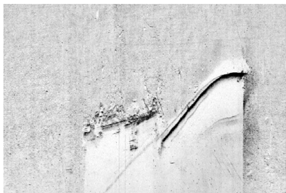
Figure 40. Sidescan of the wreck of RFA Darkdale –the ship is broken in two with the bow section at right inverted and the after end at left lying on its port side. Such surveys are routinely undertaken during environmental assessments of wrecks. © Crown copyright 2014
