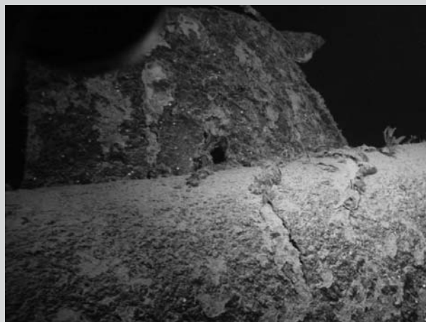
Figure 1. A shell hole at the starboard base of the conning tower on the Japanese midget submarine. Photo courtesy of the National Oceanic and Atmospheric Administration/Hawaiian Undersea Research Laboratory.
