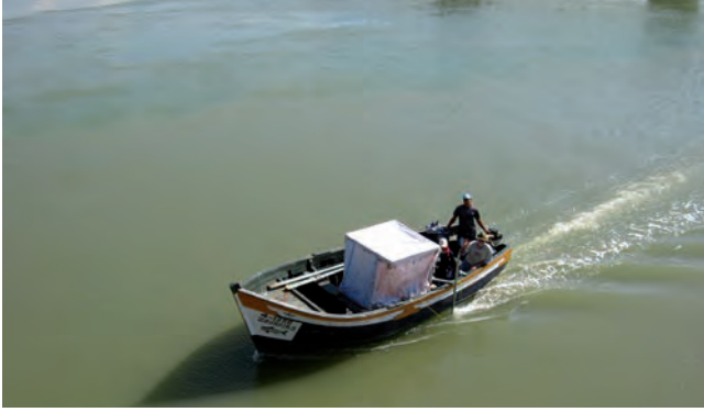
◀ © MMRG. A Knudsen 320 BP Echo-sounder in use over the port side of Zouhair 3 , a small fishing boat, in the Oued Loukkos during the Morocco Maritime Survey investigation into the location of the ancient port of Lixus, Morocco.
