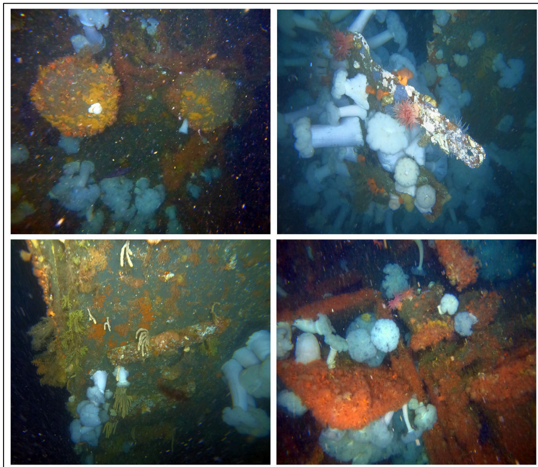
Figure 7. ROV imagery of Kotohira Maru . ( Top Left ): Deck bollards; ( Top Right ): Broken deck plating with significant anemone growth; ( Bottom Left ): Hull plating with cargo batten; ( Bottom Right ): Piping with increased corrosion and benthic growth.
