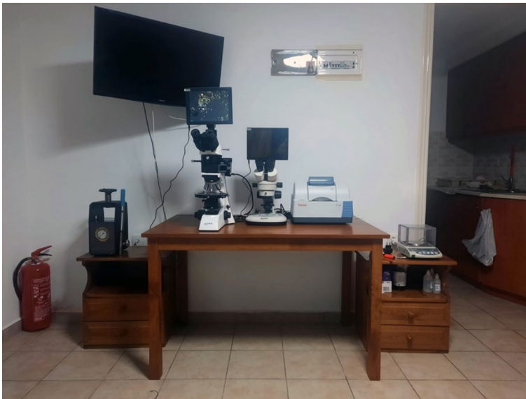
Fig. 4 Instrumentation of the on-site laboratory from left to right: petrographic microscope, binocular microscope, FTIR spectrometer and an analytical balance
