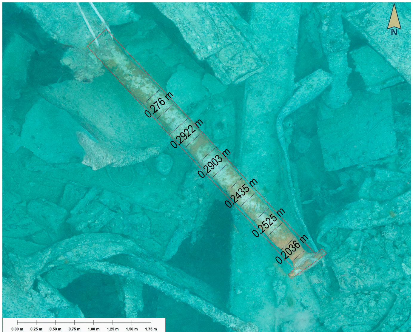
Figure 22. The steel propeller shaft as recorded in 2017 with the outline of the original as-designed shaft taken from the engineering drawing overlaid (red outline). A series of sectional measurements across the diameter of the shaft reveals lower values compared to the original manufactured shaft diameter of 1' \frac{1}{2}'' (317 mm), most likely caused by ongoing abrasion from mooring lines. Note also the evidence of red oxidation on the steel shaft (after Lloyds Register Foundation Archive Drawing No 10422).
