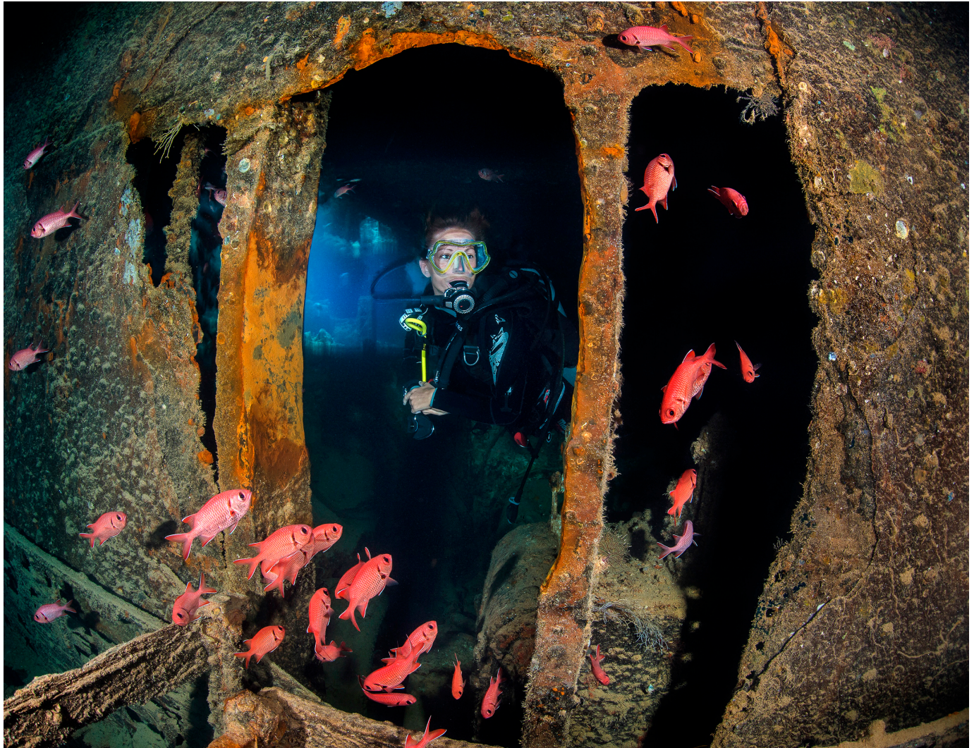
Figure 17. Access hole through the watertight bulkhead between Hold Nos. 1 and 2. The red oxidisation of the vertical ribs indicates ongoing abrasion by divers (Photo: Alex Mustard).
