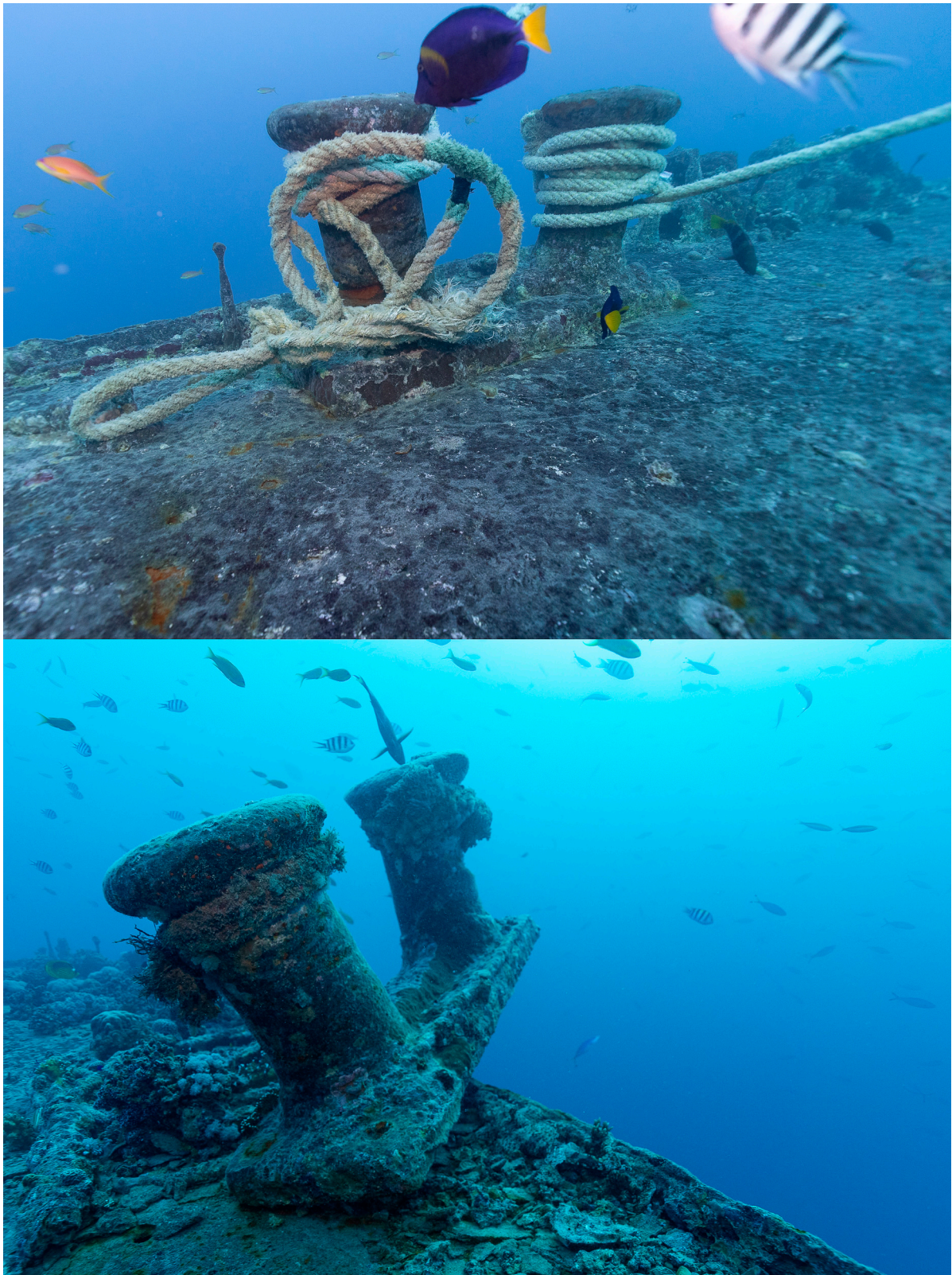
Figure 8. Top: Dive vessel mooring lines secured to a deck bollard on the bow in 2017. In absence of alternatives using the deck bollards remains a common approach but is not sustainable (photo: Alicia Johnson). Bottom: By 2023 this bollard has become displaced following failure of the welds securing it to the deck. Note the mooring line around the nearest bollard (photo: Alicia Johnson).
