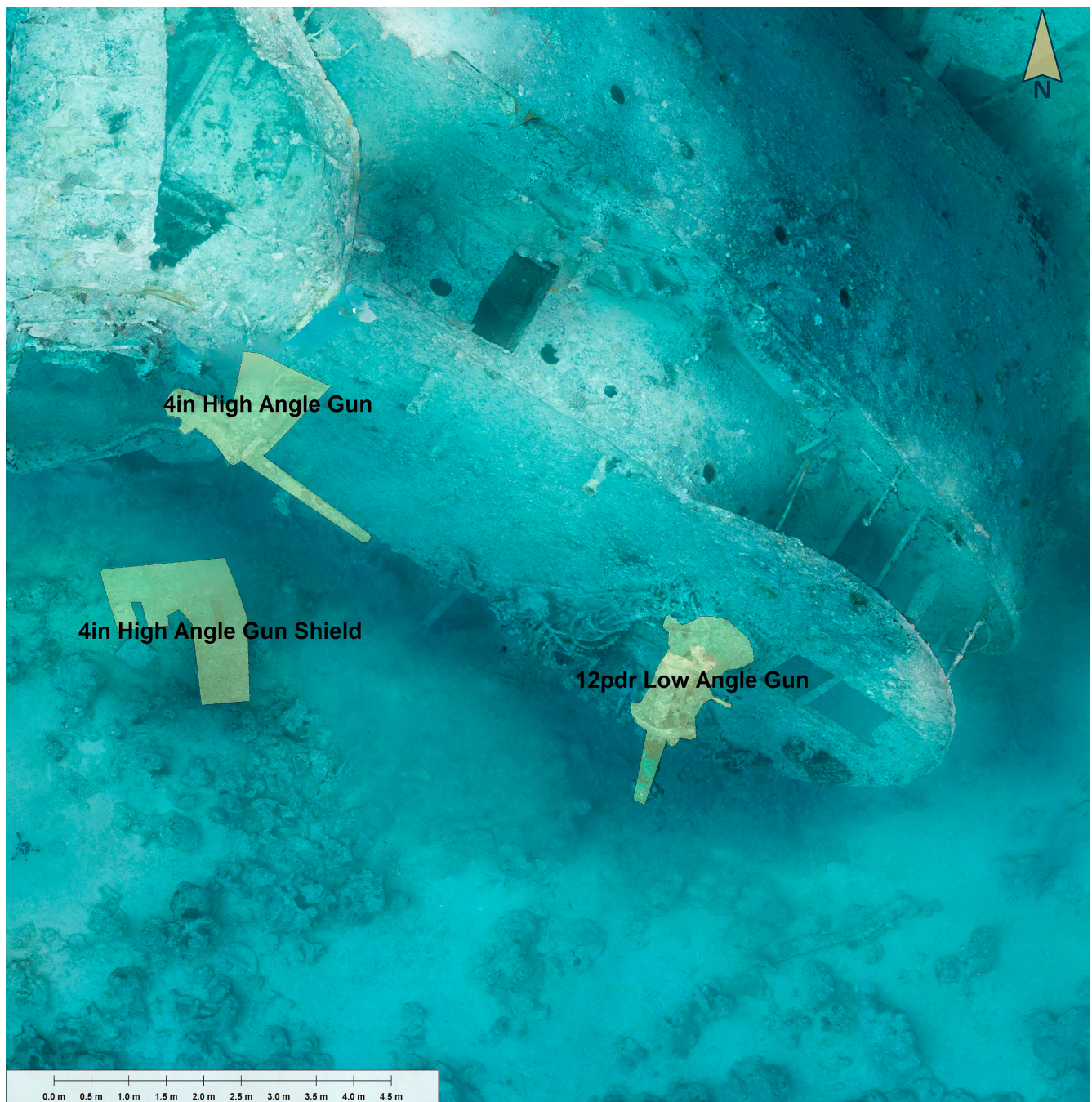
Figure 19. The 2017 survey records the stern high angle gun shield as detached and lying on the seabed directly under the gun.
