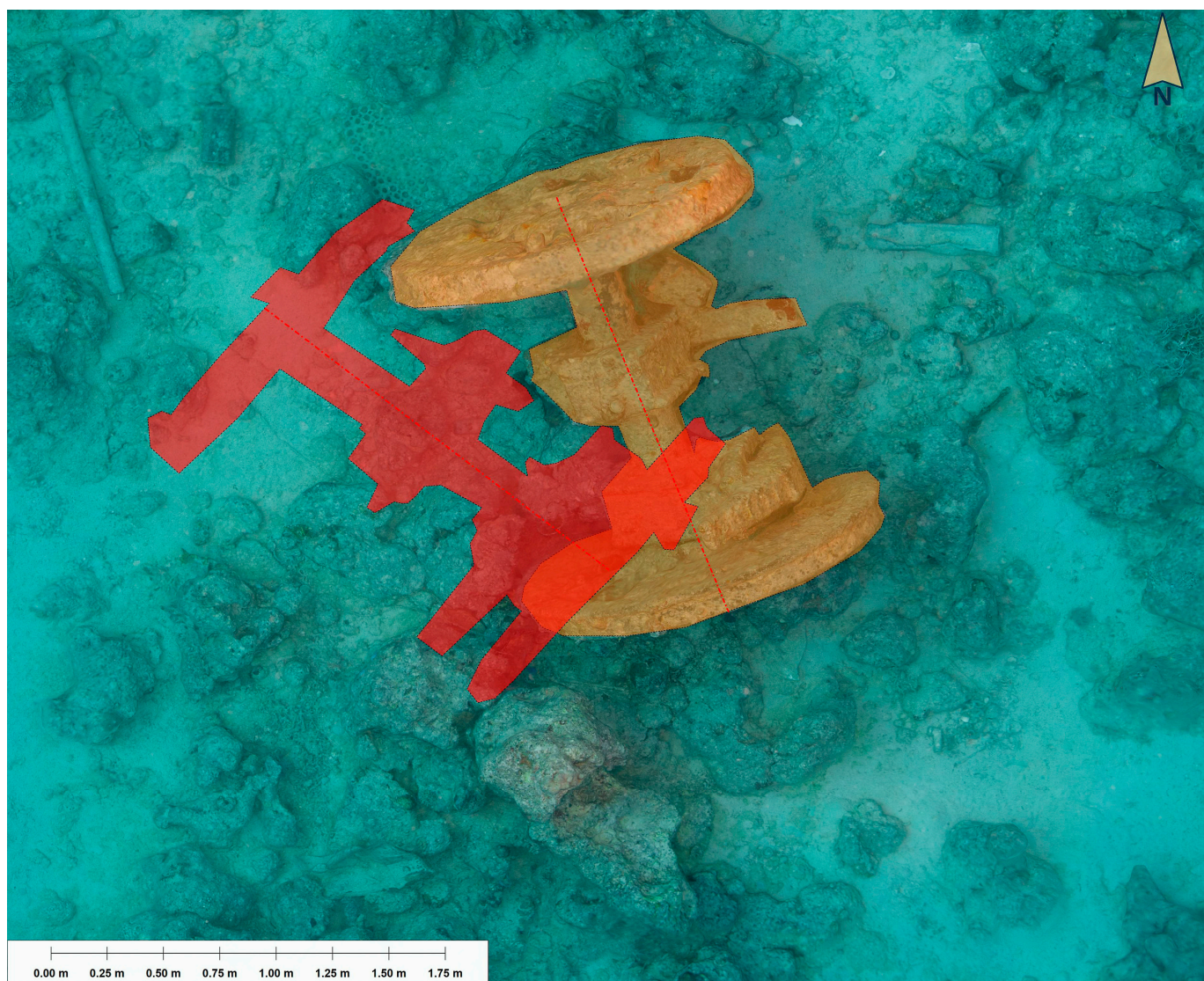
Figure 21. Starboard locomotive wheel assembly with recorded changes between 2017 (Orange) and 2022 (Red). At some point between July 2017 and May 2022 a substantial force was applied to the wheel assembly, rotating the wheels approx. 29^\circ counter-clockwise from their as-recorded position.
