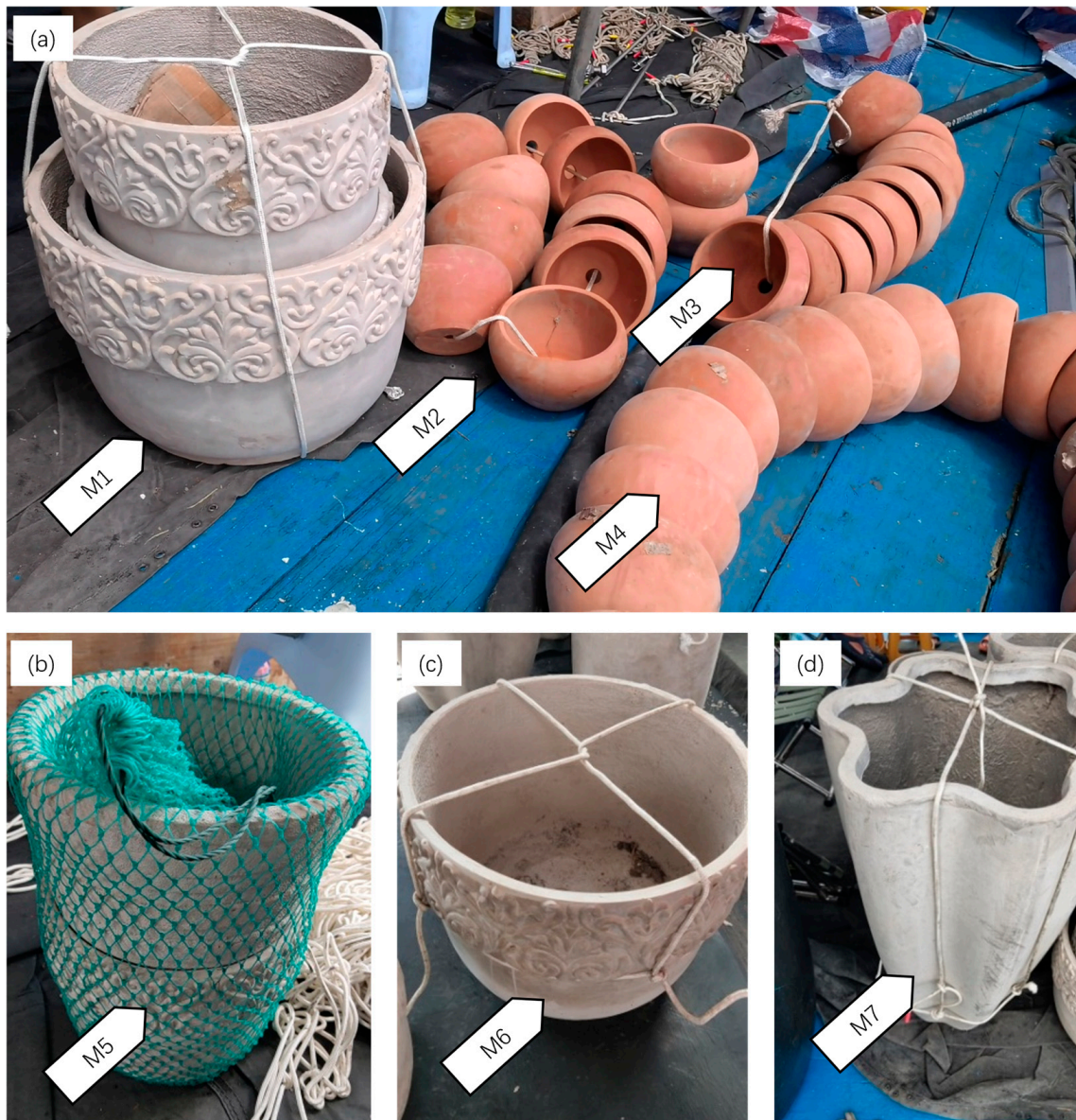
Figure 2. Physical diagram of the ceramic container. (a) Combination of medium models (M1) and small models (M2, M3, M4); (b) Combination of medium models (M5); (c) Single medium models (M6); (d) Single large models (M7).
