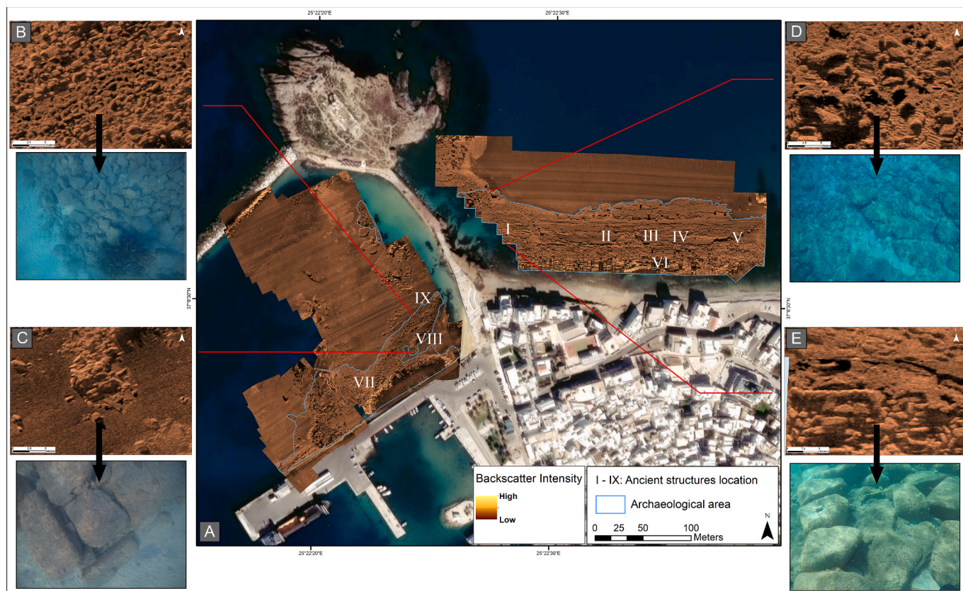
Fig. 5. (A) Side-scan sonar mosaic of the surveyed area, with the location of the submerged ancient structures (I-IX). (B-E) Selected close-up views of underwater targets, each paired with sonar imagery and corresponding underwater photographs. (B) Concentration of stones, part of the manmade structure IX. (C, E) Densely constructed masonry of Structure VIII and Structure I respectively. (D) Scattered, unprocessed stones, part of the natural seabed.
