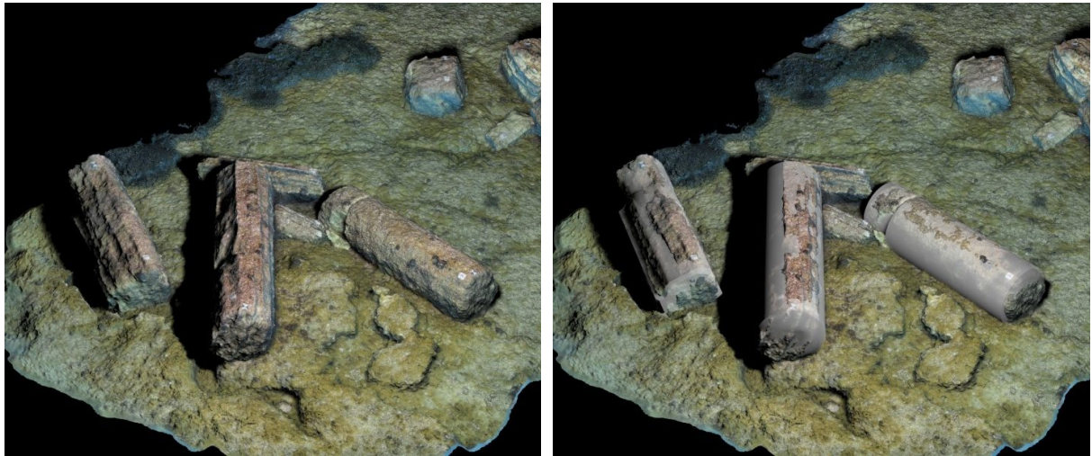
Figure 10. Marzamemi I shipwreck. Original mesh from Photoscan software (on the left) and the mesh integrated with polygonal model textured (on the right).
