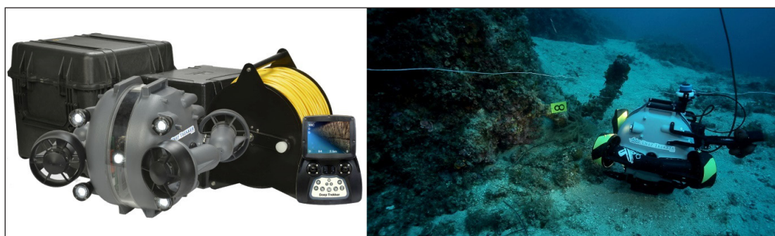
Figure 10 The DTX2 underwater drone surveying the Kamari anchorage site.
