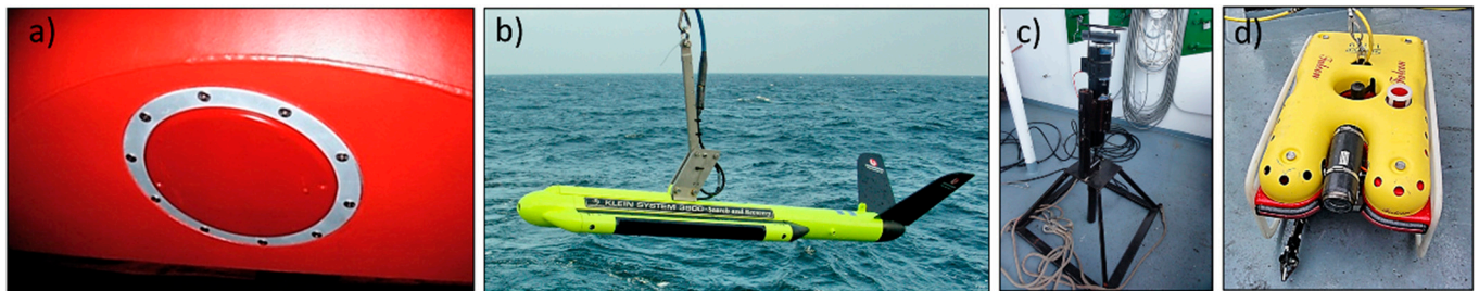
Figure 3. Instruments used for surveying the airplane wreck: (a) multibeam echo sounder EM-3002D; (b) side-scan sonar Klein 3900 System; (c) scanning sonar ver. 1071; (d) remotely operated vehicle Falcon SAAB SeaEye.
