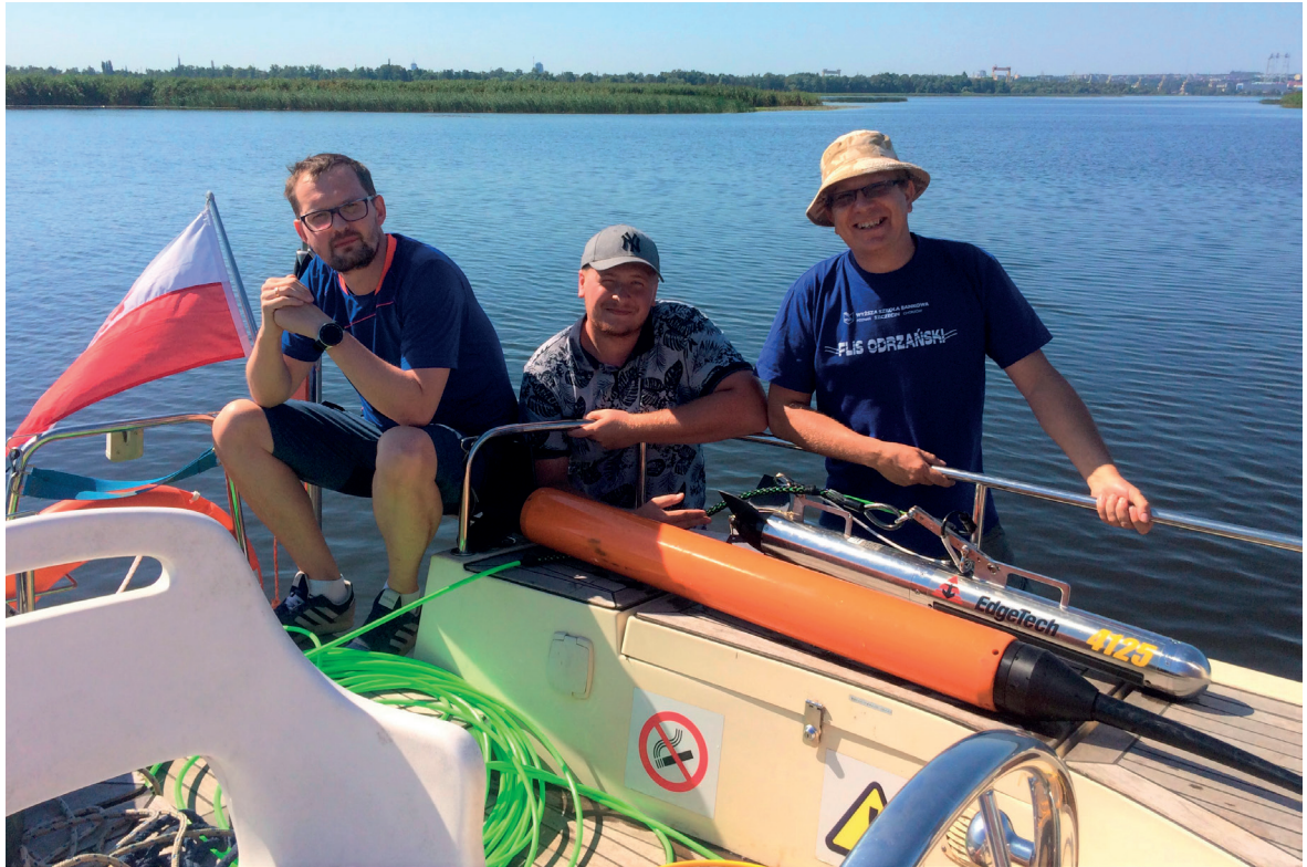
Figure 7.4. The researchers (from left: Grzegorz Zaniewicz, Adrian Popik, and Piotr Maliński) with research equipment – towfish transducers of marine magnetometer SeaSPY (in the foreground) and side-scan sonar Edgetech 4125 (photo: I. Bodus-Olkowska).
