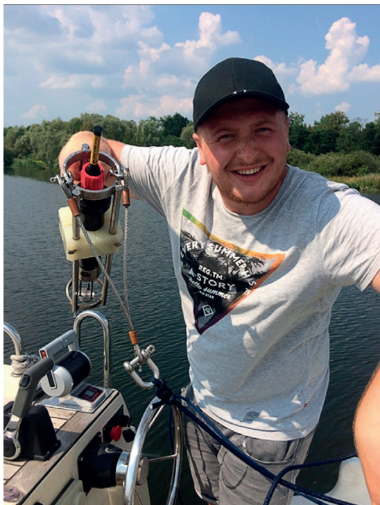
Figure 7.5. Adrian Popik presenting sound velocity sensor Valeport miniSVP just before taking measurements in the water of the East Oder (West Pomerania, Poland, photo: I. Bodus-Olkowska).
