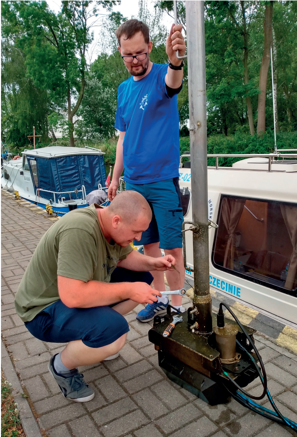
Figure 7.3. Adrian Popik and Grzegorz Zaniewicz checking the transducer of interferometric echo-sounder GeoSwath Plus (photo: P. Maliński).
