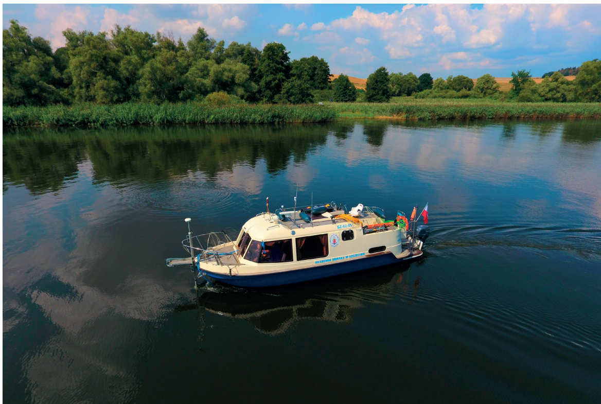
Figure 7.1. Research vessel Hydrograf XXI — Maritime University of Szczecin's 'floating laboratory' during side-scan sonar survey in the West Oder (West Pomerania, Poland, photo: P. Maliński).
